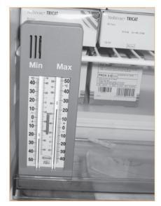
Fig. 3.8 Maximum/minimum thermometer.
