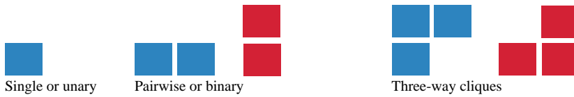
Figure 9.2. The possible cliques in a 4-neighborhood: single or unary cliques (left), pairwise or binary cliques (middle), and three-way cliques (right).
