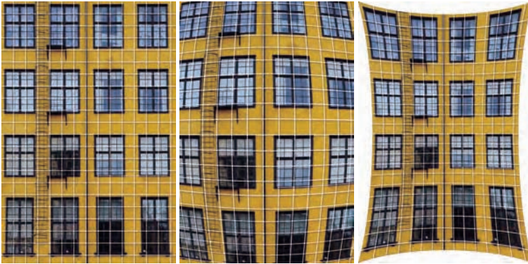
Figure 3.11. This figure demonstrates the effect of barrel (middle) and pincushion (right) distortions on an image (left). In this case, the distortions are exaggerated and overlaid with a grid for demonstration purposes.
