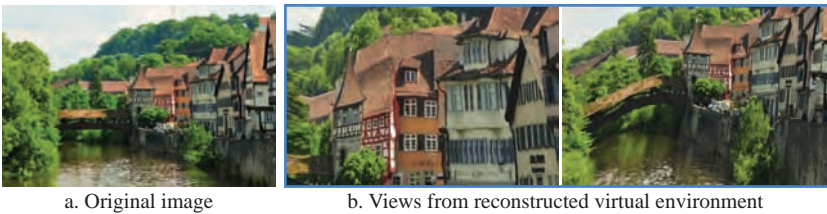
Figure 11.11. Using global and local features, Saxena et al. trained an MRF to reconstruct 3D geometry from a single image [652]. The image (a) can be mapped on the reconstructed geometry to form a virtual environment (b) that can be navigated interactively. (Schwäbisch Hall, Germany, 2012)
