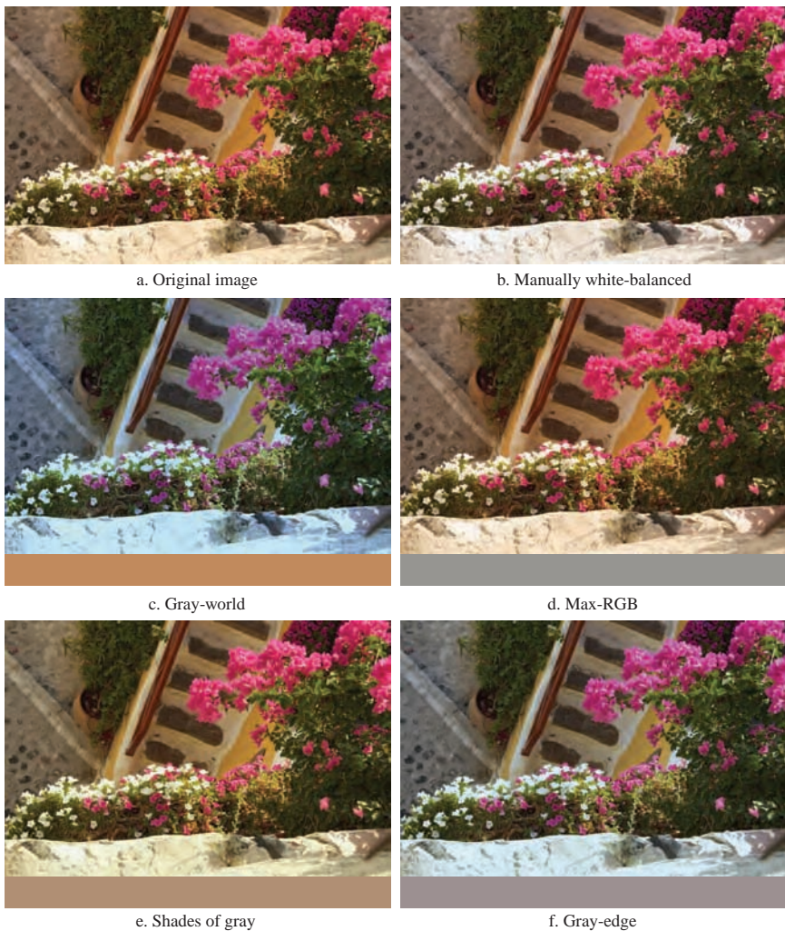
Figure 10.20. Different color constancy algorithms based on the Minkowski norm were used to white-balance the image shown at the top left (a). The algorithms used are given in Table 10.2. The small rectangle below each image shows the white point estimated by each algorithm and the manually white-balanced image is given in (b). (Santorini, Greece, 2009)
