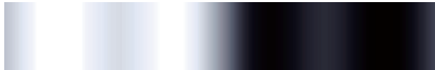
Figure 6.8. Summing a large number of sinusoids (500 in this case) approximates a step edge.
