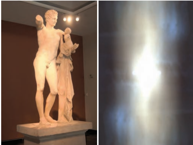
Figure 6.5. The autocorrelation for the left image is shown on the right. The autocorrelation was computed for each of the red, green, and blue channels separately, leading to slight color variations in this image. (Olympia, Greece, 2010)
