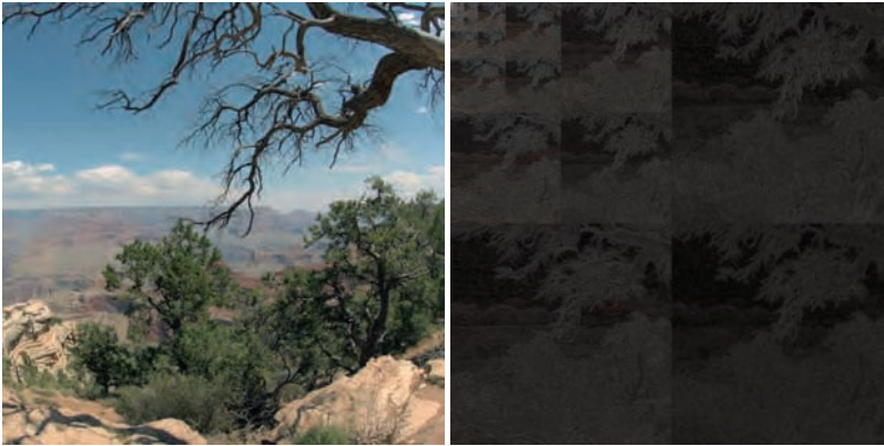
Figure 8.8. A full Haar decomposition. Note that we have passed the resulting images through a gamma curve (exponent 0.2) to help visualize the coefficients. (Grand Canyon, Arizona, 2012)
