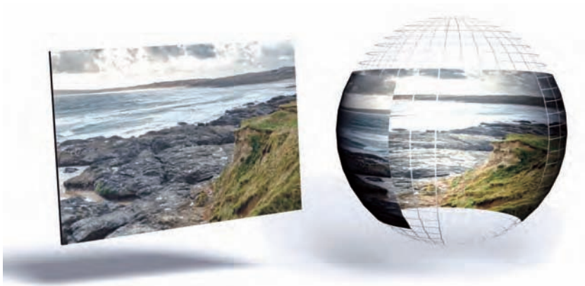
Figure 3.3. A given scene can be represented by a (hemi)sphere, resulting in a 360-degree field of view. Any image from that scene forms a slice on the sphere. To capture the complete scene, several overlapping slices are necessary.
