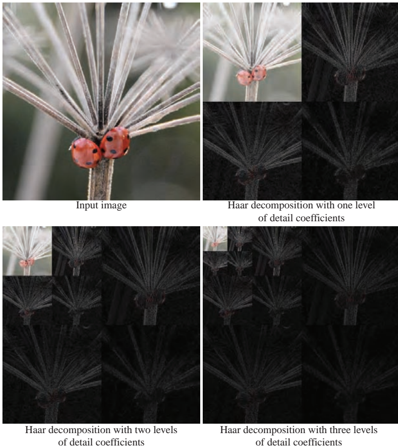
Figure 8.7. One, two, and three levels of Haar decomposition. Note that we have passed the resulting images through a gamma curve (exponent 0.4) to help visualize the coefficients.
