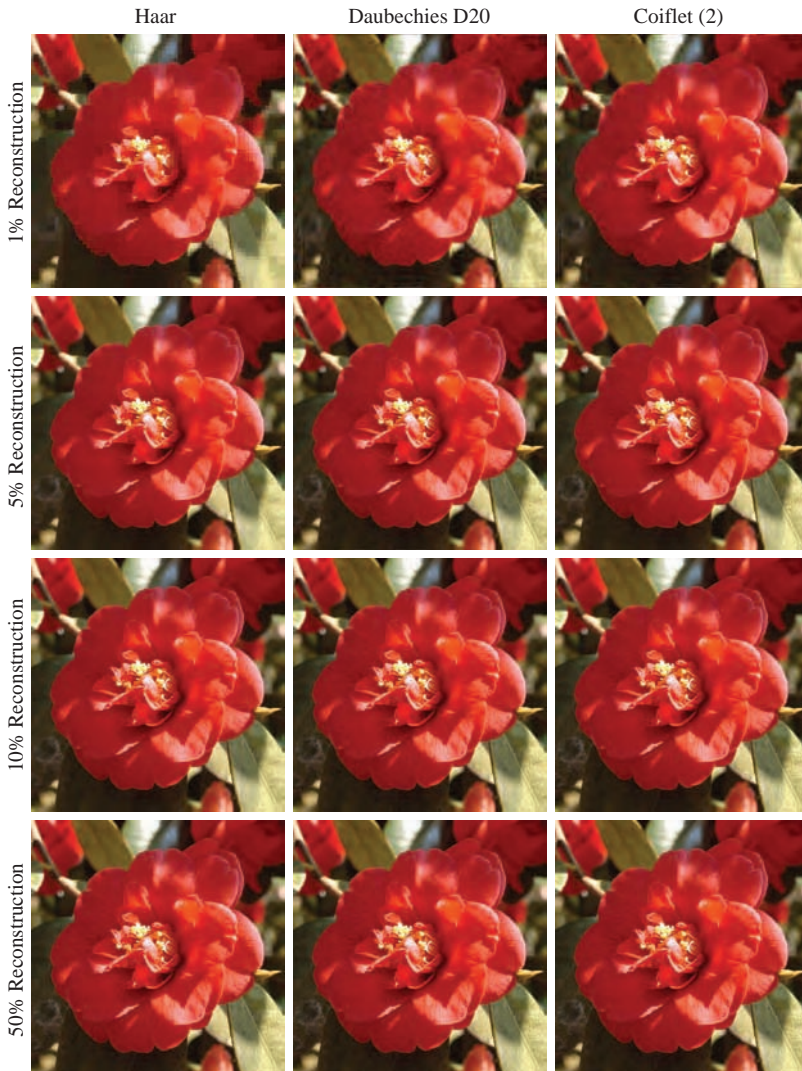
Figure 8.19. Wavelets allow images to be progressively reconstructed, which can be used in transmission. Here, we use the best 1%, 5%, 10%, and 50% of the wavelet coefficients (top to bottom), using three different wavelets (left to right): Haar, Daubechies D20, and Coiflet (2).
