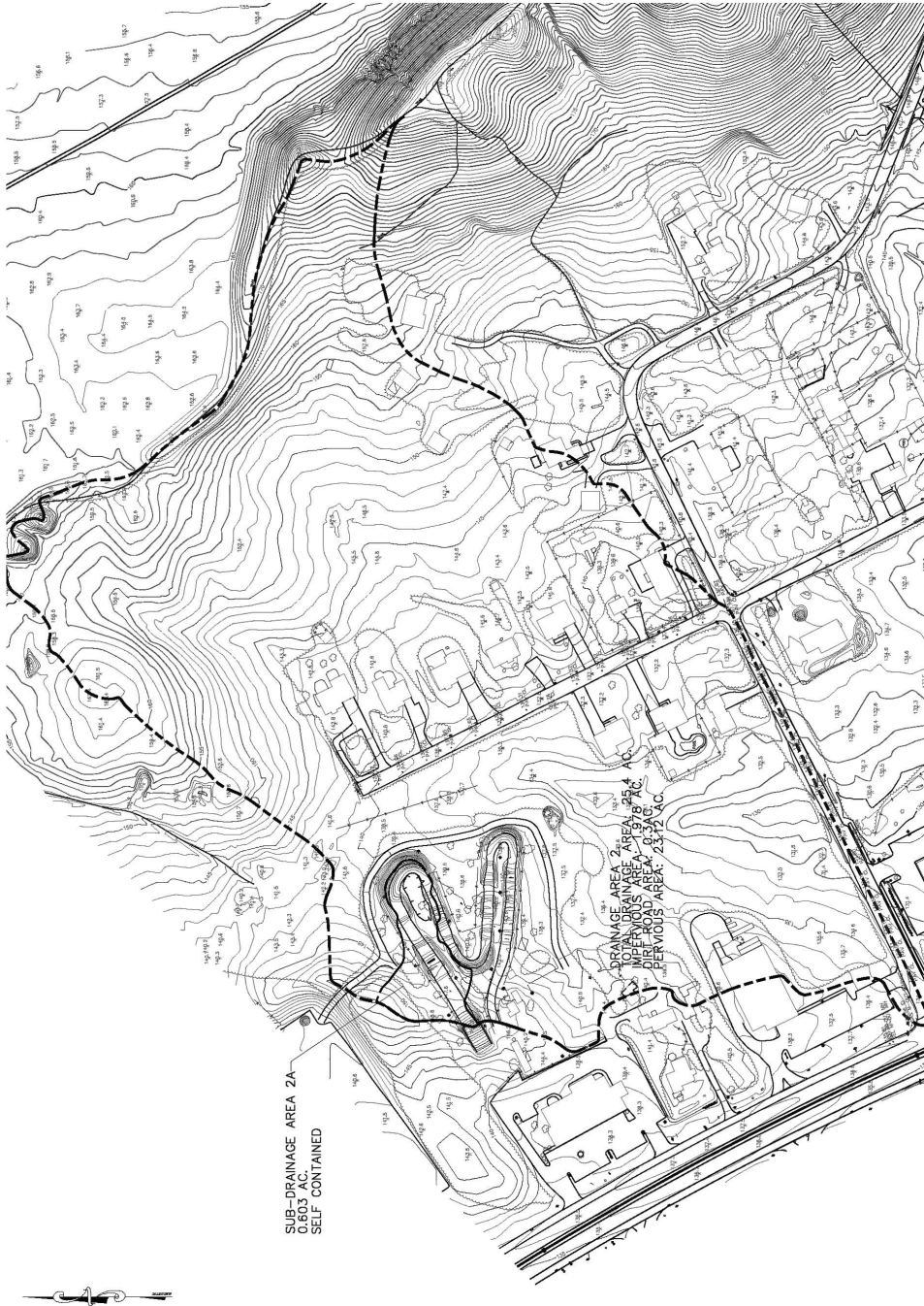
FIGURE 3.25 A drainage area map of a 26.0 acre watershed in Monmouth County in New Jersey.
