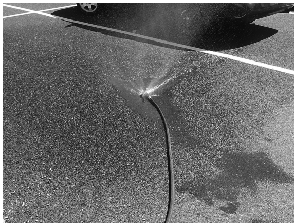
FIGURE 8.6 Experimental porous asphalt, EPA laboratory in Edison, New Jersey.
