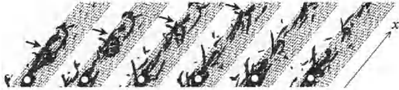
Figure 2. Time evolution of shedded vortices from a sphere visualized by \nabla^2 p isosurfaces
