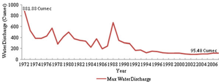
Fig. 4 Yearly maximum water discharge hydrograph of Manas River (1972–2007)
