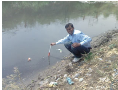
Mantola Drain, Agra [pH = 7.69, EC = 2.687, TDS = 1.657, Turbidity = 71, NH 4 = 7.55, BOD = 77.7, COD = 217.4 (Flow measurement was not performed due to deep sludge)]
