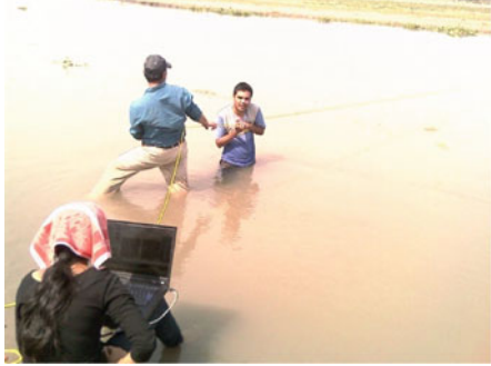
Yamuna at Palla [pH = 7.47, EC = 255.4, TDS = 153, Turbidity = 77, NH 4 = 0.13, BOD = 4.77, TC = 67,066, FC = 7,033, DO = 5.5, Q = 11 cumec]
