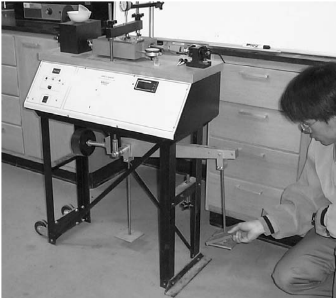
Fig. 12.8 – Applying normal load to the specimen using a dead weight system. The system shown in the photograph has a 10:1 mechanical advantage.
