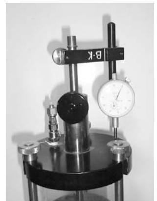
b. Top of triaxial cell with cell bars in place. Vent valve is also shown.
