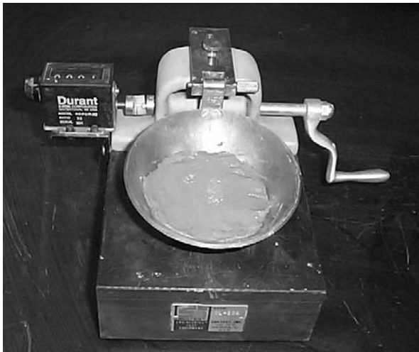
Fig. 4.3—Spread a flat layer of soil in the liquid limit device cup prior to grooving.
