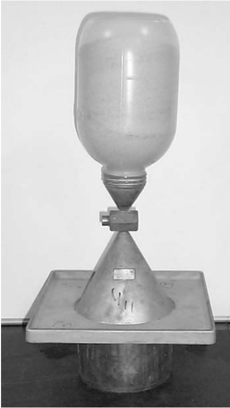
Fig. 9.3 – Filling the base plate, funnel, and calibration chamber with sand for calibration.
