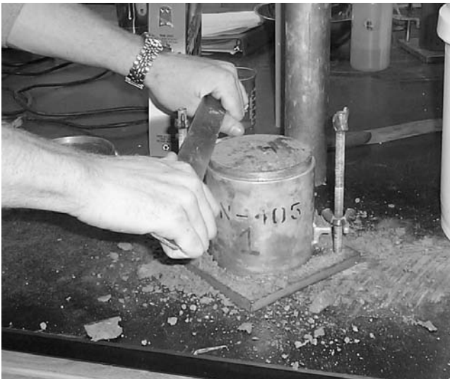
Fig. 8.4—Trimming excess soil from the top of the mold using the cutting bar.
