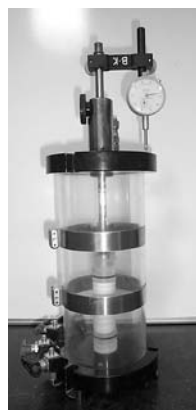
a. Cell wall and top in position, with piston seated in the cap.
