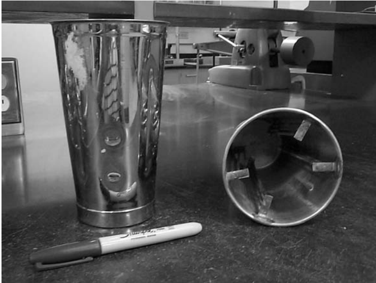
Fig. 5.3—ASTM D422-specified dispersion cup (2 cups shown with pen for scale; note the bafflers inside the cup).
