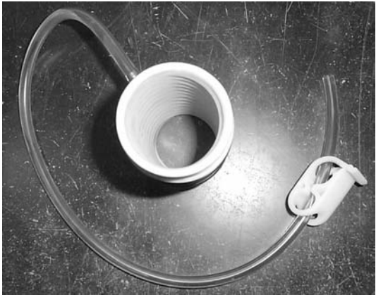
c. membrane pulled against inside wall of membrane stretcher using a light vacuum
