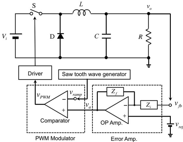
**Figure 5.1** A buck converter with a fixed switching frequency voltage-mode PWM controller.
