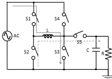
**Figure 8.16** H bridge AC–DC converter (current when  $V_{in} < 0$ ).
