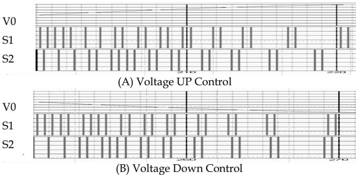
**Figure 8.4** Output pulses of dual  $\Delta\Sigma$  modulators.
