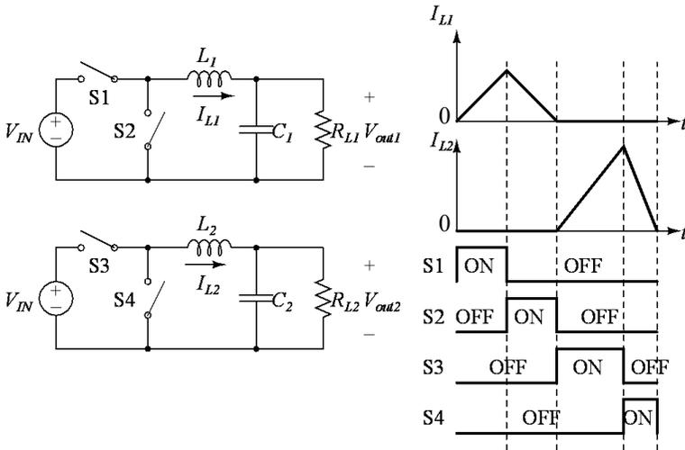
Figure 9.8 Timing diagram of S1-S4 and inductor currents of L1 and L2.
