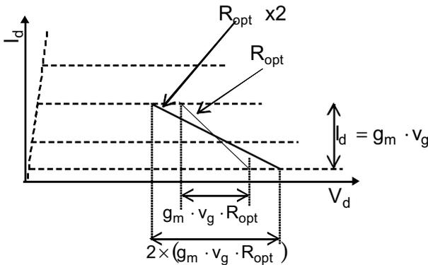
**Figure 12.35** Voltage swing at  $R_{opt}$  and  $R_{opt} \times 2$ .
