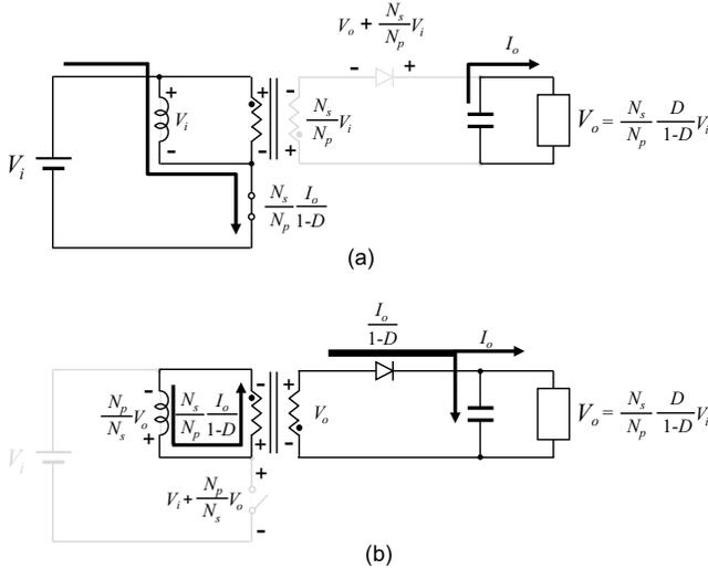
**Figure 3.3** Equivalent circuits for each operation state. (a)  $t_0 - t_1$  and (b)  $t_1 - t_2$ .
