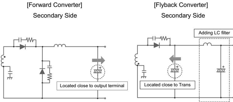
**Figure 6.40** Capacitor optimum location for a forward converter and a flyback converter.
