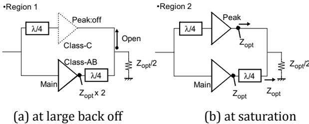
Figure 12.27 Situation at saturation and back-off power region.
