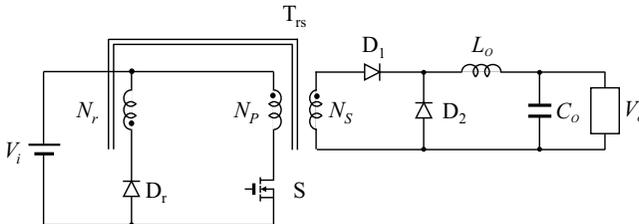
**Figure 3.6** Ideal single-switch forward converter.
