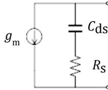
Figure 12.6  $C_{ds}$  with  $R_s$ .
