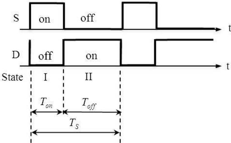
Figure 4.2 Switching state.
