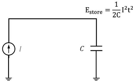
**Figure 1.6** Ideally a current source can provide energy to a capacitor indefinitely without loss.
