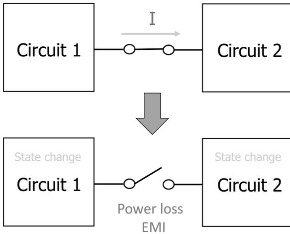
**Figure 1.18** Switch turns off when  $I \neq 0$ .
