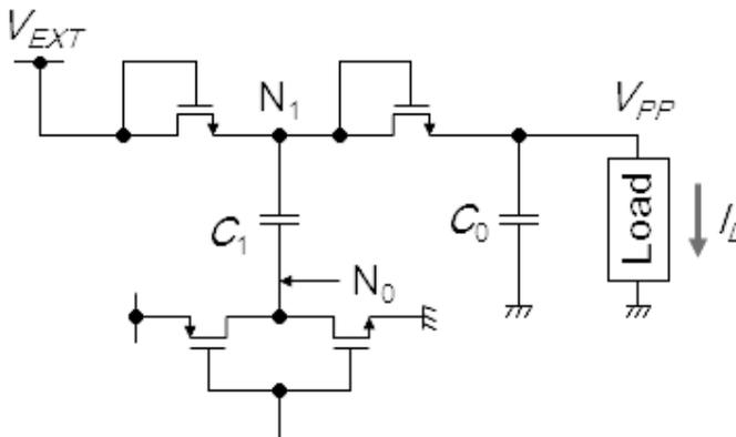
**Figure 7.27** Charge pump voltage doubler.
