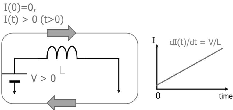
**Figure 1.2** Current can flow through an inductor from higher-voltage to lower-voltage nodes.
