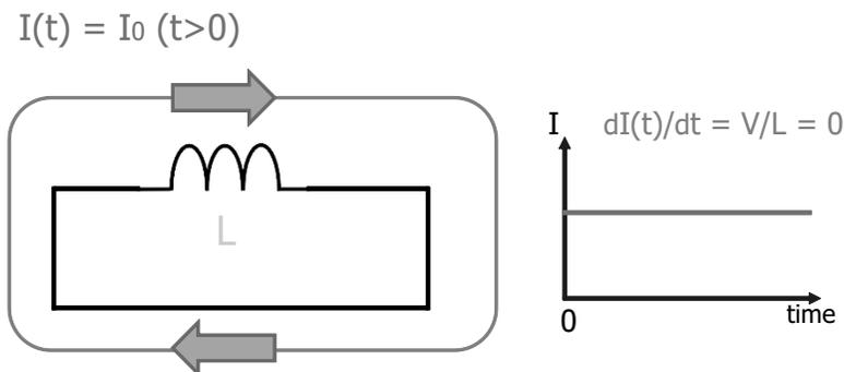
**Figure 1.3** Constant current flows in an inductor loop, which is a current memory.
