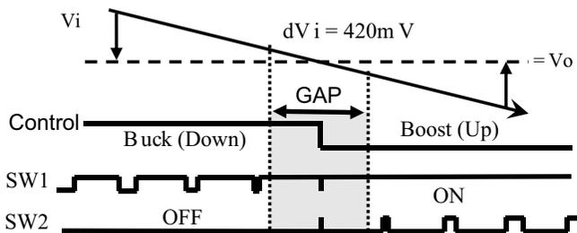
**Figure 8.1** Mixed-control buck–boost converter.
