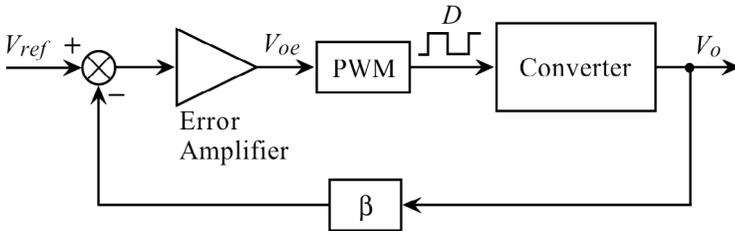
**Figure 2.12** Block diagram of the regulator system.
