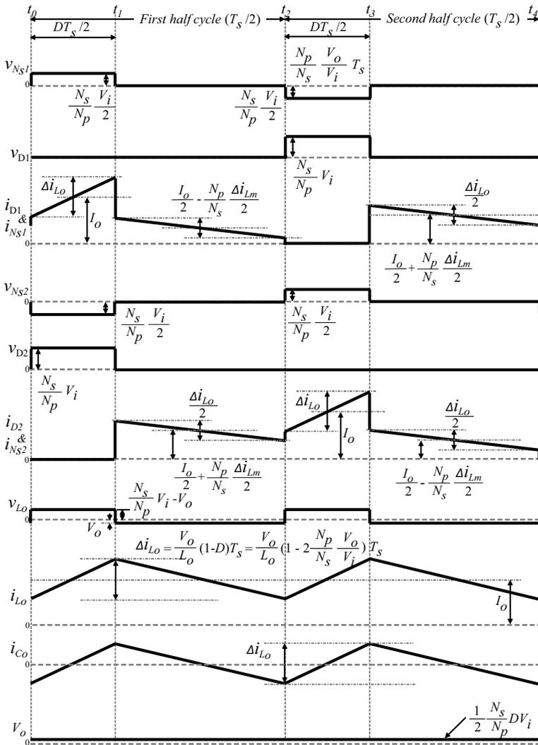
**Figure 3.21** Typical waveforms of a half-bridge converter.
