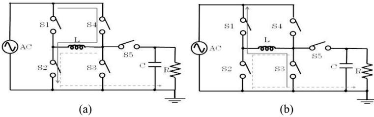
**Figure 8.25** Inverting H bridge AC–DC converter. (a) Current flow when  $V_i > 0$ . (b) Current flow when  $V_i < 0$ .
