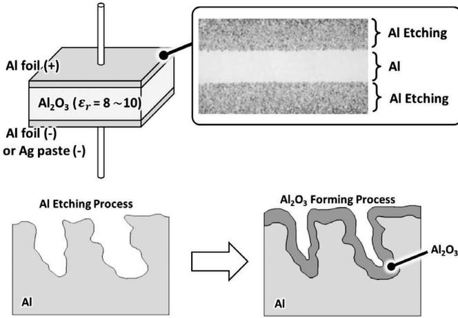
**Figure 6.12** Aluminum foil etching and dielectric (Al<sub>2</sub>O<sub>3</sub>) forming.
