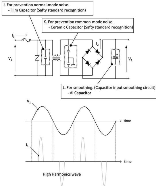
**Figure 6.41** Input voltage and current waveform without a PFC circuit.
