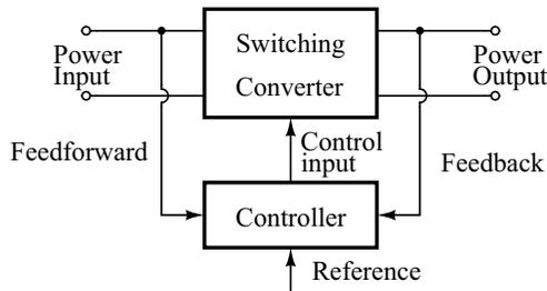
**Figure 9.1** Basic schematic of a switching regulator.
