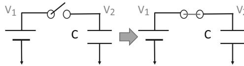
**Figure 1.9** A voltage source and a capacitor do not have a good relationship.
