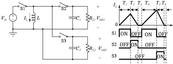
**Figure 9.17** Schematic of a SIMO converter using two negative buck–boost converters.
