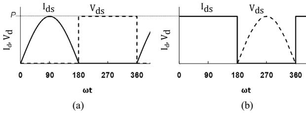
**Figure 12.17** Waveforms of (a) class F and (b) inverse class F.
