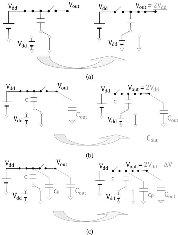
**Figure 13.6** Charge pump circuit. (a) Principle of high voltage generation. (b) Charge pump circuit with output capacitor  $C_{out}$ . (c) Charge pump circuit with parasitic capacitor in parallel with output capacitor  $C_{out}$ .
