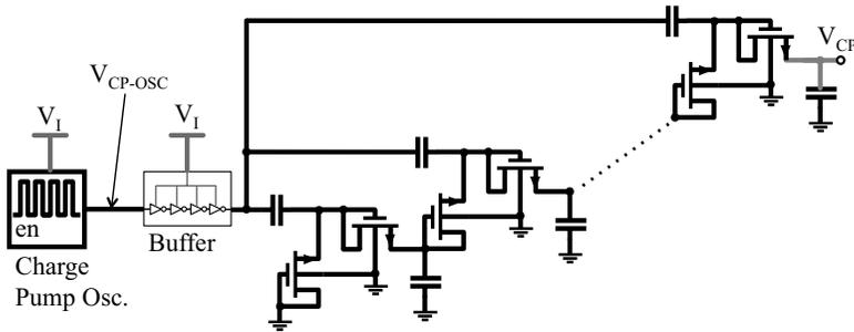
**Figure 10.4** Full charge pump schematic.
