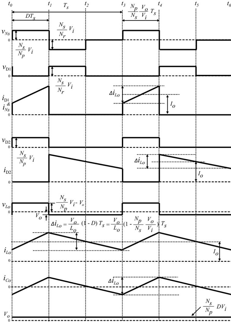
**Figure 3.9** Typical waveforms of a single-switch forward converter.
