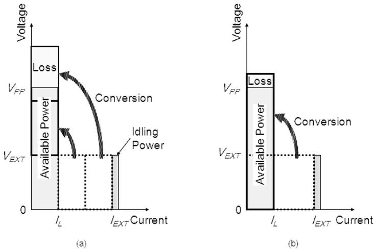
**Figure 7.25** Comparison of power conversion efficiencies of voltage up-converters; (a) charge pump and switched capacitor; (b) switching converter.
