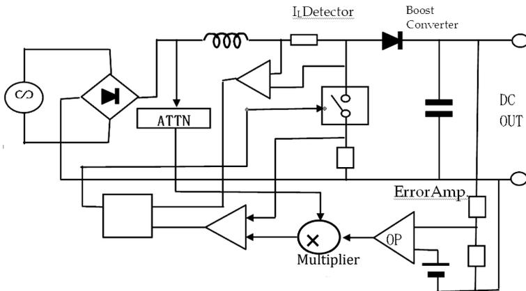
Figure 8.28 Conventional PFC circuit in BCM.
