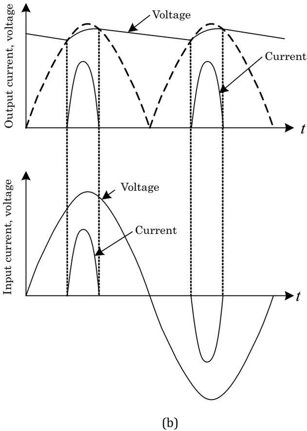
**Figure 1.25** (a) Circuit and (b) waveforms of a conventional diode bridge rectifier.
