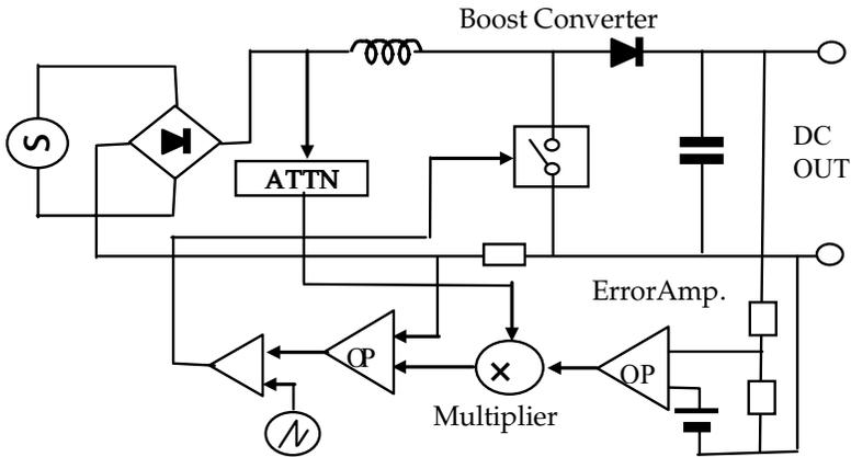
Figure 8.35 Conventional CCM PFC circuit.
