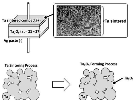
**Figure 6.17** Sintered tantalum and dielectric ( $Ta_2O_5$ ) forming.
