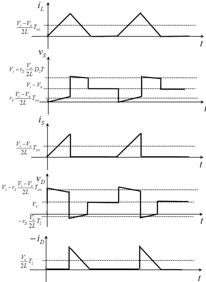
**Figure 4.11** Waveforms of currents and voltages of S and D.
