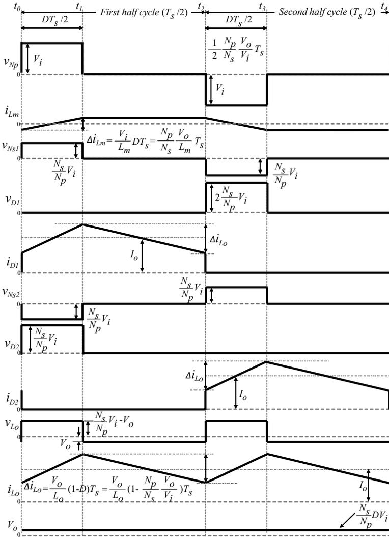
**Figure 3.25** Typical waveforms of a PWM-controlled full-bridge converter.
