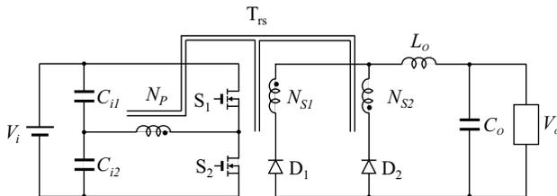
**Figure 3.18** Ideal half-bridge converter.
