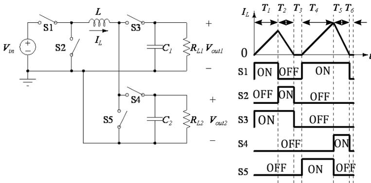
**Figure 9.10** Schematic of a SIMO converter using buck and boost converters.
