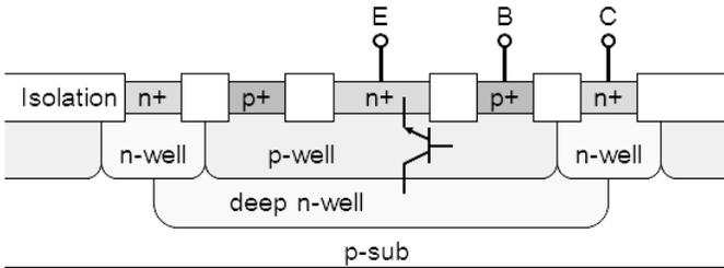
**Figure 7.13** Cross section of a parasitic npn bipolar transistor.
