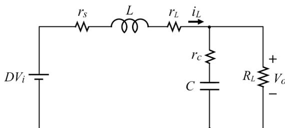
**Figure 2.8** Averaged equivalent circuit.
