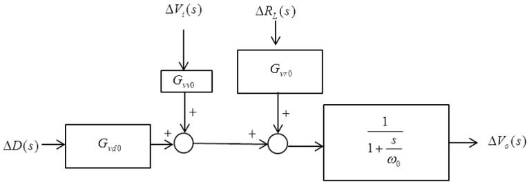
Figure 4.15 Small-signal model for DCM.
