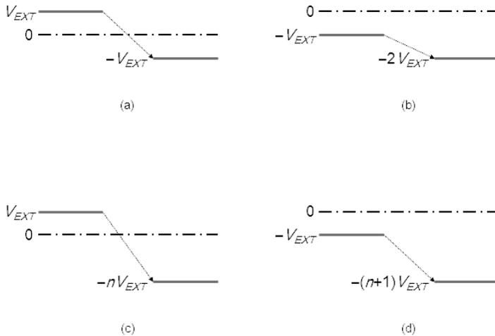
**Figure 7.28** Principle of voltage inversion.
