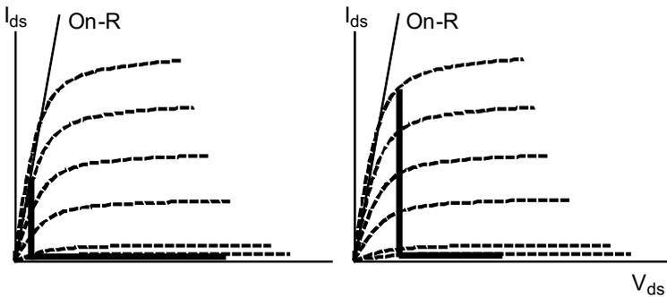
**Figure 12.20** Switching load line for class F and inverse class F.
