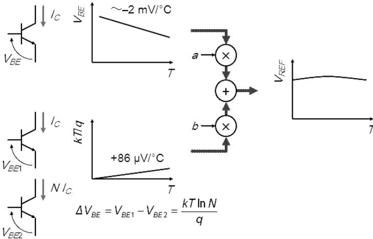
**Figure 7.9** Principle of a bandgap reference (BGR).
