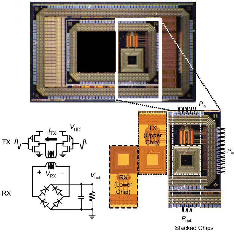
**Figure 11.2** Microphotograph of stacked chips and schematic of wireless interchip power delivery. Copyright (2009), The Japan Society of Applied Physics.
