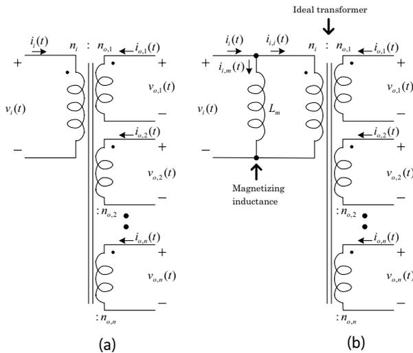
**Figure 1.23** (a) Multiple-winding transformer circuit and (b) its equivalent circuit containing a magnetizing inductance and an ideal transformer.
