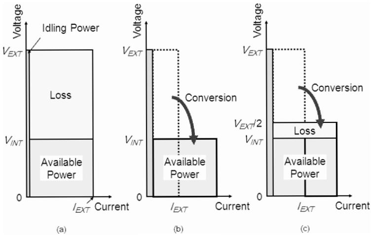
**Figure 7.19** Comparison of power conversion efficiencies of voltage down-converters.
