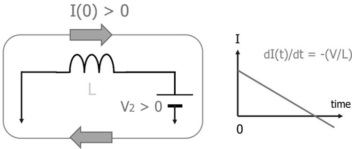
**Figure 1.1** Current can flow through an inductor from lower-voltage to higher-voltage nodes.
