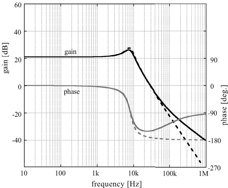
**Figure 2.13** Frequency response of an open-loop transfer function.
