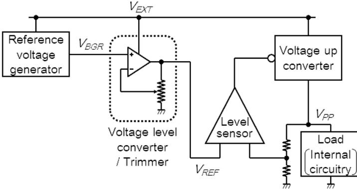
**Figure 7.7** Schematic of an on-chip voltage up-converter.
