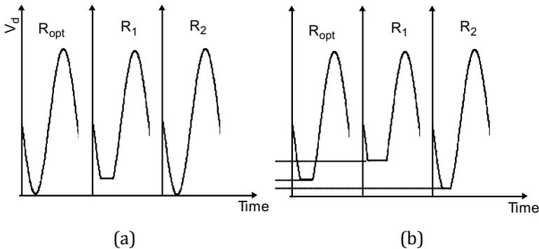
**Figure 12.30** Voltage waveform (a) without and (b) with  $R_{\text{on}}$ .
