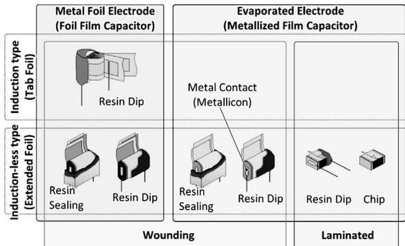
**Figure 6.22** Types of electrodes and structures.
