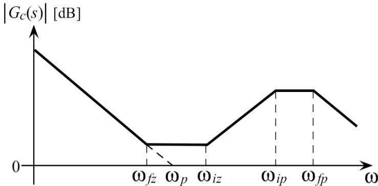
**Figure 2.15** Gain versus frequency of an error amplifier with phase compensation networks.
