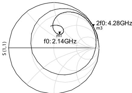
**Figure 12.24** Simulated load impedance.
