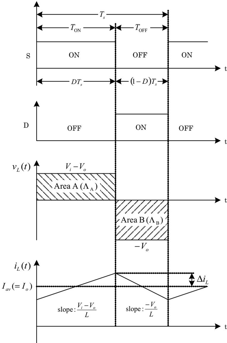
**Figure 1.21** Steady-state inductor voltage and current waveforms in a buck converter.
