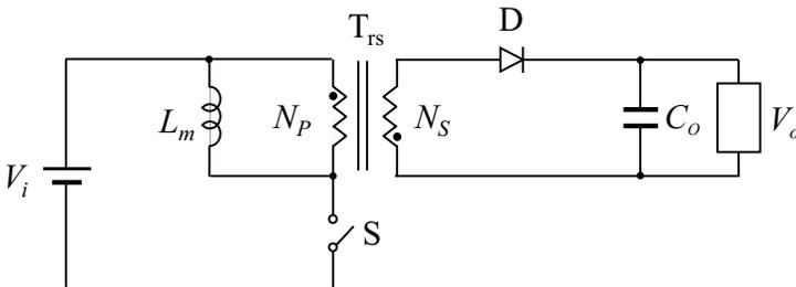
**Figure 3.2** Flyback converter with the transformer-equivalent circuit.
