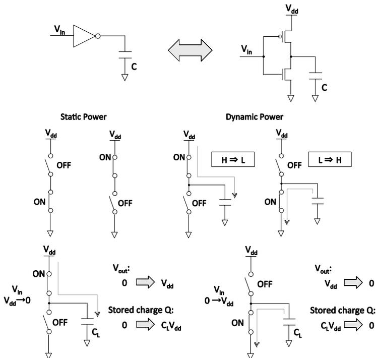
Figure 13.11 Dynamic power dissipation CMOS circuit.
