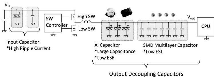
**Figure 6.28** Decoupling circuit for a CPU.
