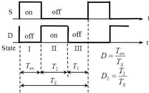
**Figure 4.9** Switching state in discontinuous conduction mode.
