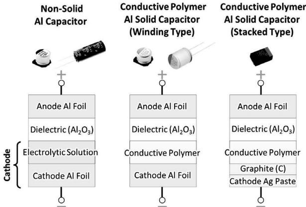
**Figure 6.13** Basic model of an aluminum electrolytic capacitor.
