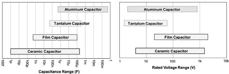
**Figure 6.11** Capacitance range/rated voltage range.
