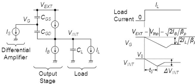
**Figure 7.23** Large-signal equivalent circuit of a series regulator (a) and step-response waveforms (b).
