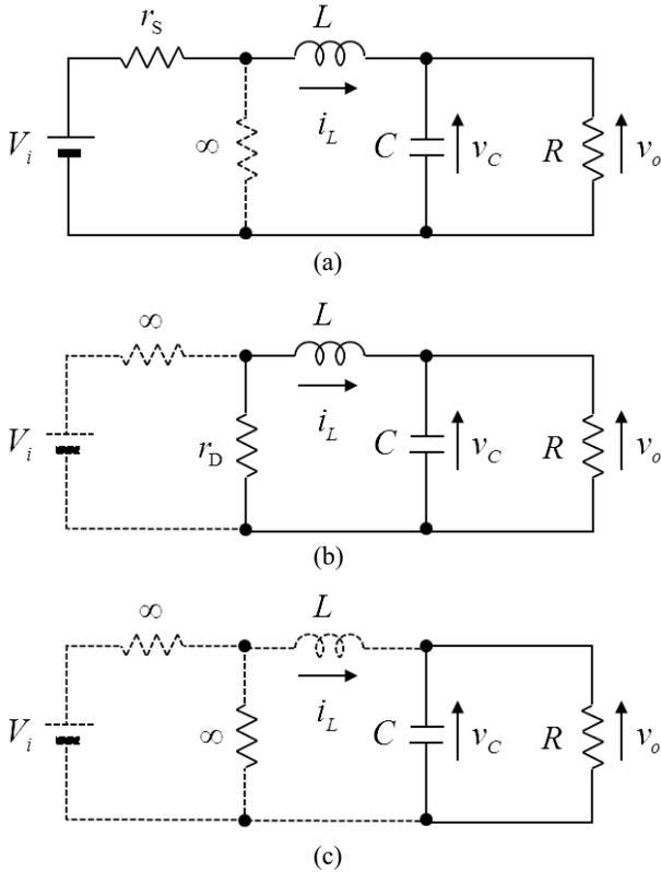
**Figure 4.10** Equivalent circuits in discontinuous conduction mode. (a) State I, (b) state II, and (c) state III.
