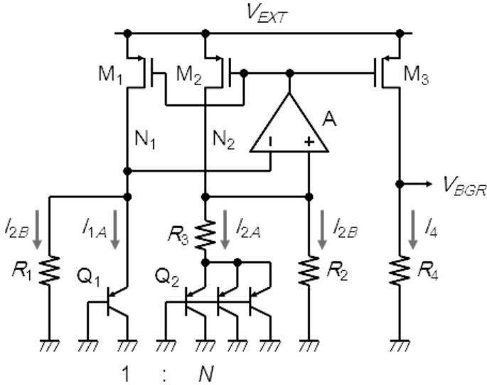
**Figure 7.15** Low-voltage bandgap reference circuit [25].
