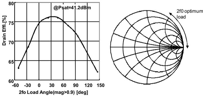
Figure 12.18 Load pull measurement results.
