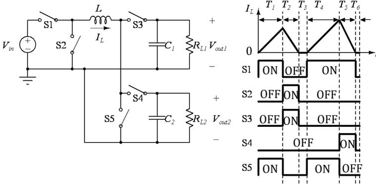
**Figure 9.13** Schematic of a SIMO converter using boost and positive buck–boost converters.
