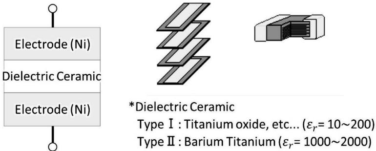
**Figure 6.26** Basic model of a ceramic capacitor (nonpolarity).
