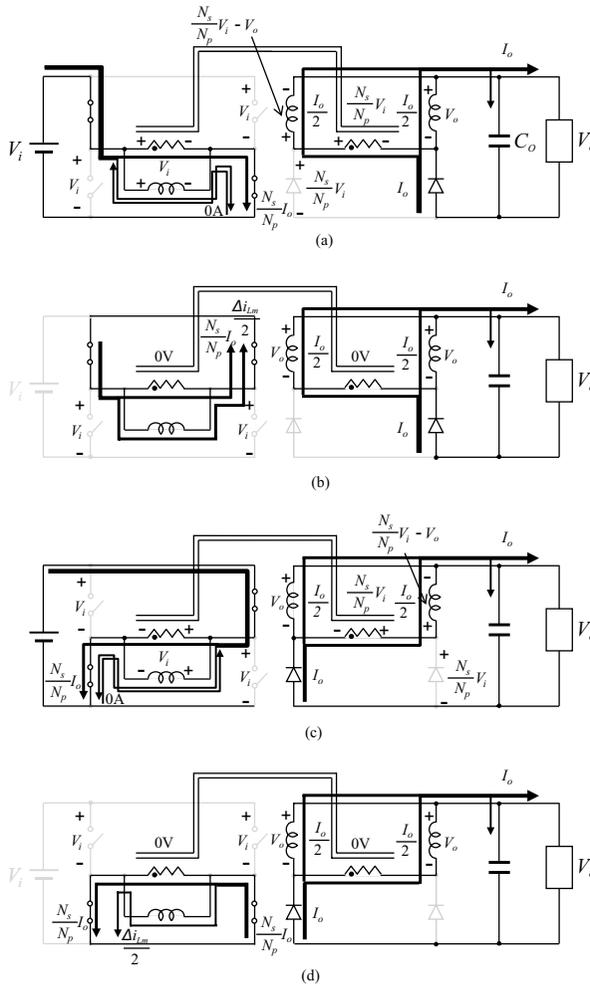
**Figure 3.29** Equivalent circuits for each operation state with a current-doubler circuit. (a)  $t_0 - t_1$ , (b)  $t_1 - t_2$ , (c)  $t_2 - t_3$ , and (d)  $t_3 - t_4$ .
