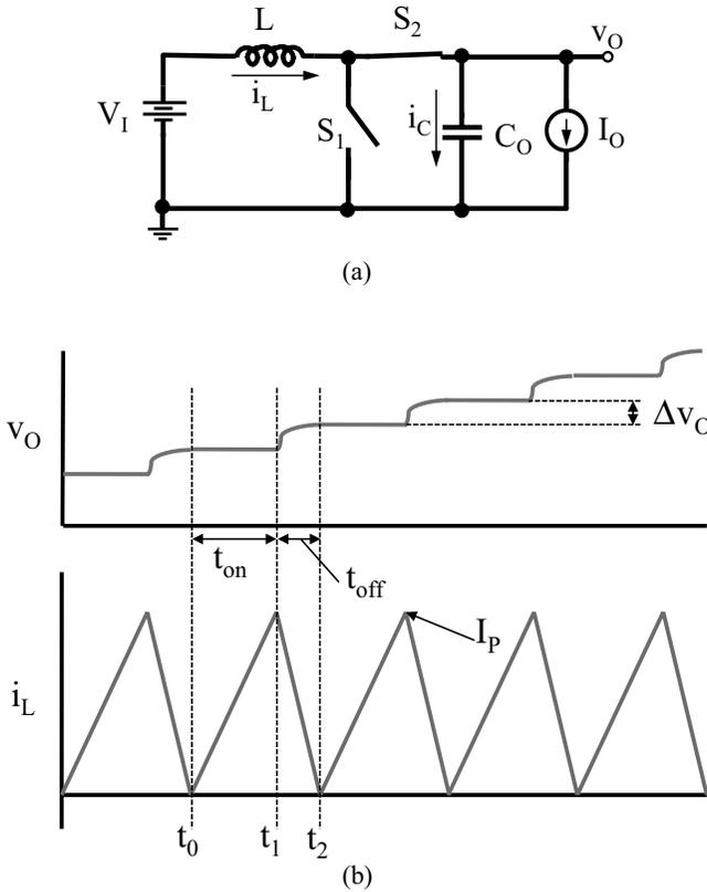
**Figure 10.10** Constant on-time voltage ripple analysis. (a) Off-time schematic. (b) Switching inductor current and output voltage.
