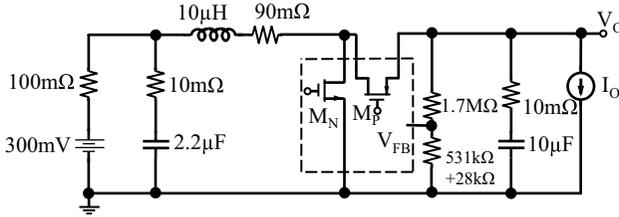
**Figure 10.11** Simulation schematic including parasitic resistances.
