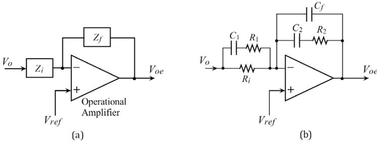
**Figure 2.14** Error amplifier with phase compensation.
