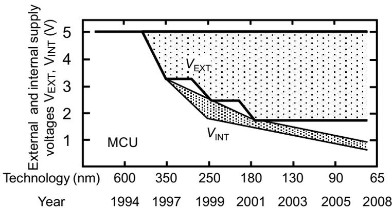
**Figure 7.2** Trends in external and internal supply voltages of microcontrollers [15].
