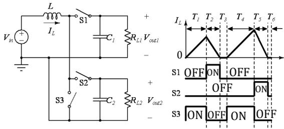
**Figure 9.11** Schematic of a SIMO converter using two boost converters.
