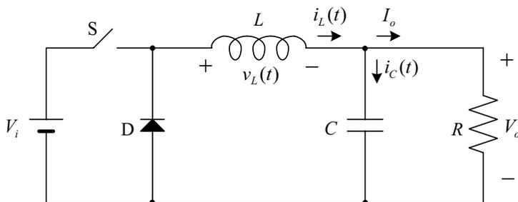
**Figure 1.20** Buck converter circuit.
