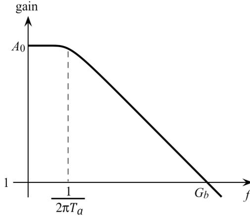
**Figure 2.16** Frequency response of open-loop gain for a first-order lag circuit.
