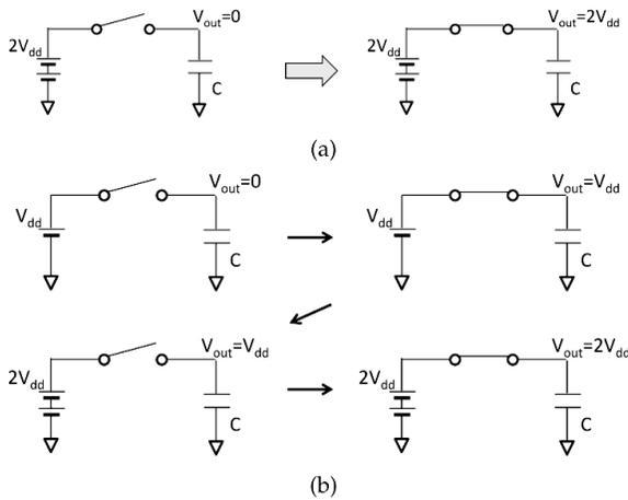
**Figure 13.8** Capacitor charging to  $2CV_{\text{dd}}$ . (a) Method 1. (b) Method 2.
