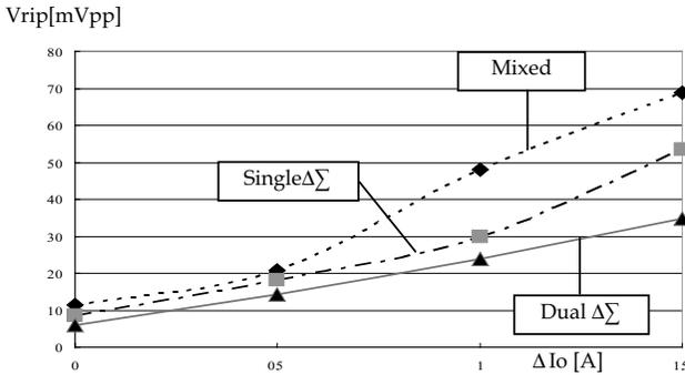
**Figure 8.7** Output ripple versus load current step.
