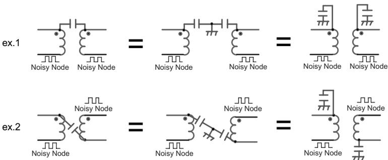
**Figure 6.39** Line bypass capacitor for isolated transformer.
