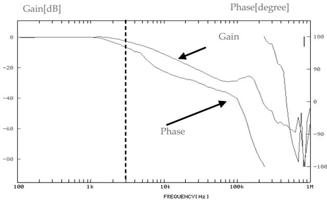
**Figure 8.15** Closed-loop characteristics of an experimental circuit.
