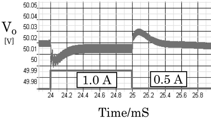
**Figure 8.22** Load transient response.
