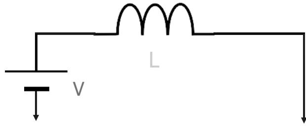
**Figure 1.4** Ideally a voltage source can provide energy to an inductor indefinitely without loss.
