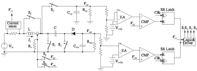
**Figure 9.23** Schematic of the current-mode control of Fig. 9.21.
