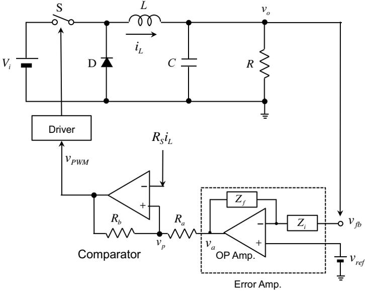
**Figure 5.7** A buck converter with a current-mode PWM controller.
