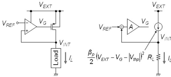
**Figure 7.21** A pMOSFET output series regulator (a) and its large-signal equivalent circuit (b).
