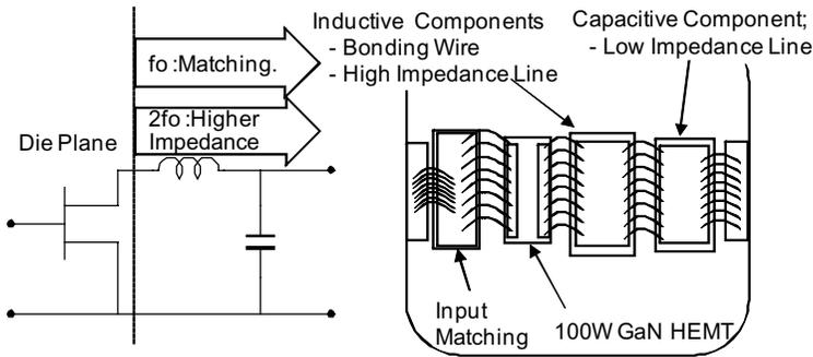
**Figure 12.23** High-power class F concept.
