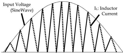
Figure 8.29 Waveform of the inductor current in BCM.
