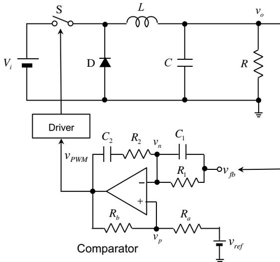
**Figure 5.3** A buck converter with a hysteretic PWM controller.
