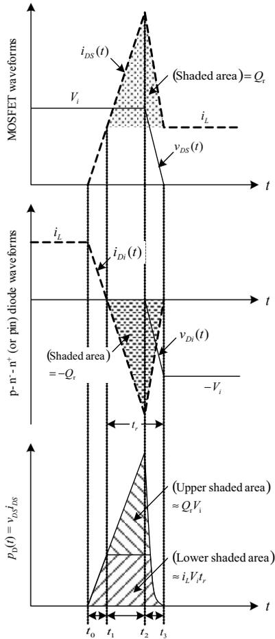
**Figure 1.29** MOSFET turn-on transition piecewise-linear waveforms for the buck converter circuit in Fig. 1.28.
