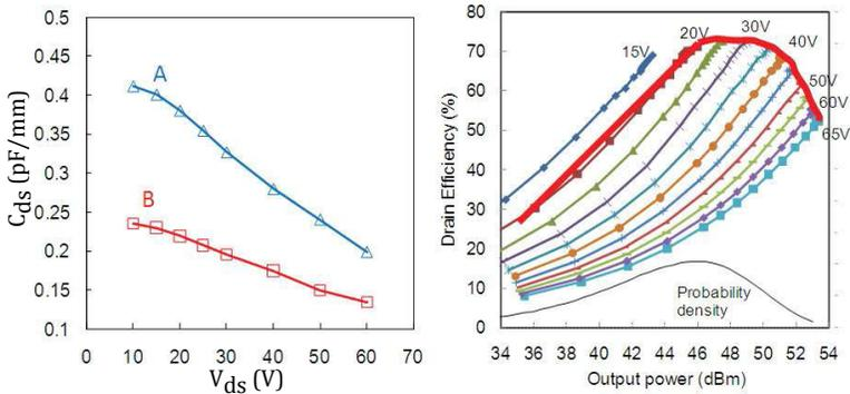
**Figure 12.41**  $C_{ds}$  linearity improvement and efficiency for ET.
