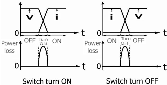
Figure 1.15 Switching loss.
