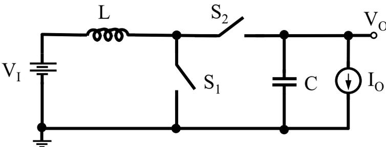
Figure 10.1 Ideal synchronous boost converter.
