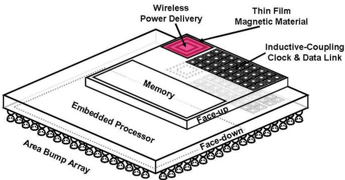
**Figure 11.3** Concept of 3D system integration with wireless power delivery using thin-film magnetic material. Copyright (2009), The Japan Society of Applied Physics.
