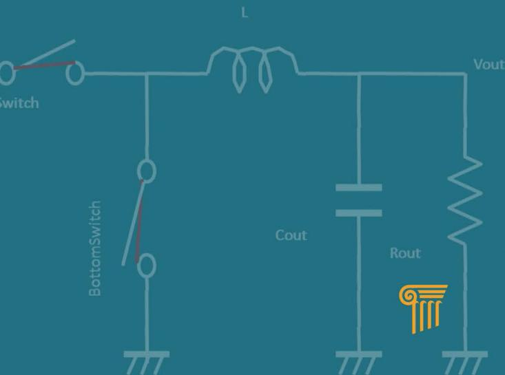
$$V_{out} = \frac{T_{on}}{T_{on} + T_{off}} V_{in}$$
