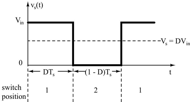
Figure 9.3 Switch output voltage waveform.
