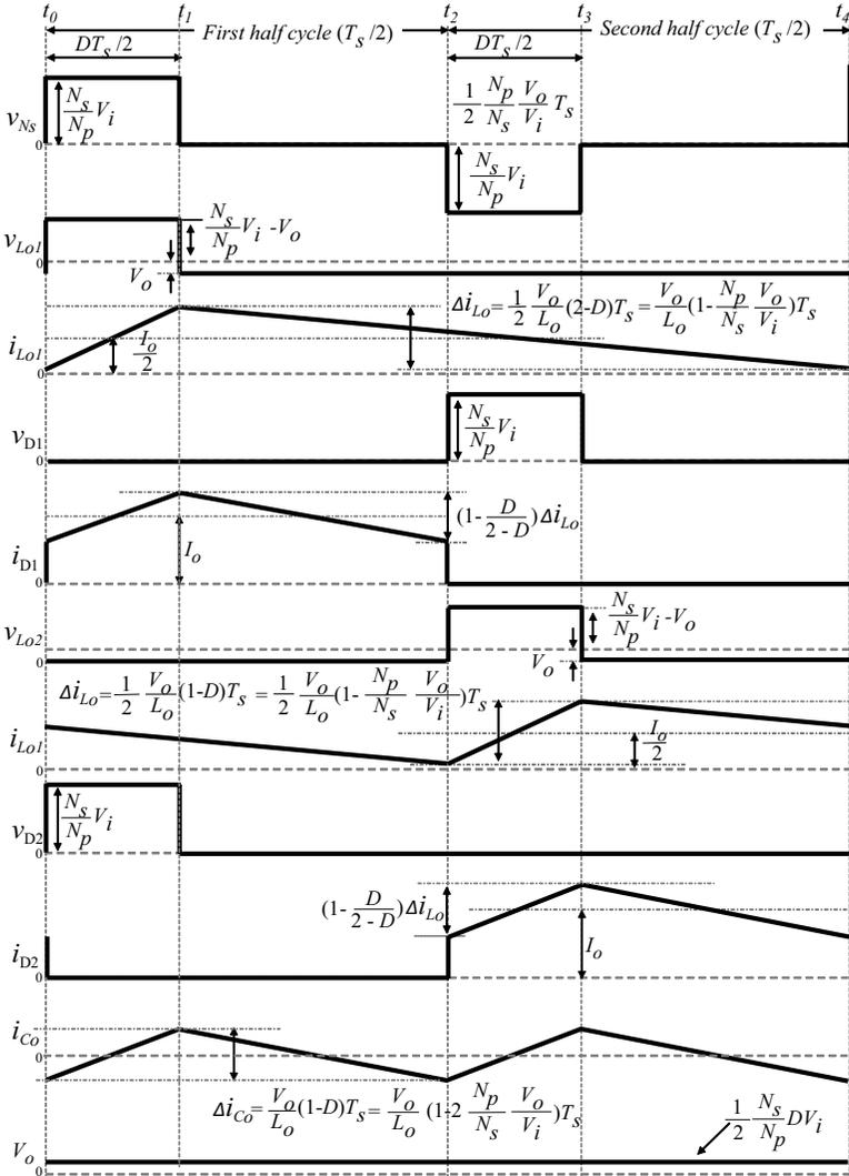
Figure 3.30 Typical waveforms of a current-doubler circuit.
