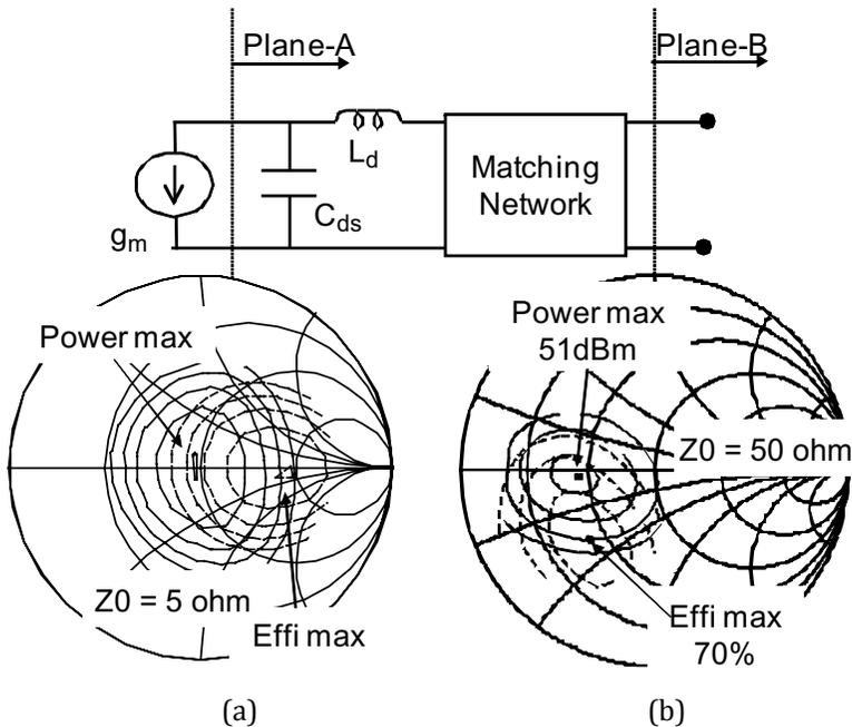
**Figure 12.31** Load pull at (a) plane A (simulated) and (b) plane B (measurement).
