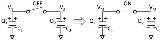
**Figure 13.4** Two capacitors and a switch. (a) When the switch is off, the voltages across  $C_1$  and  $C_2$  are  $V_1$  and  $V_2$ , respectively. (b) When the switch is on, the charges in  $C_1$  and  $C_2$  move so that the voltages across  $C_1$  and  $C_2$  become the same ( $V_M$ ), and some energy is dissipated in the switch.
