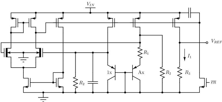
**Figure 10.7** Banba bandgap voltage reference.
