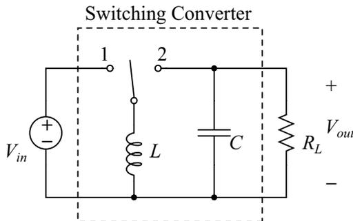
**Figure 9.5** Schematic of a buck–boost converter.
