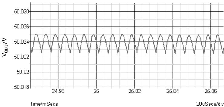
**Figure 8.21** Output voltage ripple.
