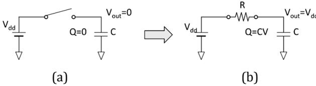
**Figure 13.3** Charging a capacitor.
