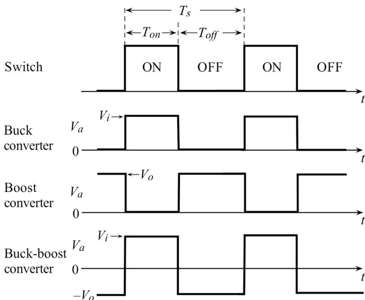
**Figure 2.2** States of the switch and the voltage waveforms of  $V_a$ .
