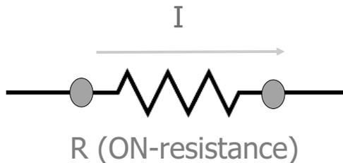
**Figure 1.14** Conduction loss  $P = RI^2$  when the switch is on.
