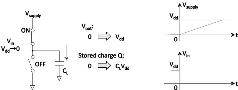
Figure 13.12 Principle of adiabatic digital CMOS circuit.
