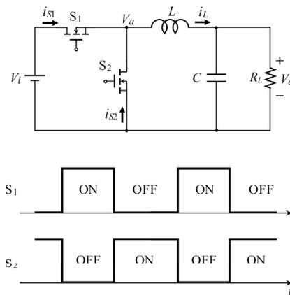
**Figure 2.5** Circuit configuration of a buck converter and states of switches  $S_1$  and  $S_2$ .
