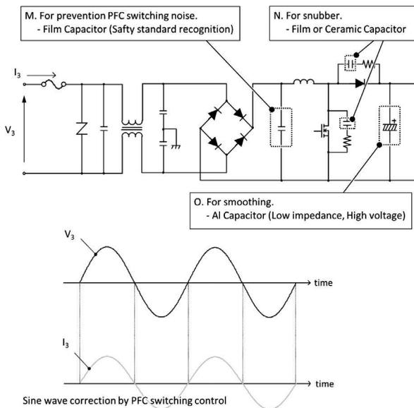
**Figure 6.43** Input voltage and current waveform with a PFC circuit.
