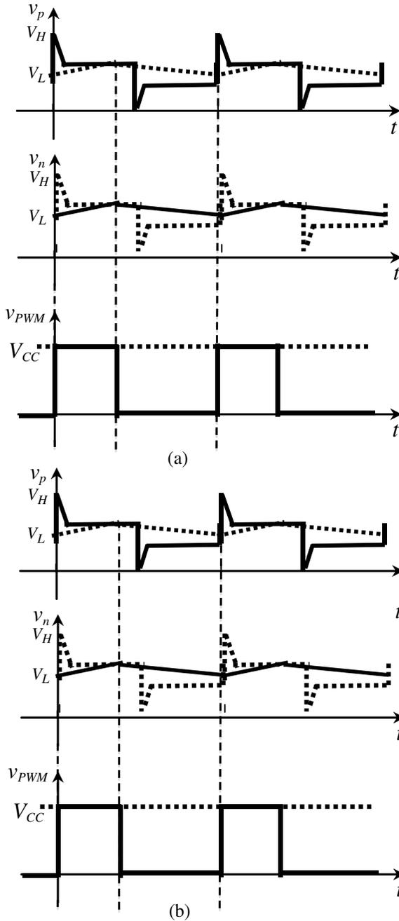
**Figure 5.6** Operating waveforms of a constant-frequency hysteretic PWM generator. (a)  $D < 0.5$  and (b)  $D > 0.5$ .
