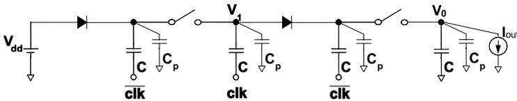
**Figure 13.21** A non-ideal three-stage Dickson charge pump circuit where the voltage drop  $V_d$  across each switch capacitance  $C_p$  at each node and the output load current  $I_{out}$  are considered.
