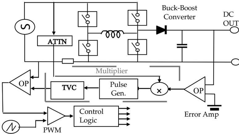
Figure 8.37 New CCM PFC with an H bridge.
