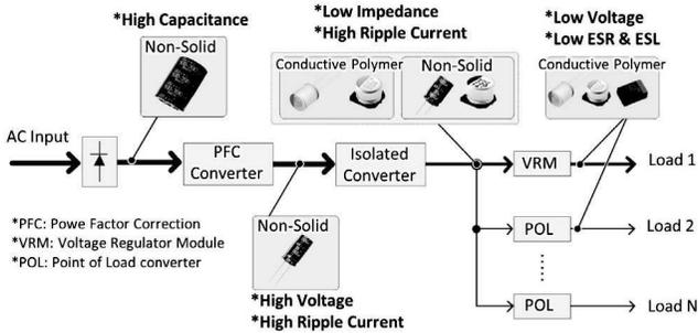
**Figure 6.16** Usage of aluminum electrolytic capacitors in a power distribution network.
