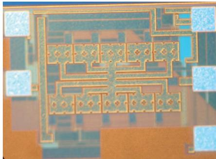
**Figure 10.17** Charge pump test chip.
