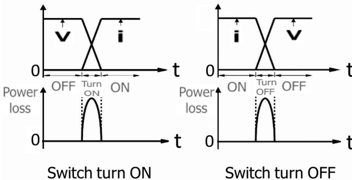
**Figure 13.2** Switching loss (which is ignored in this chapter). (a) When the switch is turned on and (b) when the switch is turned off.
