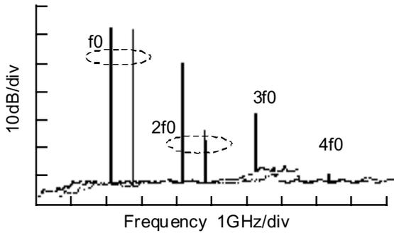
**Figure 12.15** Spectrum of class C and class E operations.
