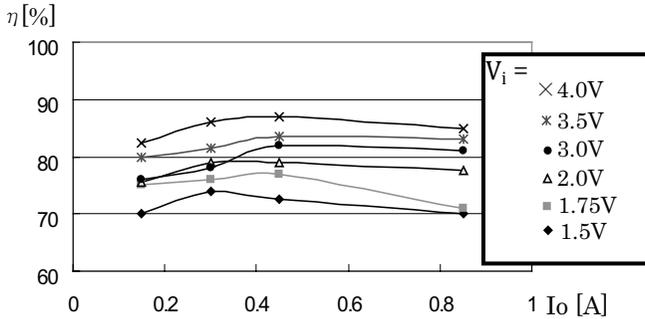
Figure 8.8 Efficiency versus input voltage.
