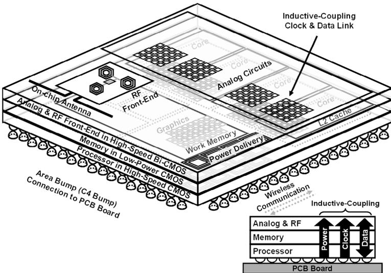
**Figure 11.1** Concept of wirelessly connected 3D system integration. Copyright (2009), The Japan Society of Applied Physics.
