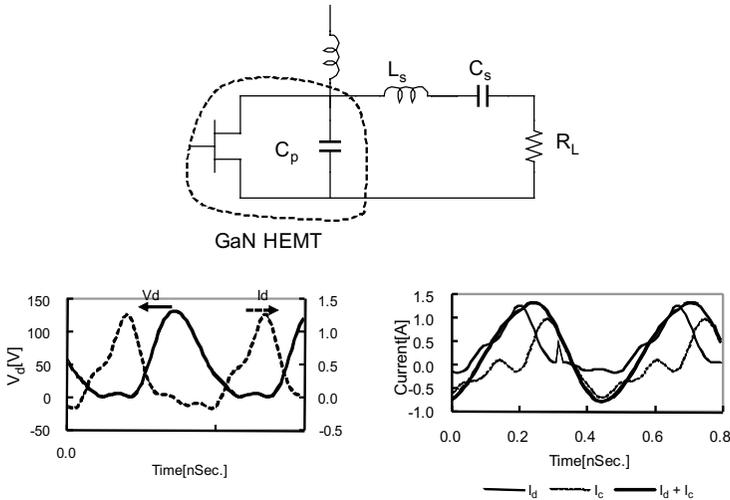
**Figure 12.9** Simulated class E waveform.
