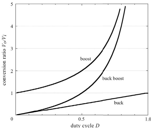
**Figure 2.3** Voltage conversion ratio  $V_o / V_i$ .
