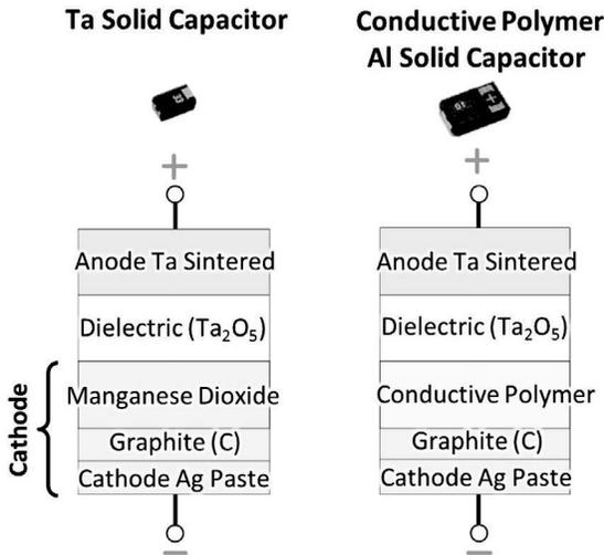
**Figure 6.18** Basic models of a tantalum solid electrolytic capacitor.
