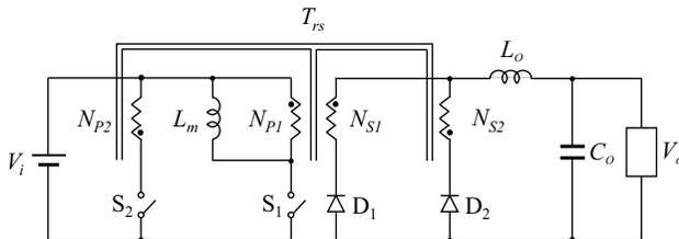
**Figure 3.15** Push–pull converter with the transformer-equivalent circuit.
