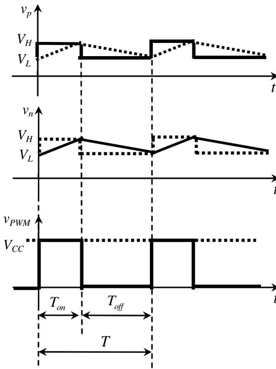
**Figure 5.4** Operating waveforms of a comparator.
