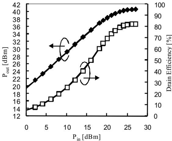
**Figure 12.12** Power characteristics of a 10 W class E amplifier.
