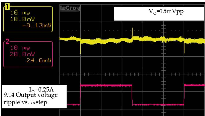
**Figure 8.14** Output voltage ripple versus  $I_o$  step.
