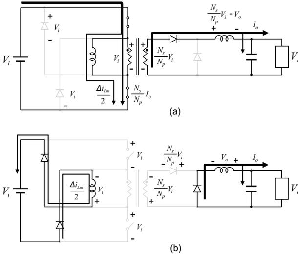
**Figure 3.12** Equivalent circuits for each operation state. (a)  $t_0 - t_1$  and (b)  $t_1 - t_2$ .
