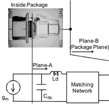
**Figure 12.28** Definition of a reference plane.
