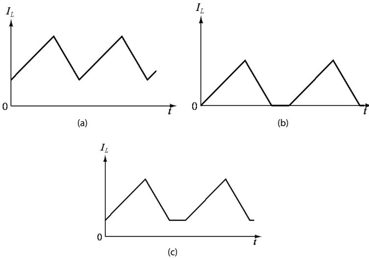
**Figure 9.6** Inductor current waveforms. (a) Inductor current waveform of CCM. (b) Inductor current waveform of DCM. (c) Inductor current waveform of PCCM.
