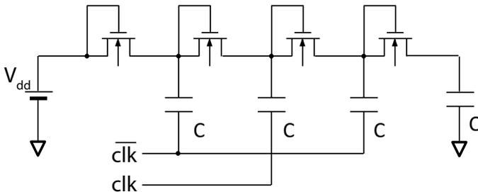
Figure 13.16 A three-stage Dickson charge pump.
