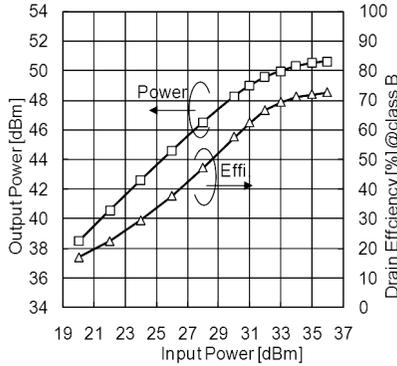
**Figure 12.25** Power characteristics of a 100 W class F.
