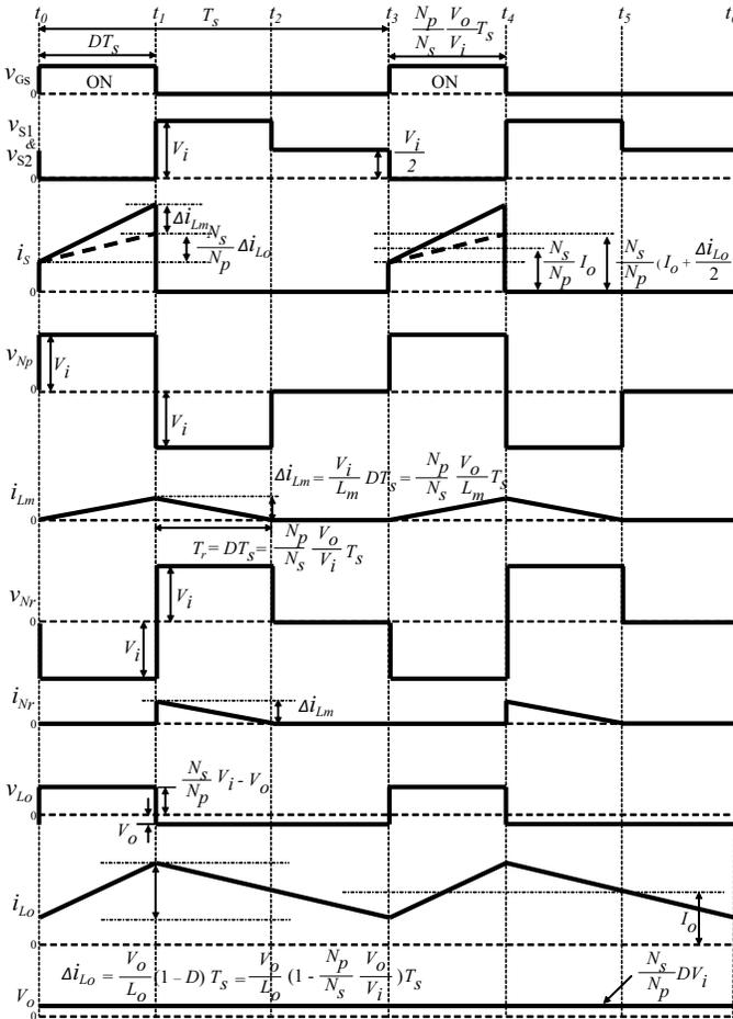
**Figure 3.13** Typical waveforms of a two-switch forward converter.
