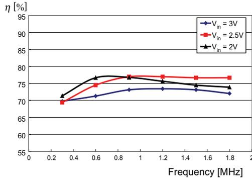
**Figure 8.13** Efficiency versus clock frequency.
