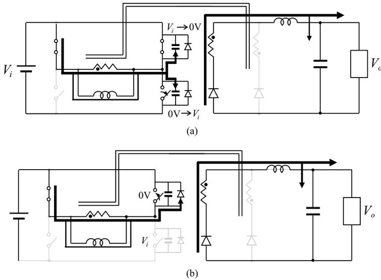
**Figure 3.31** Equivalent circuits for dead time with zero voltage switching (a) before reaching zero voltage and (b) after reaching zero voltage.
