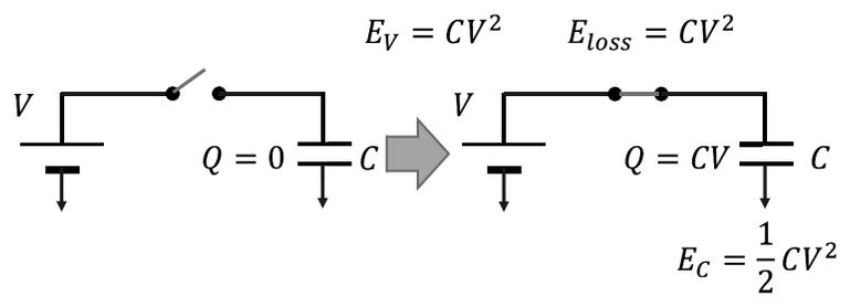
**Figure 1.5** A voltage source  $V$  can provide energy up to  $(1/2)CV^2$  into a capacitor  $C$ , and there power loss is essential in principle.
