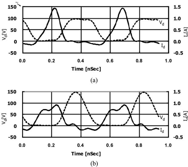
Figure 12.19 Simulated waveform of (a) class F and (b) inverse class F.
