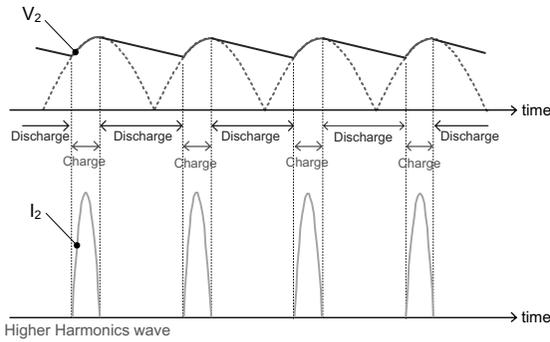
**Figure 6.42** Smoothing output voltage (without a PFC circuit).
