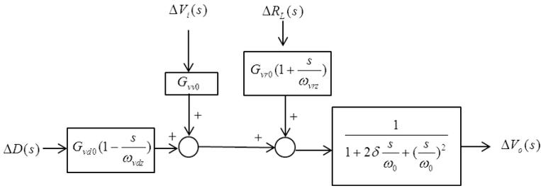
Figure 4.14 Small-signal model for CCM.
