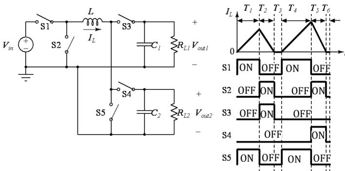
**Figure 9.16** Schematic of a SIMO converter using two positive buck-boost converters.
