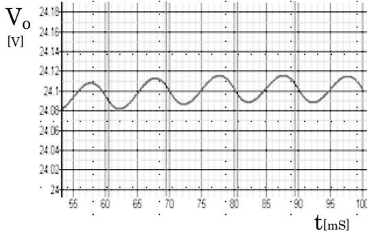
Figure 8.32 Output voltage ripple (100 Hz).
