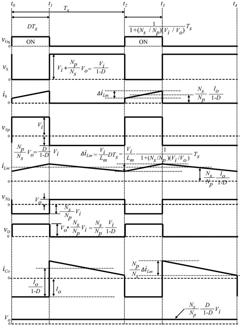
**Figure 3.4** Typical waveforms of a flyback converter.
