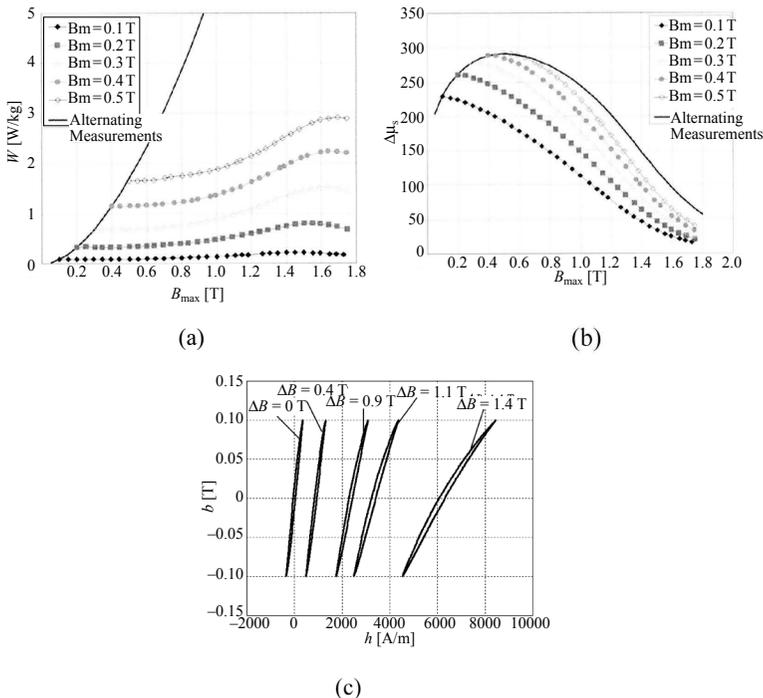
**Figure 6.6** DC bias characteristics of a nonoriented electromagnetic sheet. (a) Core loss characteristics. (b) Increment permeability characteristics. (c) Hysteresis loops with DC bias. Exciting frequency = 50 Hz.
