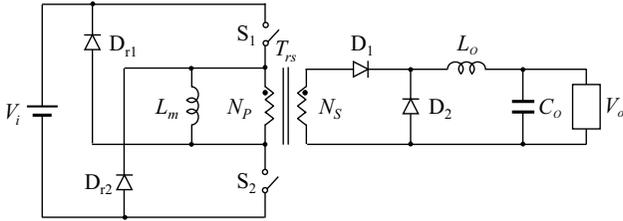
**Figure 3.11** Two-switch forward converter with the transformer-equivalent circuit.
