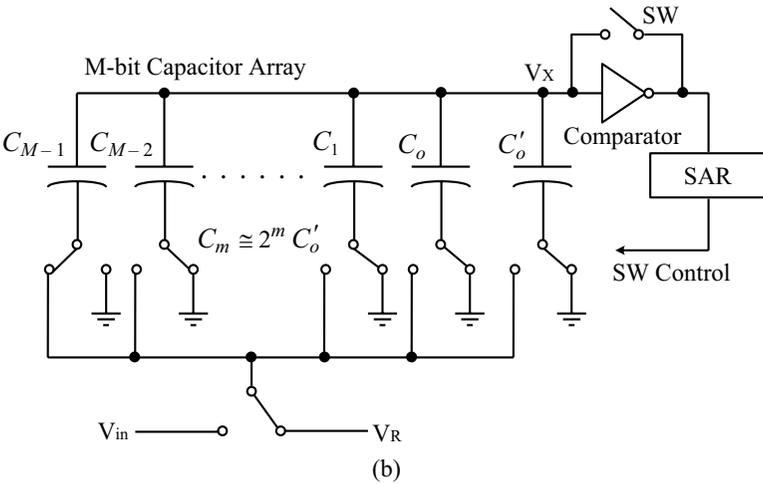
**Figure 13.13** Charge-distributed SAR ADC.
