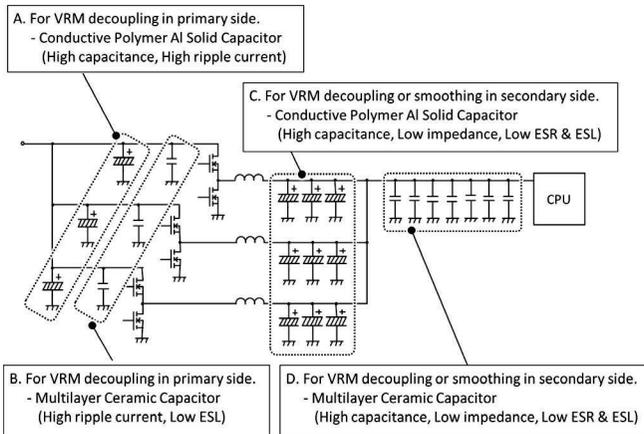
**Figure 6.31** VRM converter, ex.3phase VRM.
