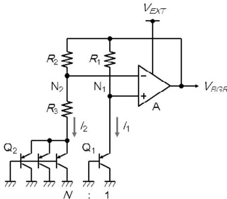
**Figure 7.10** Bandgap reference circuit using pnp bipolar transistors [22].
