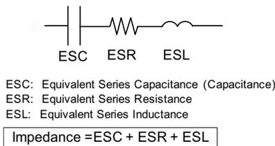
Figure 6.15 Equivalent circuit of a capacitor.
