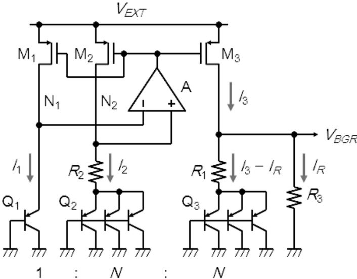
**Figure 7.14** Low-voltage bandgap reference circuit [24].
