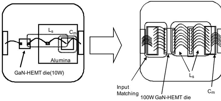
**Figure 12.13** High-power GaN die and class E circuit.
