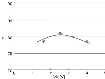
**Figure 8.12** Efficiency versus  $V_{in}$  (experiment).
