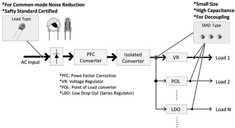
**Figure 6.27** Usage of ceramic capacitors in a power distribution network.
