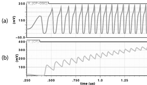
**Figure 10.12**  $V_{CP}$  start-up.
