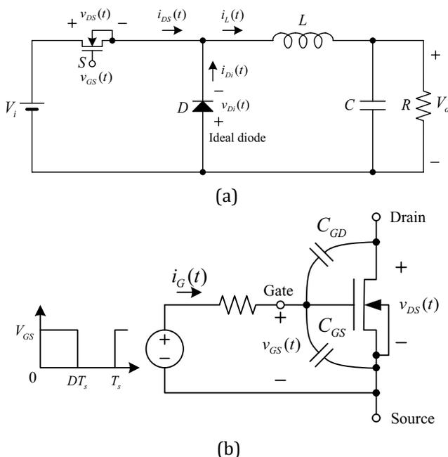
**Figure 1.26** Buck converter circuit having a MOSFET and an ideal diode as switching devices. (a) Buck converter circuit and (b) capacitances in the MOSFET and a waveform driving its gate.
