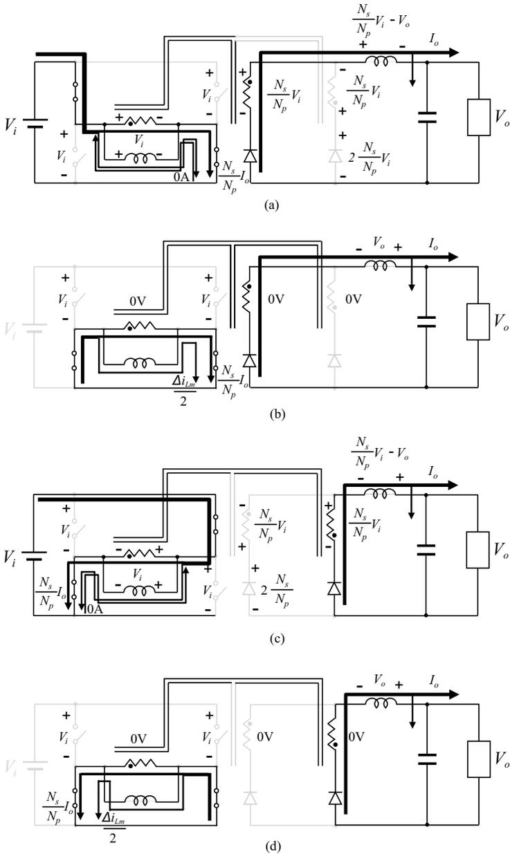
**Figure 3.24** Equivalent circuits for each operation state with PWM control. (a)  $t_0 - t_1$ , (b)  $t_1 - t_2$ , (c)  $t_2 - t_3$ , and (d)  $t_3 - t_4$ .
