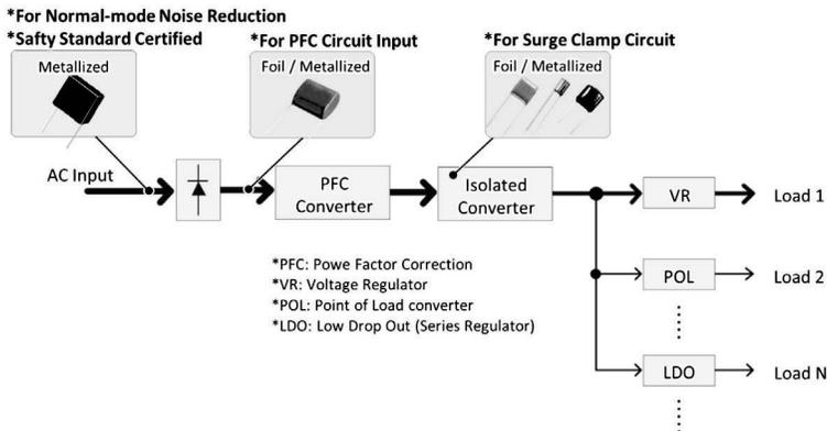
**Figure 6.23** Usage of film capacitors in a power distribution network.
