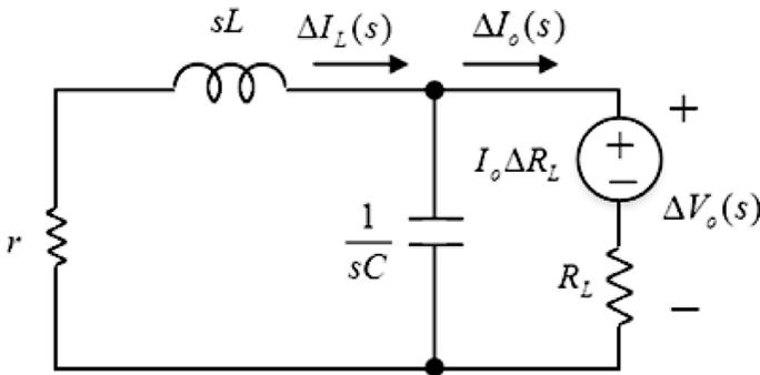
**Figure 4.8** Equivalent circuit for load resistance change.
