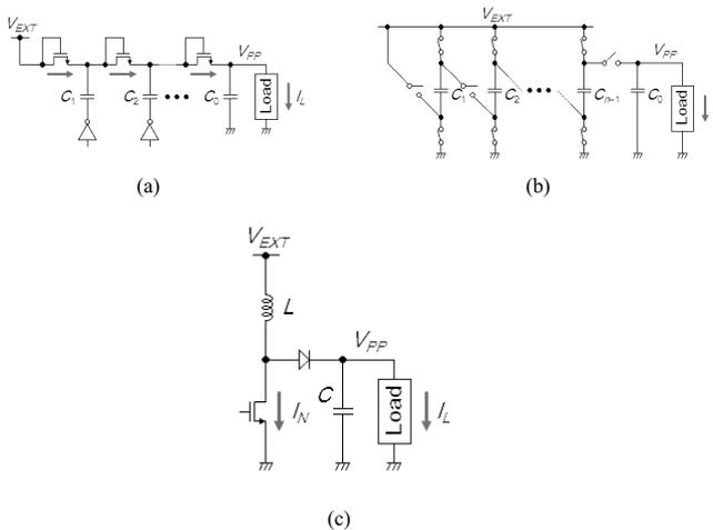
**Figure 7.24** (a) Voltage up-converters; charge pump. (b) Switched capacitor. (c) Switching (boost) converter.
