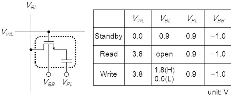
**Figure 7.5** Example of voltages used for DRAM.
