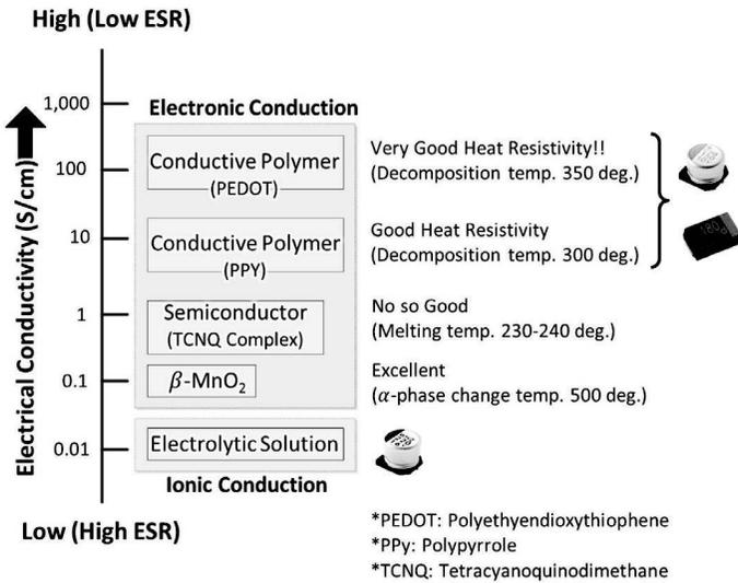
Figure 6.14 Electrical conductivity of an electrolyte (aluminum electrolytic capacitor).
