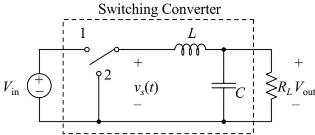
Figure 9.2 Schematic of a buck converter.
