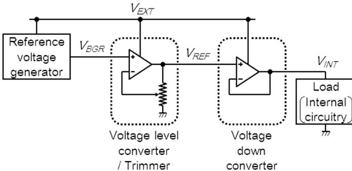
**Figure 7.6** Schematic of an on-chip voltage down-converter.
