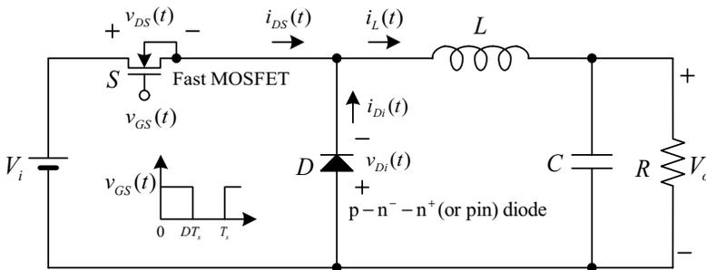
**Figure 1.28** Buck converter circuit having a MOSFET and a p-n<sup>-</sup>-n<sup>+</sup> (or pin) diode.
