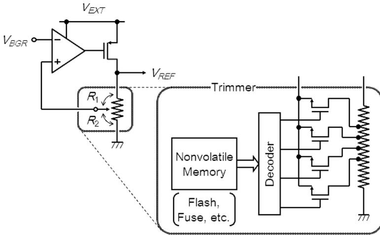
**Figure 7.17** Voltage converter/trimmer circuit.
