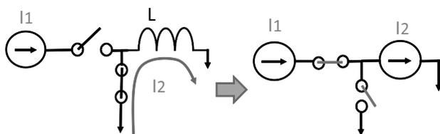
**Figure 1.11** A current source and an inductor do not have a good relationship.
