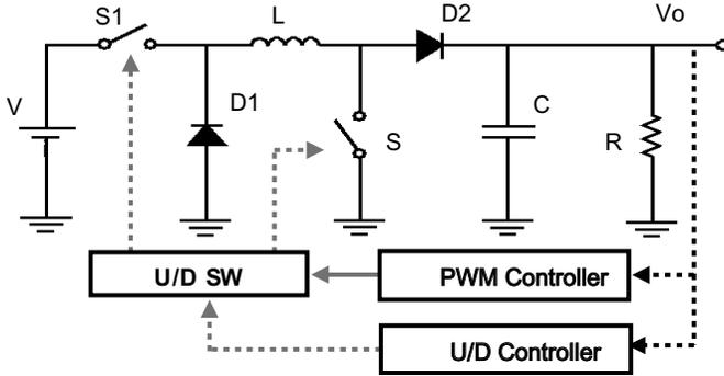
Figure 8.2 Buck–boost converter with U/D controller.
