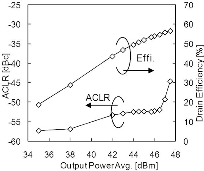
**Figure 12.38** Efficiency and ACLR of a Doherty amplifier.  $V_{ds} = 50$  V,  $I_{ds-main} = 400$  mA ( $V_{gs} = -1.24$  V),  $I_{ds-peak} = 0$  mA ( $V_{gs} = -3$  V),  $F = 2.14$  GHz W-CDMA 2-carrier, 5 MHz spacing PAPR = 7.8 dB with a DPD evaluation test system.
