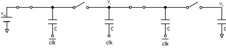
**Figure 13.17** An ideal three-stage Dickson charge pump circuit.
