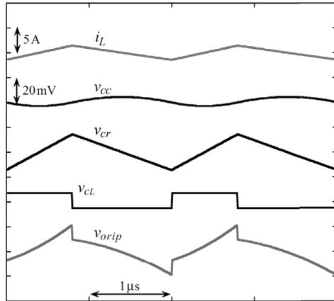
**Figure 2.11** Waveforms of ripple current and voltages.  $V_i = 12 \text{ V}$ ,  $D = 0.4$ ,  $L = 2 \mu\text{H}$ ,  $C = 100 \mu\text{F}$ ,  $r_c = 10 \text{ m}\Omega$ , and  $L_c = 2 \text{ nH}$ .
