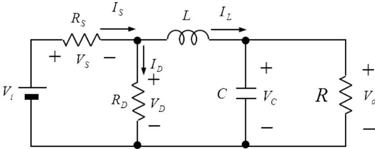
**Figure 4.12** The equivalent device model for discontinuous conduction mode.
