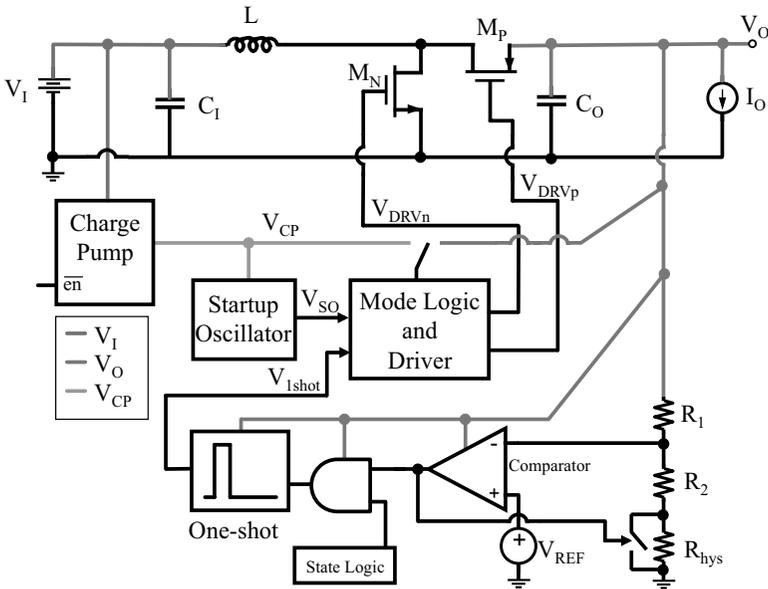
**Figure 10.2** Bootstrapped boost converter block diagram.
