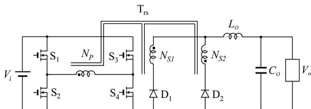
**Figure 3.22** Ideal pulse width modulation (PWM)-controlled full-bridge converter circuit.
