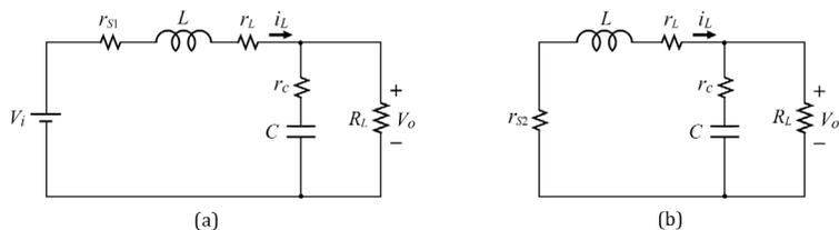
**Figure 2.7** Equivalent circuit of a buck converter. (a) On state and (b) Off state.
