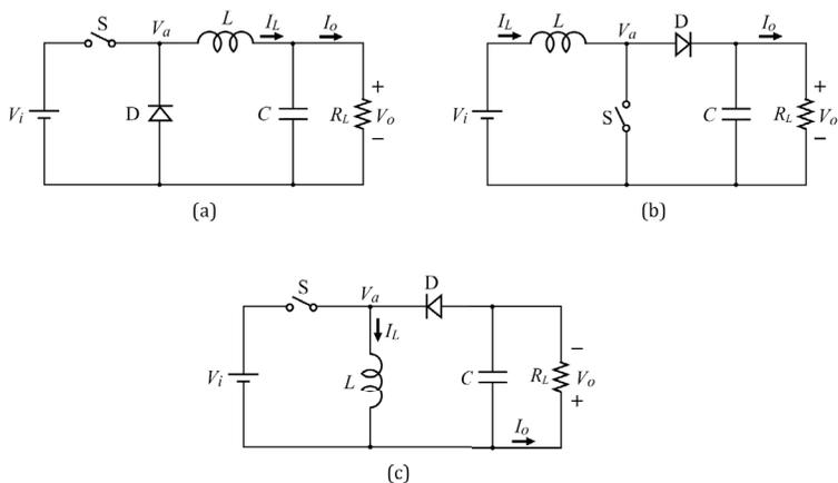
**Figure 2.1** Three typical DC-to-DC converters. (a) A buck converter, (b) a boost converter, and (c) a buck-boost converter.
