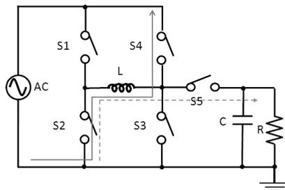
**Figure 8.17** H bridge AC–DC converter (current when  $V_{in} > 0$ ).
