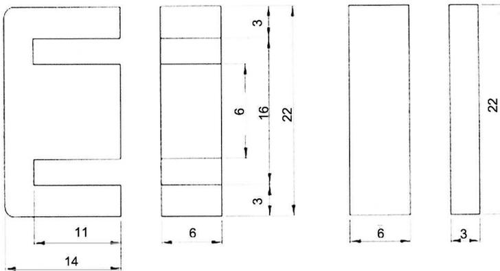
**Figure 6.7** Core dimensions of the inductor (unit is mm).
