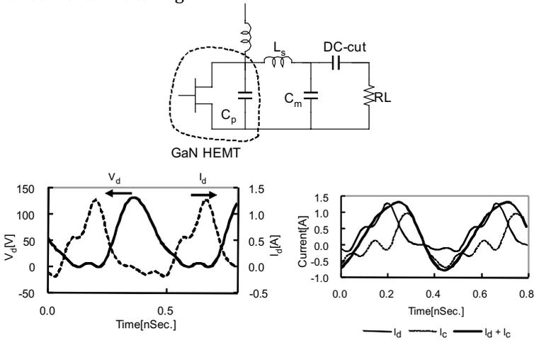
Figure 12.10 Low-pass-type class E circuit and waveform.
