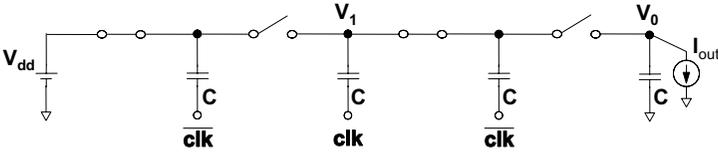
**Figure 13.20** A non-ideal three-stage Dickson charge pump circuit where the output load current  $I_{\text{out}}$  is considered.
