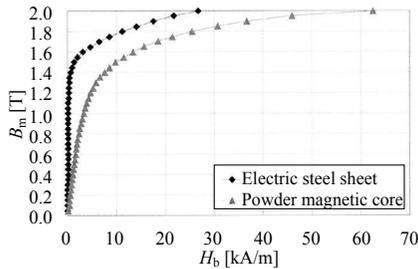
**Figure 6.4** Magnetization characteristics of various magnetic materials (electrical steel sheet and powder magnetic core). Exciting frequency = 50 Hz.
