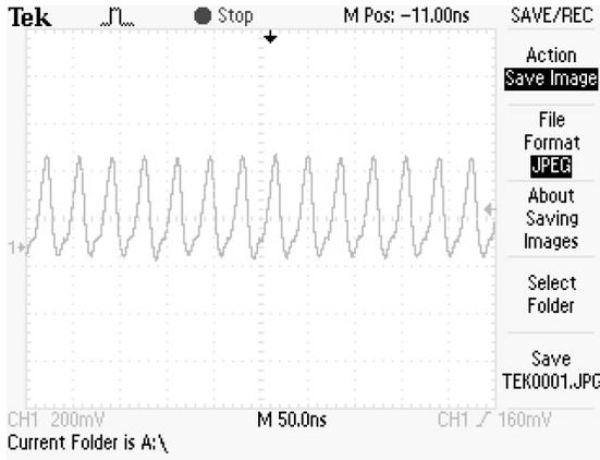
Figure 10.20 Charge pump oscillator buffer output at 400 mV.
