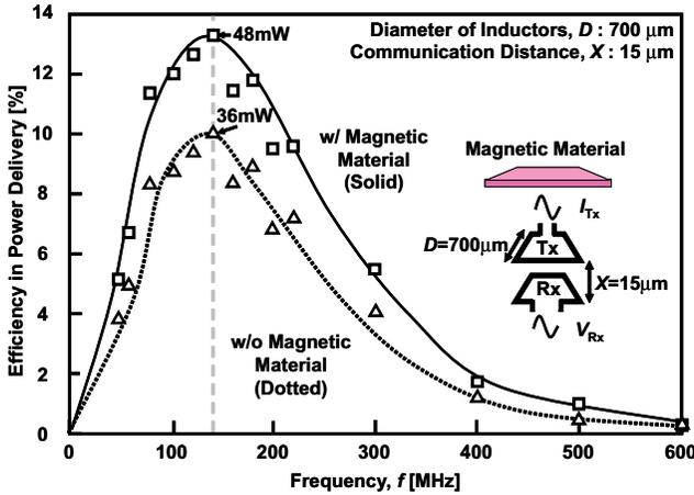
**Figure 11.6** Measured efficiency dependence on operational frequency. Copyright (2009), The Japan Society of Applied Physics.
