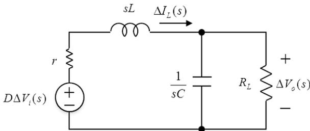
Figure 4.7 Equivalent circuit for an input voltage change.
