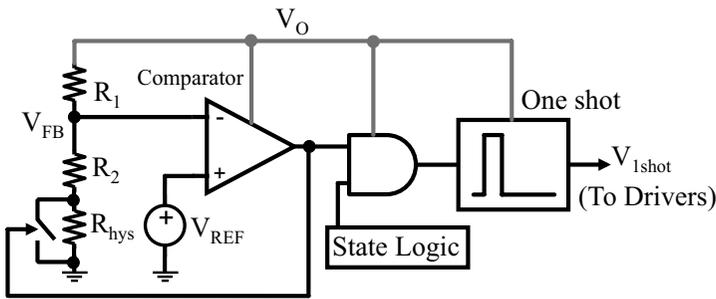
**Figure 10.8** Hysteretic control schematic.
