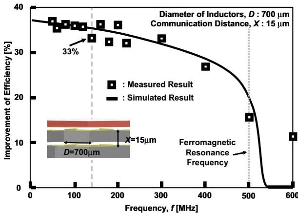
**Figure 11.7** Measured improvement of efficiency dependence on operational frequency. Copyright (2009), The Japan Society of Applied Physics.
