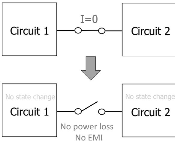
**Figure 1.19** Switch turns off when  $I = 0$  (ZCS).
