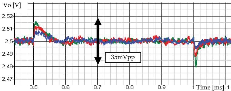
**Figure 8.6** Improvement of output voltage ripple.
