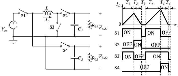
**Figure 9.15** Schematic of a SIMO converter using boost and negative buck-boost converters.
