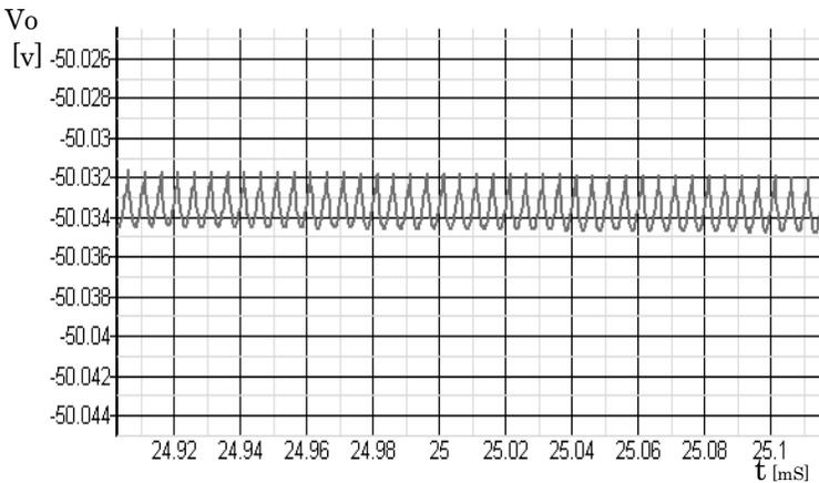
**Figure 8.27** Output ripple of the converter.
