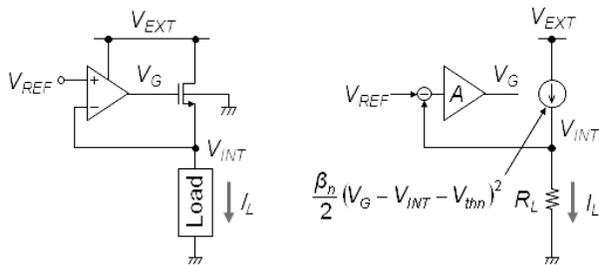
**Figure 7.22** An nMOSFET output series regulator (a) and its large-signal equivalent circuit (b).
