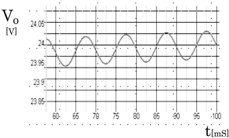
**Figure 8.39** Output voltage ripple.
