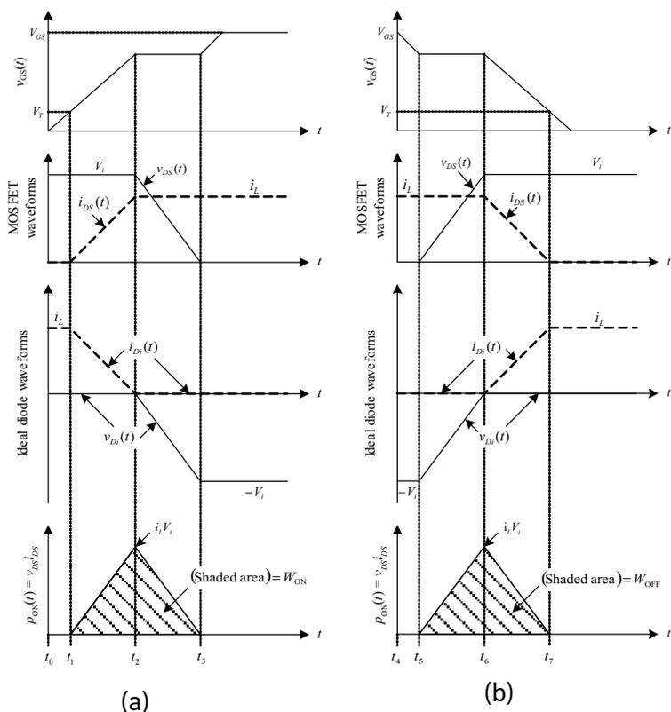
**Figure 1.27** (a) Turn-on and (b) turn-off transition piecewise-linear waveforms of the MOSFET and diode for the buck converter circuit in Fig. 1.26.
