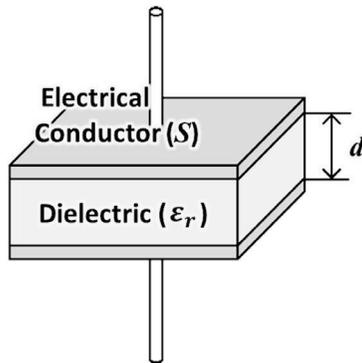
**Figure 6.10** Basic model of a capacitor.
