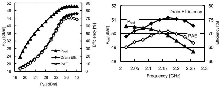
**Figure 12.14** Power and frequency characteristics of 100 W class E GaN HEMT.
