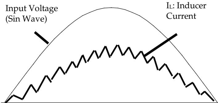
Figure 8.36 Waveform of the inductor current in CCM.
