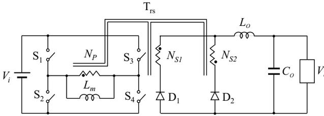
**Figure 3.23** PWM-controlled full-bridge converter with the transformer-equivalent circuit.
