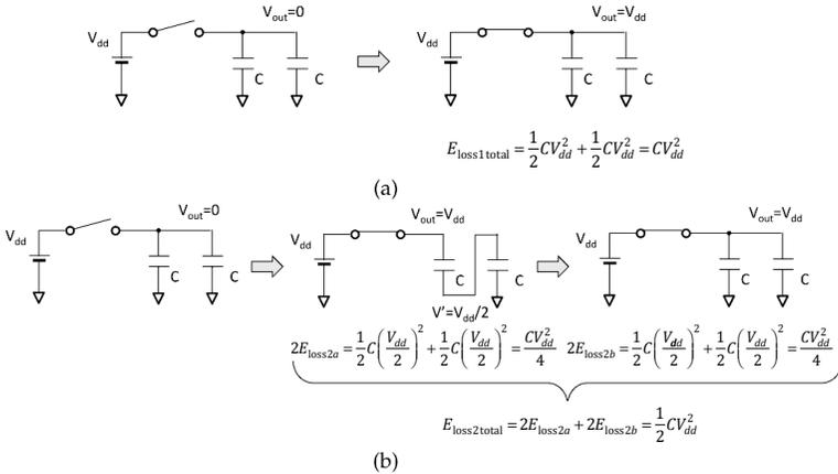
Figure 13.9 Charging two capacitors to  $CV_{\text{dd}}$ . (a) Method 1. (b) Method 2.
