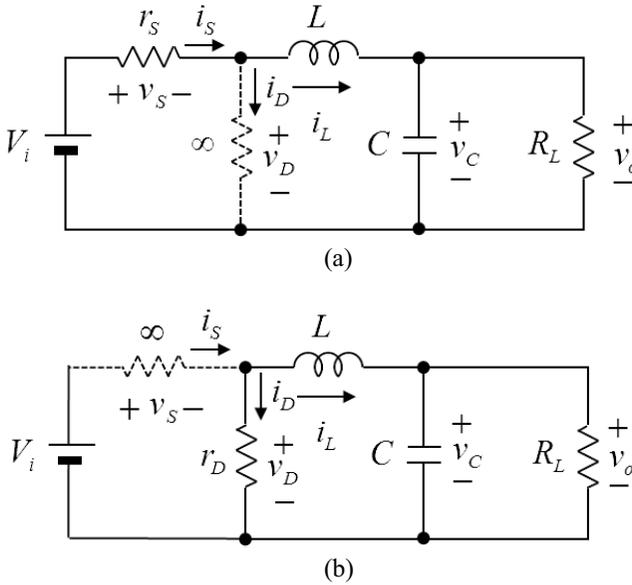
**Figure 4.3** Equivalent circuits in continuous conduction mode. (a) State I and (b) state II.
