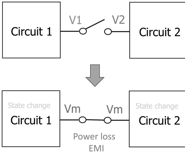
Figure 1.16 Switch turns on when  $V_1 \neq V_2$ .
