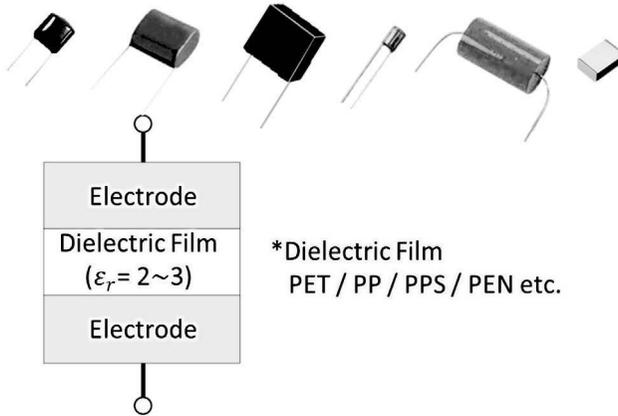
**Figure 6.21** Basic model of a film capacitor (nonpolarity).
