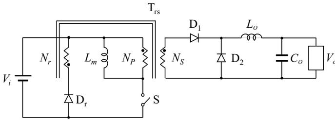
**Figure 3.7** Single-switch forward converter with the transformer-equivalent circuit.
