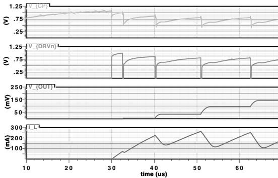
Figure 10.13  $V_{CP}$  driving switch transistors.
