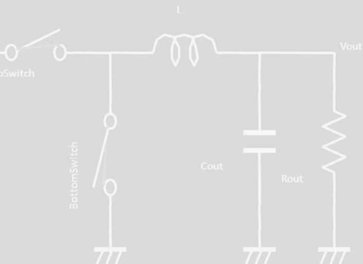
$$\begin{aligned} V_{out} &= \frac{T_{on}}{T_{on} + T_{off}} V_{in} \\ &= \frac{T_{on}}{T} V_{in} \end{aligned}$$
