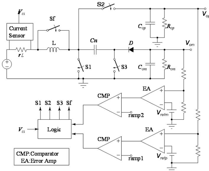
Figure 9.22 Schematic of the voltage-mode control of Fig. 9.21.
