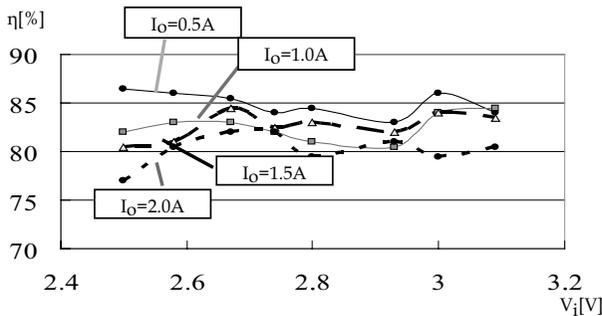
Figure 8.9 Efficiency versus input voltage.
