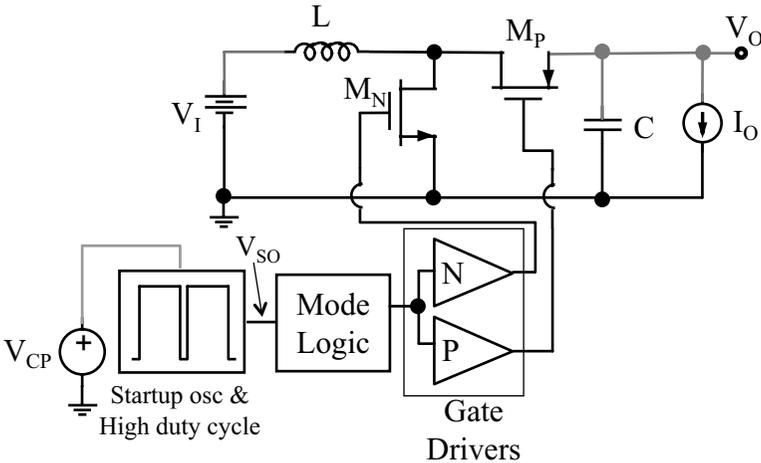
**Figure 10.6** Start-up circuitry connected to drivers and output switches.
