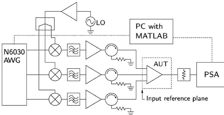
**Figure 12.39** Example of an  $N$ -way Doherty with a mixed-signal approach.
