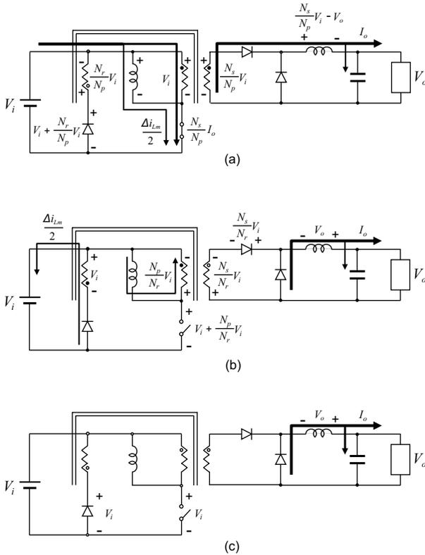
**Figure 3.8** Equivalent circuit for each operation state. (a)  $t_0 - t_1$ , (b)  $t_1 - t_2$ , and (c)  $t_1 - t_3$ .
