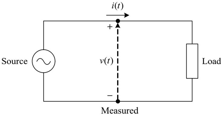
**Figure 1.24** Measurement of energy transmission in a power supply system.
