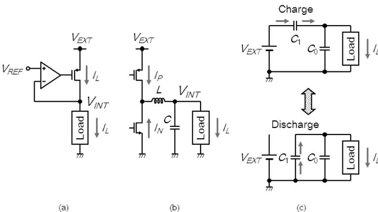
**Figure 7.18** Voltage down-converters.
