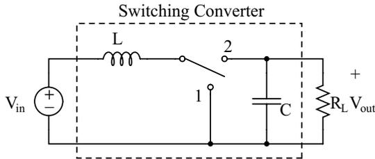
**Figure 9.4** Schematic of a boost converter.
