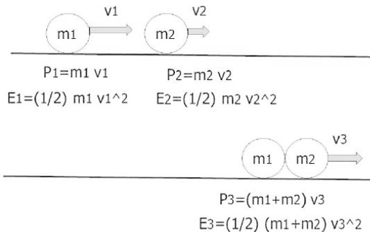
**Figure 13.10** Collision of two masses.
