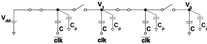
**Figure 13.19** A non-ideal three-stage Dickson charge pump circuit where the parasitic capacitance  $C_p$  of each node is considered.
