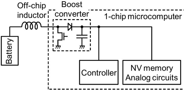
Figure 7.3 Microcomputer with an on-chip DC-DC boost converter [19].
