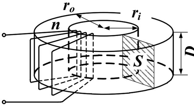
**Figure 6.1** Ring-shaped core.
