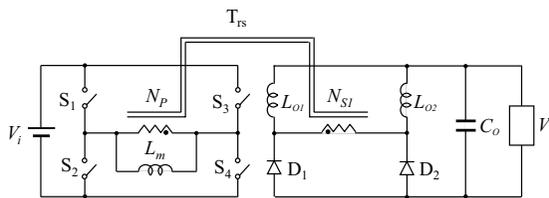
**Figure 3.28** Equivalent circuit of a full-bridge converter with a current-doubler circuit.
