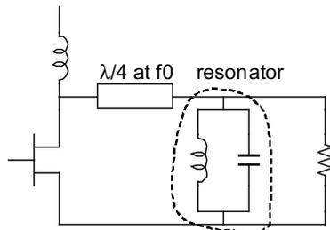
**Figure 12.16** Typical circuit and waveforms of class F.
