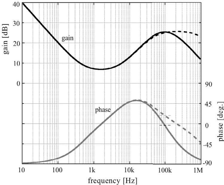
**Figure 2.17** Comparison of frequency responses of the error amplifier for ideal and actual operational amplifiers. Dashed lines are the ideal case, and solid lines are the actual case with a 5 MHz GBW.
