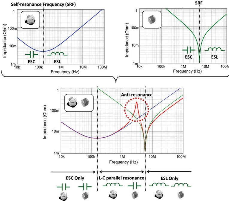
**Figure 6.29** Output antiresonance.
