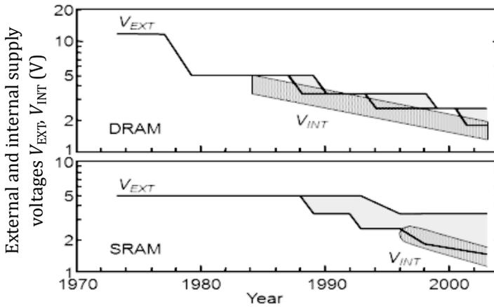
**Figure 7.1** Trends in external and internal supply voltages of memory LSIs, dynamic RAMs (DRAMs, top), and static RAMs (SRAMs, bottom) [1].
