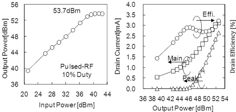
**Figure 12.37** Power characteristics of a Doherty amplifier.
