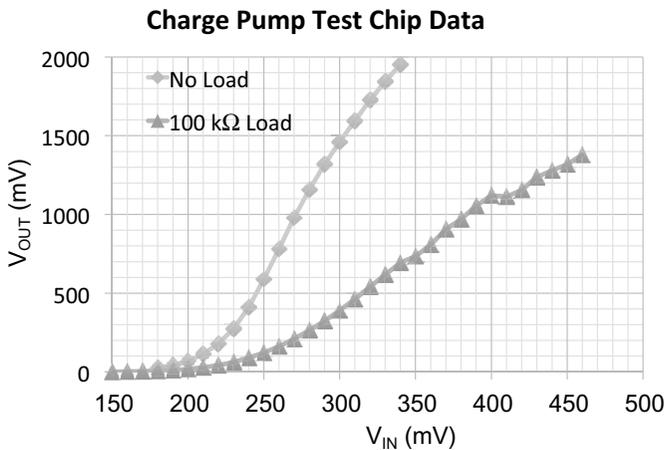
Figure 10.21 Test chip transfer function with and without a load.
