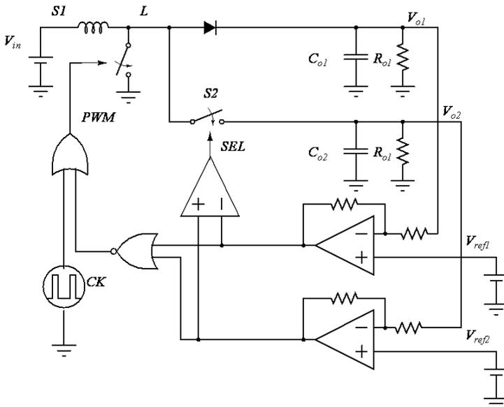
**Figure 9.25** Schematic of a SIMO boost-boost converter using hysteresis control.
