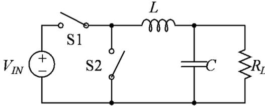
Figure 9.7 Schematic of a buck converter using an ideal switch.
