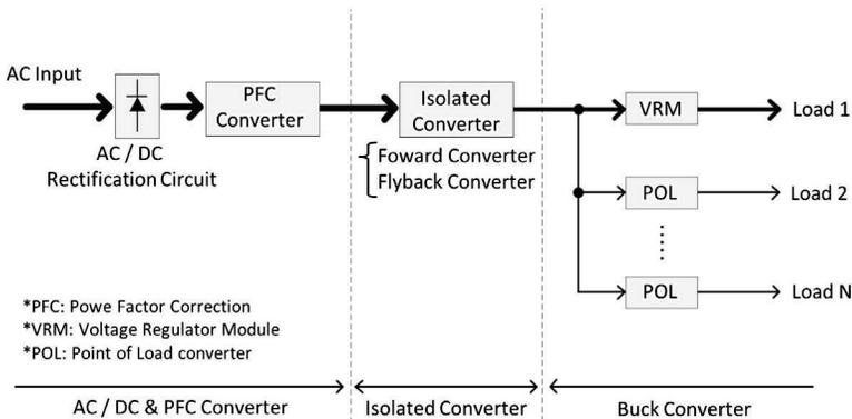
**Figure 6.30** Distributed power generation system (three stages).
