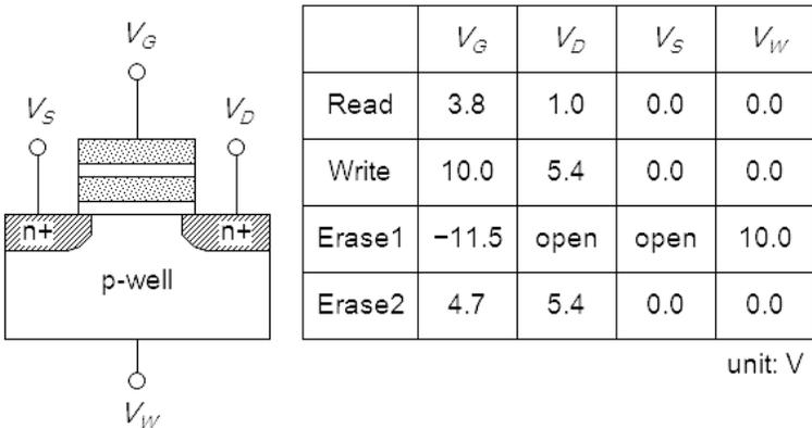
Figure 7.4 Example of voltages used for flash memory.
