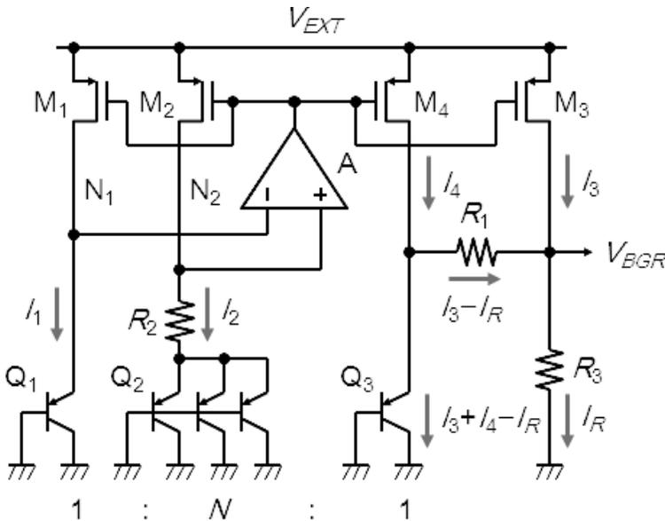
**Figure 7.16** Low-voltage bandgap reference circuit [26].
