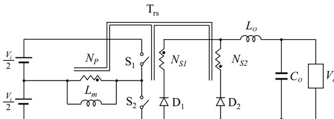
**Figure 3.19** Half-bridge converter with the transformer-equivalent circuit.
