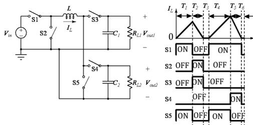
**Figure 9.12** Schematic of a SIMO converter using buck and positive buck–boost converters.
