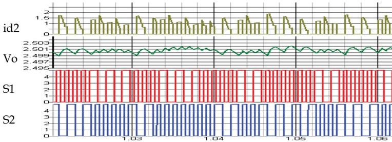
**Figure 8.5** Waveform of a dual  $\Delta\Sigma$  converter.
