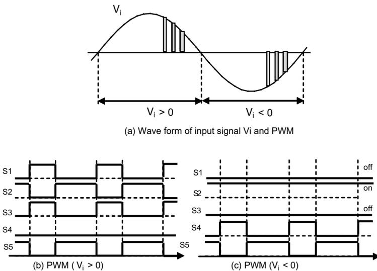
**Figure 8.18** Timing chart of control signals for switches. (a) Waveform of input signal  $V_i$  and PWM. (b) PWM ( $V_i > 0$ ). (c) PWM ( $V_i < 0$ ).
