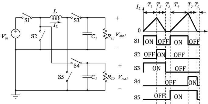
**Figure 9.14** Schematic of a SIMO converter using buck and negative buck-boost converters.
