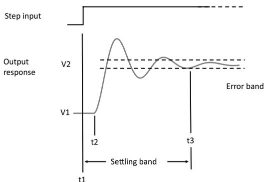
**Figure 1.12** An inductor can cause overshoot or ringing for step response.
