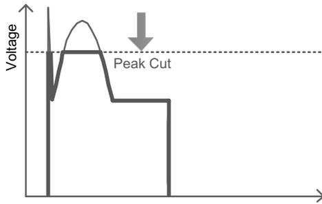
**Figure 6.37** Surge clamp circuit waveform.
