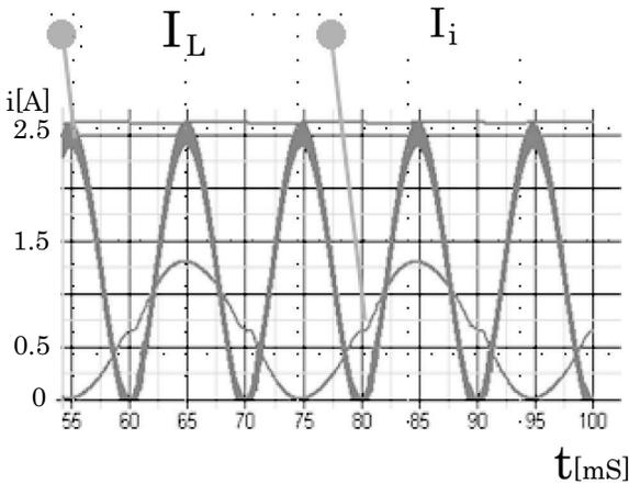
Figure 8.38  $I_i$  and inductor current.
