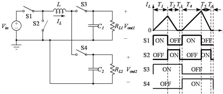
**Figure 9.9** Schematic of a basic SIMO converter using two buck converters.
