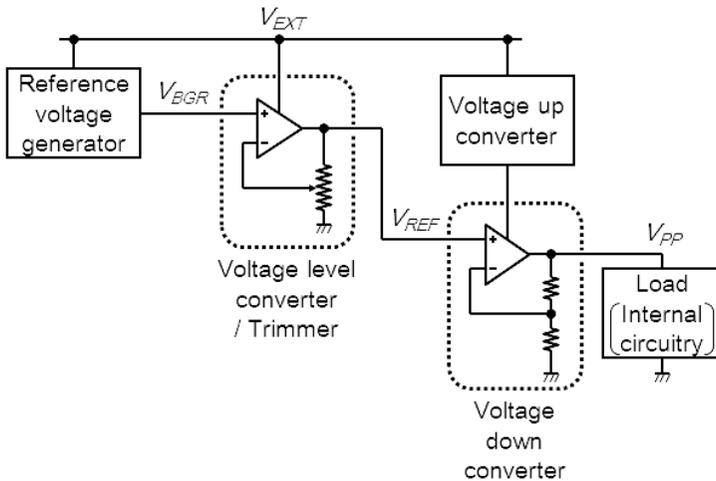
**Figure 7.8** Schematic of an on-chip voltage down-converter.
