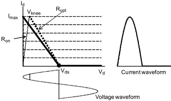
**Figure 12.2** Load resistance and waveform at class B.
