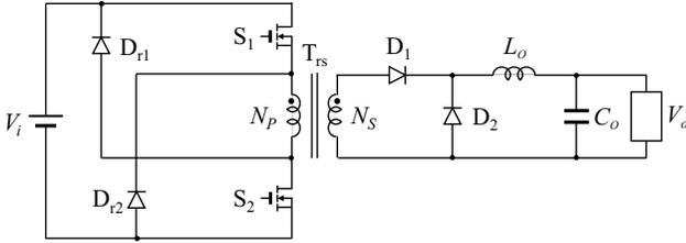
**Figure 3.10** Ideal two-switch forward converter.
