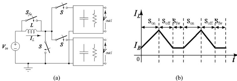
**Figure 9.20** Waveform of inductor current using PCCM. (a) SIMO circuit with a freewheel switch. (b) Waveform of inductor current using PCCM.
