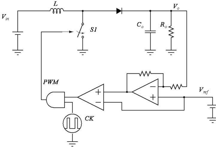
**Figure 9.24** Schematic of a boost converter using hysteresis control.
