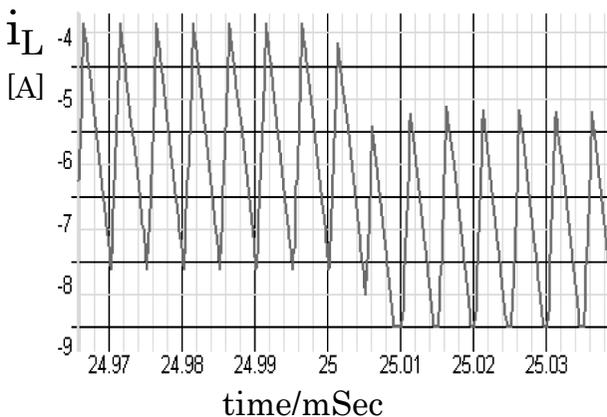
**Figure 8.23** Waveform of inductor current.
