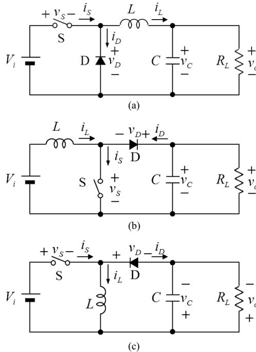
**Figure 4.13** Basic converters: (a) Buck, (b) boost, and (c) buck–boost.
