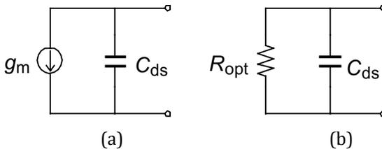
**Figure 12.3** Simplified equivalent circuit at the drain side (a) and  $Z_{\text{opt}}^*$  (b).
