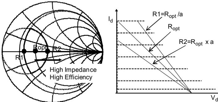
**Figure 12.29** Contours for power and load lines.
