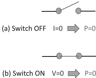
**Figure 1.13** Power loss of an ideal switch is zero.
