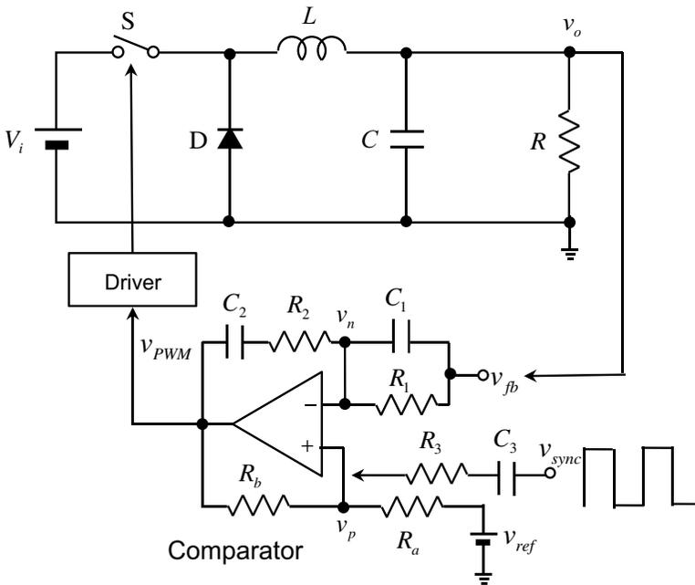
**Figure 5.5** Constant-frequency hysteretic PWM generator.
