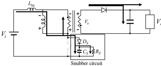
**Figure 3.5** Flyback converter with an RCD snubber circuit.
