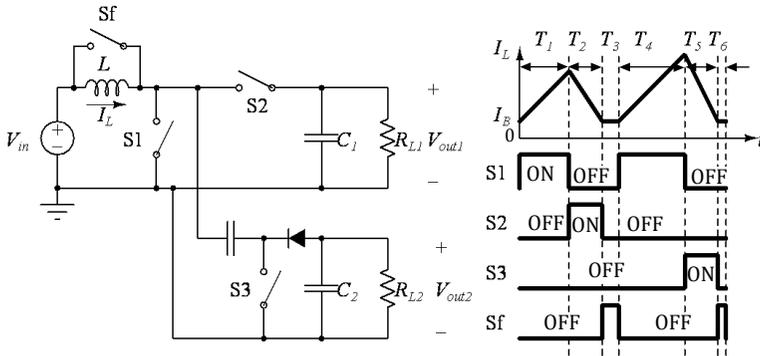
**Figure 9.21** Schematic of a SIMO converter using a boost converter and a charge pump circuit.
