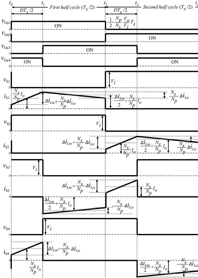
**Figure 3.27** Typical waveforms of a phase-shift controlled full-bridge converter.
