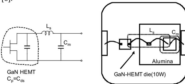
Figure 12.11 Designed class E amplifier.
