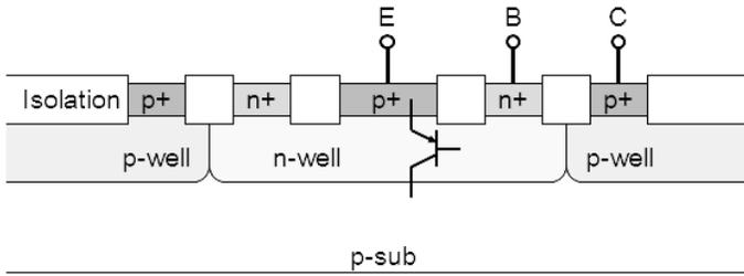
**Figure 7.11** Cross section of a parasitic pnp bipolar transistor.
