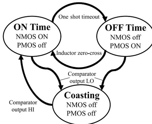
**Figure 10.9** Hysteretic control state diagram.
