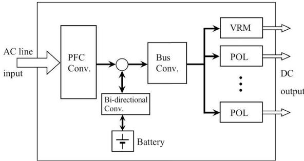
**Figure 2.4** Schematic of the power supply in a computer system.
