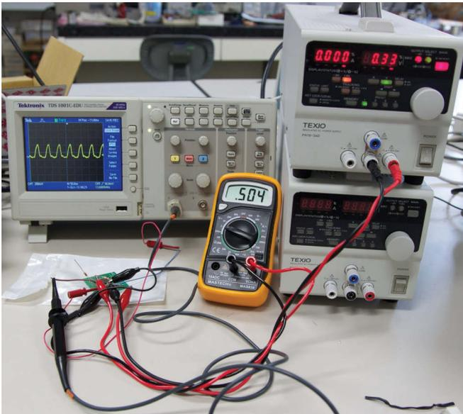
Figure 10.19 Charge pump lab setup.
