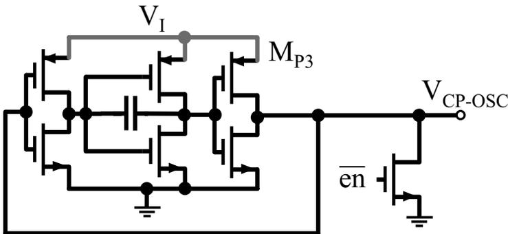
**Figure 10.3** Start-up charge pump oscillator.
