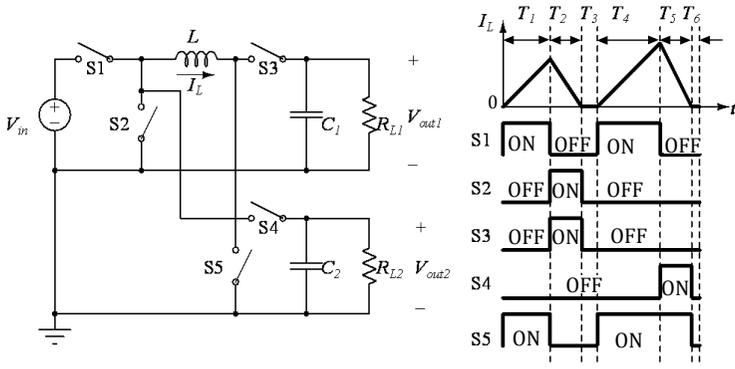
**Figure 9.18** Schematic of a SIMO converter using positive and negative buck-boost converters.
