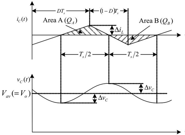
**Figure 1.22** Steady-state capacitor voltage and current waveforms in the buck converter.
