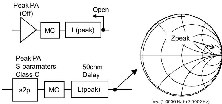
**Figure 12.33** Design of the peak amplifier.
