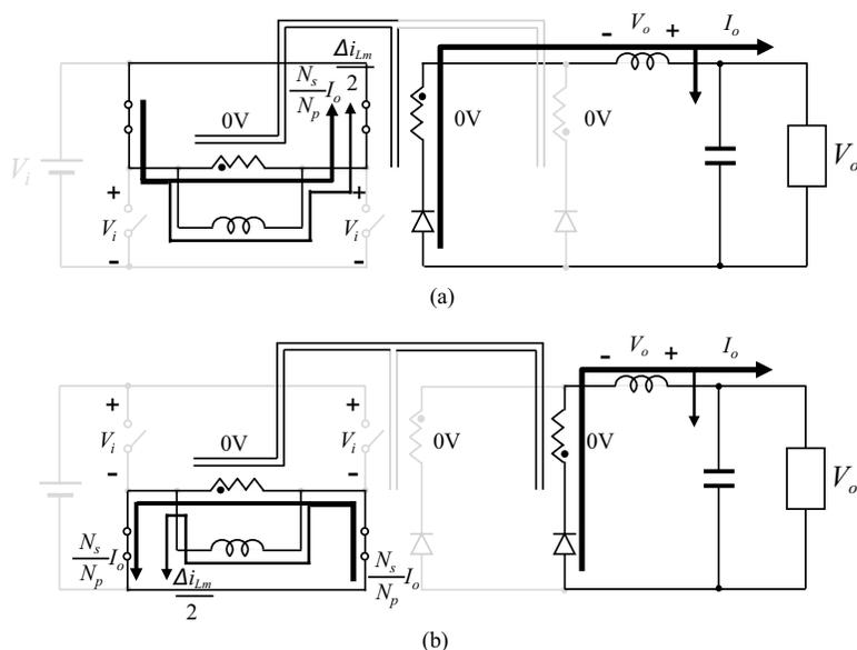
**Figure 3.26** Equivalent circuits for each operation state with phase-shift control. (a)  $t_1 - t_2$  and (b)  $t_3 - t_4$ .
