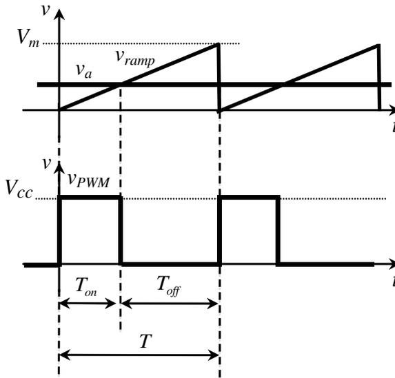
**Figure 5.2** Operating waveforms of a comparator.
