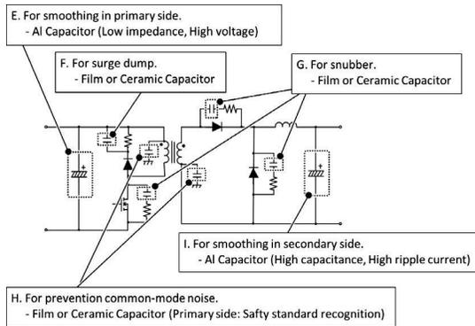
**Figure 6.35** Forward converter.
