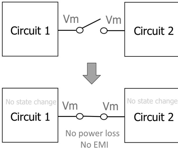
**Figure 1.17** Switch turns on when  $V_1 = V_2$  (ZVS).
