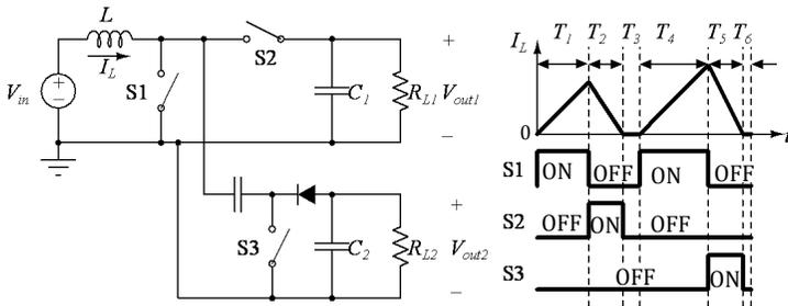
**Figure 9.19** Schematic of a SIMO converter using a boost converter and a charge pump circuit.
