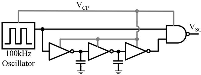
**Figure 10.5** Start-up oscillator and high-duty-cycle circuitry.
