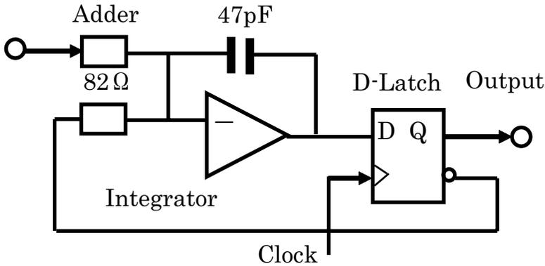
**Figure 8.10** Circuit of a  $\Delta\Sigma$  modulator.
