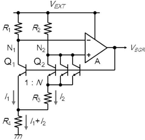
**Figure 7.12** Bandgap reference circuit using npn bipolar transistors [23].
