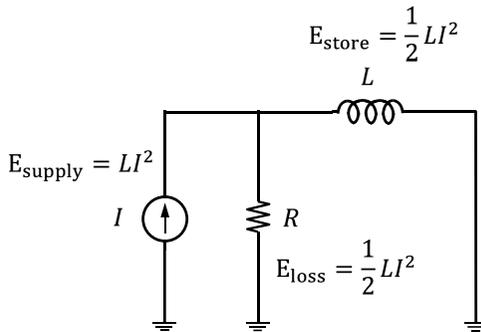
**Figure 1.7** A current source  $I$  can provide energy up to  $(1/2)LI^2$  into an inductor  $L$ , and there power loss is essential in principle.
