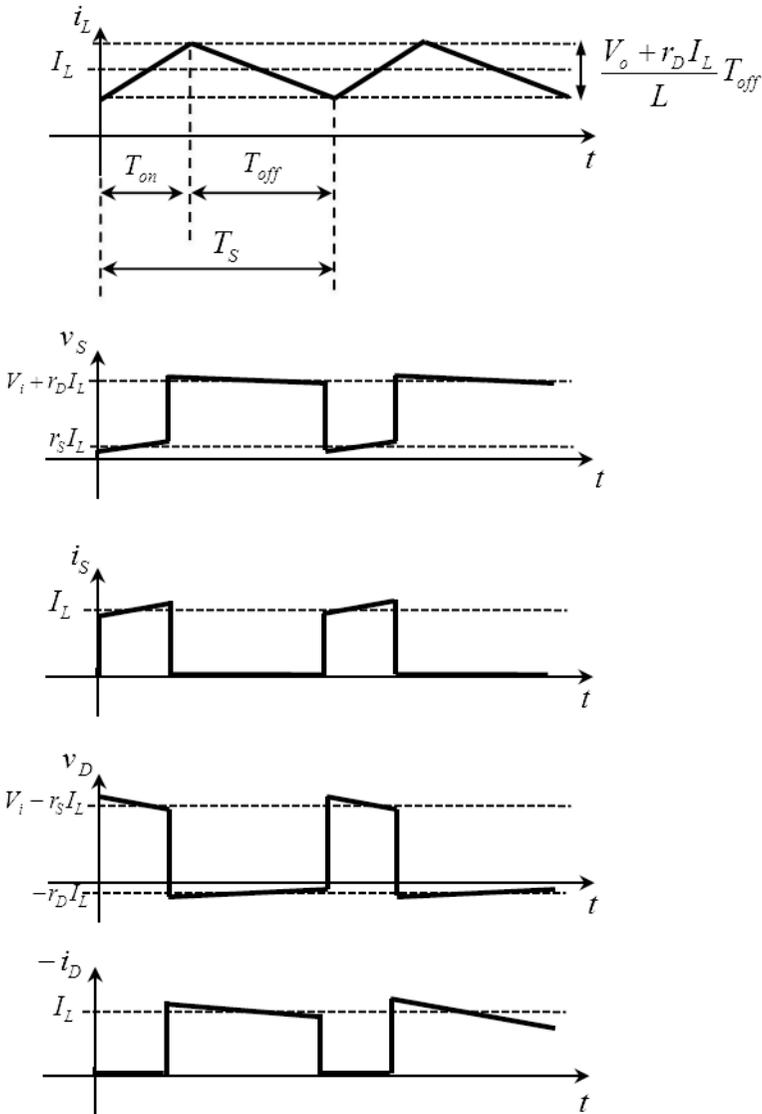
**Figure 4.4** Key waveforms of the currents and voltages in CCM.
