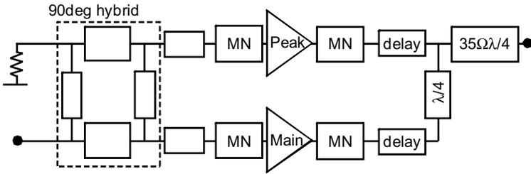
**Figure 12.34** Total design of a Doherty amplifier.
