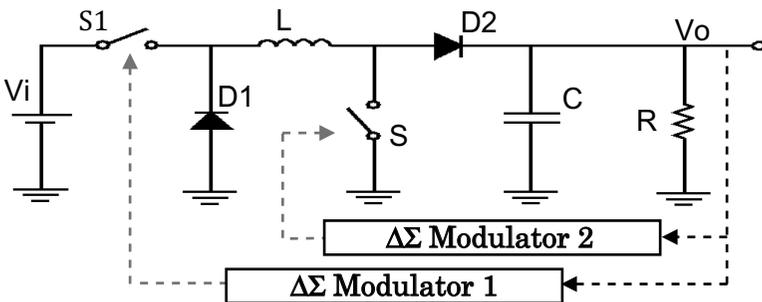
Figure 8.3 Buck–boost converter with dual  $\Delta\Sigma$  modulators.
