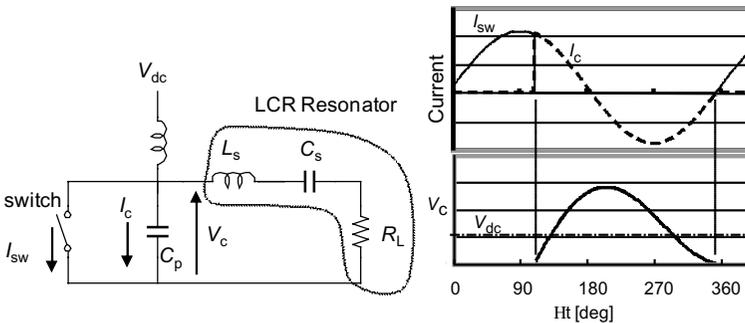
**Figure 12.7** Common class E circuit and current and voltage waveforms.
