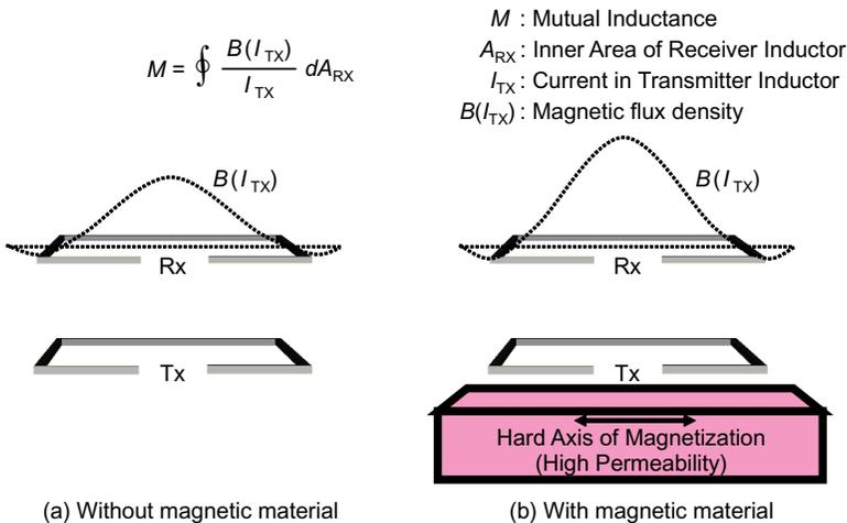
**Figure 11.4** Improvement of efficiency using thin-film magnetic material (a) without magnetic material and (b) with magnetic material. Copyright (2009), The Japan Society of Applied Physics.
