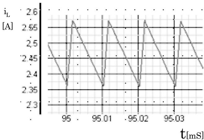
**Figure 8.40** Inductor current in CCM.
