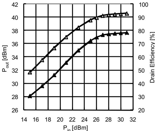
**Figure 12.22** Power characteristics of a 10 W class F.
