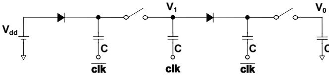
**Figure 13.18** A non-ideal three-stage Dickson charge pump circuit where the voltage drop  $V_d$  across each switch is considered.
