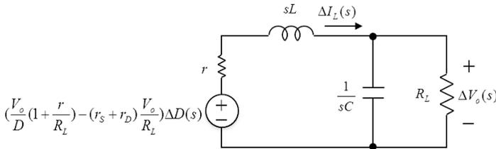
**Figure 4.6** Equivalent circuit for a duty cycle change.
