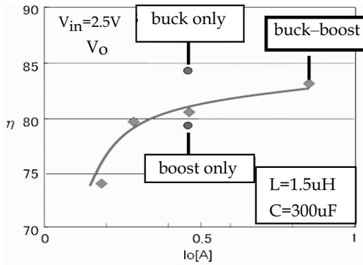
**Figure 8.11** Efficiency versus  $I_o$  (experiment).
