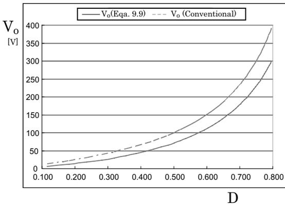
Figure 8.24 Average  $D$  versus  $V_o$  ( $V_{rms} = 100$  V).
