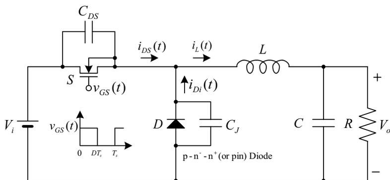
**Figure 1.30** Drain–source capacitance of the MOSFET and p-n junction capacitance of the pin diode in a buck converter circuit: the energy stored in the capacitances is dissipated by the MOSFET during the turn-on transition.
