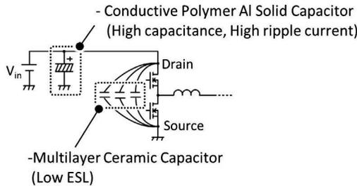
**Figure 6.33** Layout position of MLCCs for input.
