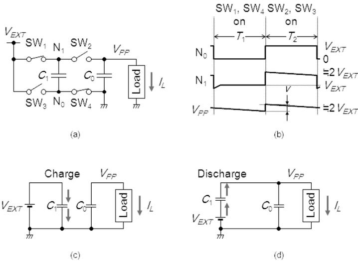
**Figure 7.26** Principle of voltage doubling; circuit diagram (a), operating waveforms (b), equivalent circuit during  $T_1$  (c), and equivalent circuit during  $T_2$  (d).
