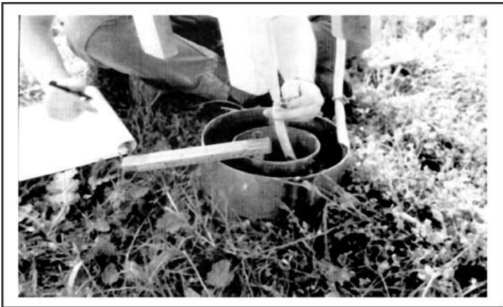
Fig. 2.10 Ring infiltrometer for measuring the infiltration capacity
