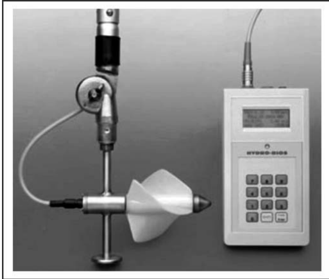
Fig. 2.19 Rodheld portable current meter manufactured by Hydro-Bios Intern. Ltd. Co.
