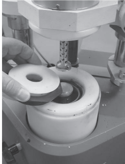
FIGURE A.54 Water bath for controlling specimen temperature during testing.
