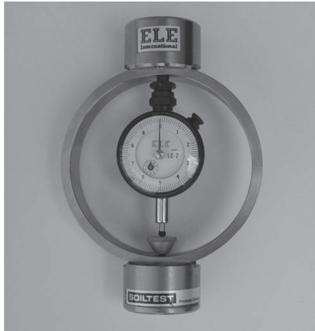
FIGURE 1.34 Proving ring. (Courtesy of Humboldt Mfg. Co.)
