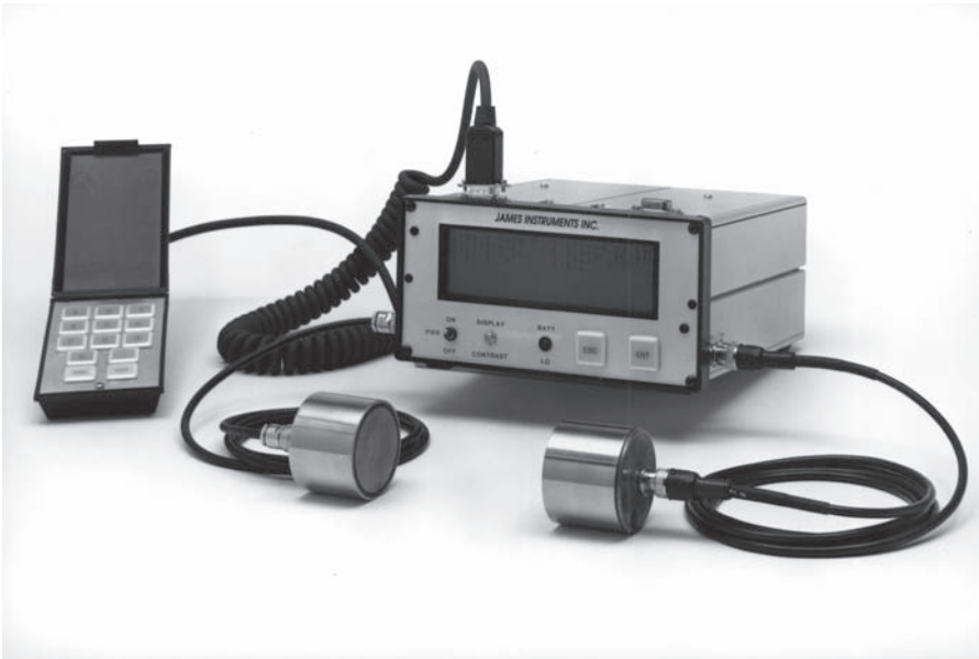
FIGURE 7.41 Ultrasonic pulse velocity apparatus. (Courtesy of James Instruments Inc.)
