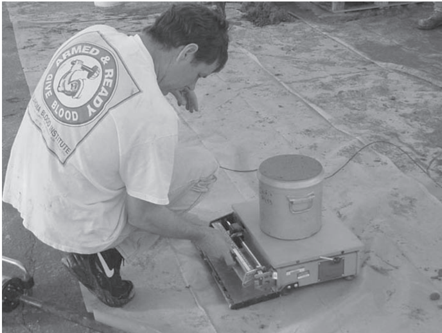
FIGURE A.33 Weighing concrete inside the container.
