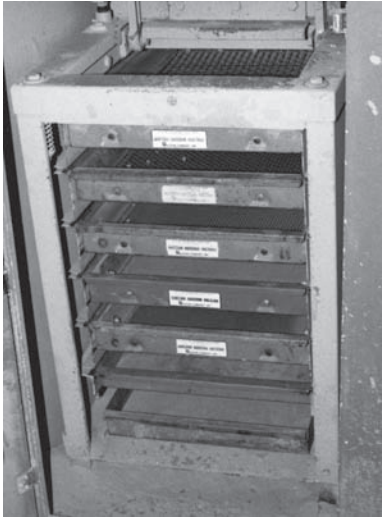
FIGURE 5.12 Sieve shaker for large samples of aggregates.
