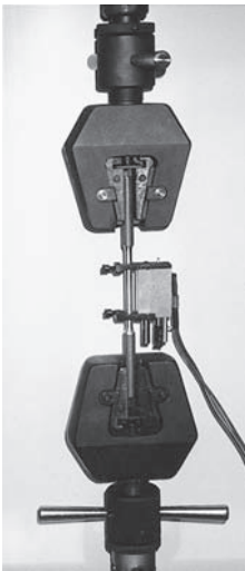
FIGURE 3.16 Tension test on a round steel specimen showing grips and an extensometer with an LVDT.
