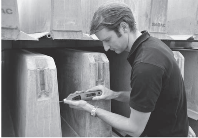
FIGURE A.47 Testing concrete with a rebound hammer. (Courtesy of Proceq)
