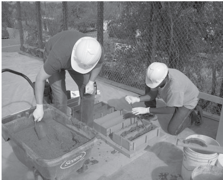
FIGURE A.37 Filling and rodding concrete in beams.
