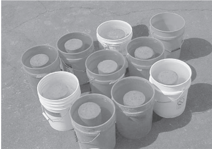
FIGURE A.39 Curing concrete cylinders in lime-saturated water.
