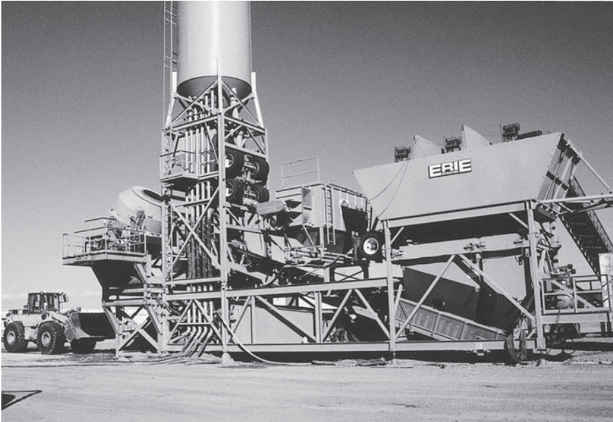
FIGURE 7.6 Mobile batcher mixer at the job site.
