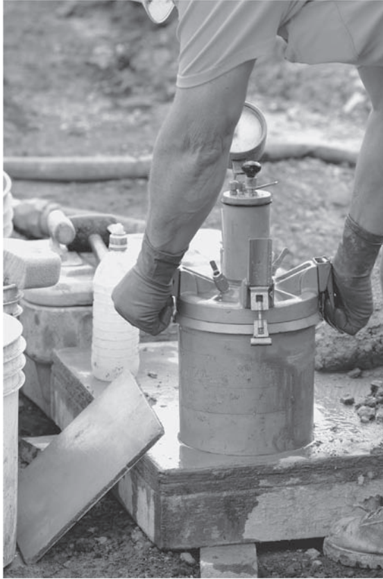
FIGURE A.34 Reading pressure meter. (Shutterstock/TFoxFoto)
