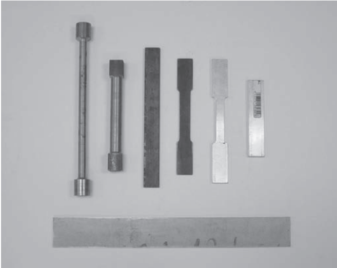
FIGURE A.6 Rounded and plate-type steel and aluminum tension test specimens.
