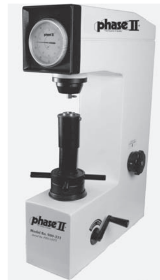
FIGURE 3.26 Rockwell hardness test machine. (Courtesy of Phase II)
