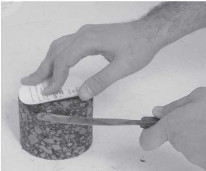
FIGURE A.63 Removing paper disk from a Marshall plug.
