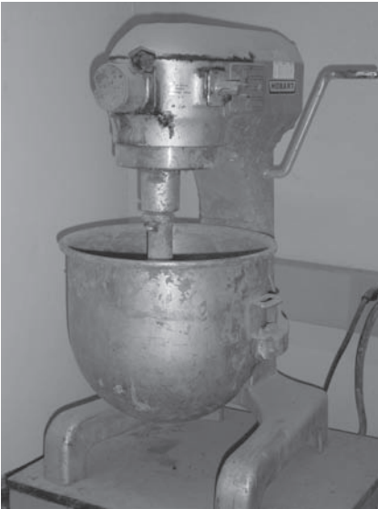
FIGURE A.60 Mixing HMA using a mechanical mixer.
