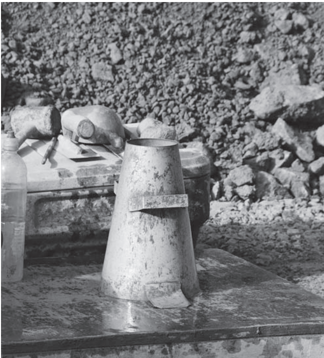
FIGURE 7.4 Slump test apparatus. (Fotolia/Bradlee Mauer)
