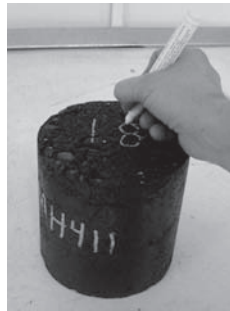
FIGURE A.59 Specimen prepared with gyrotory shear compactor.
