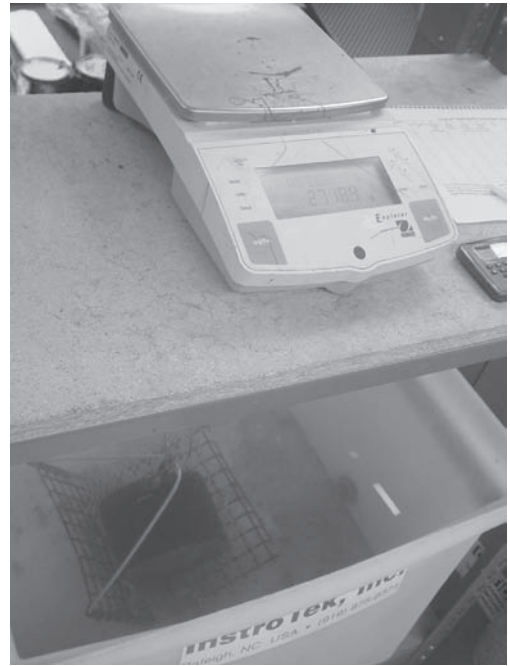
FIGURE A.65 Weighing HMA specimen in water.
