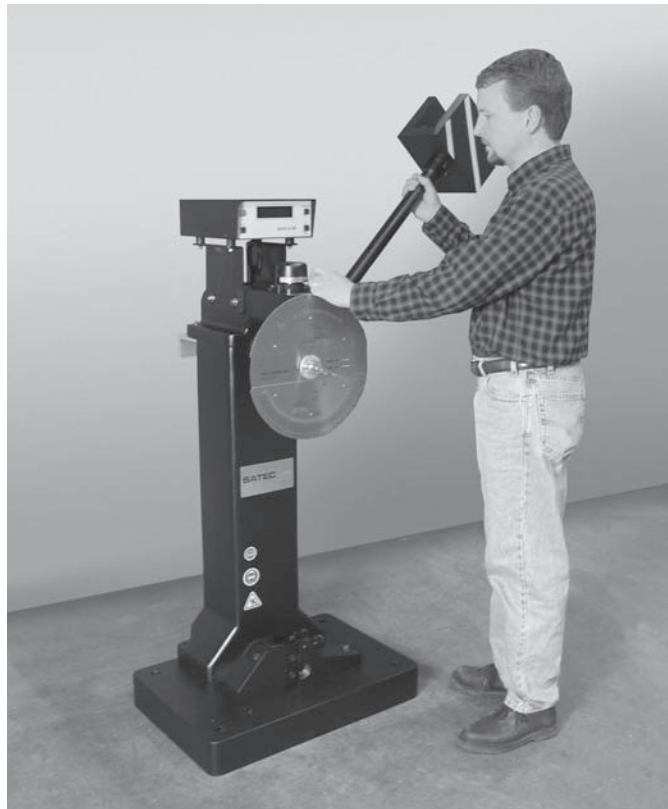
FIGURE A.12 Charpy V notch impact testing machine. (Courtesy of Instron®)
