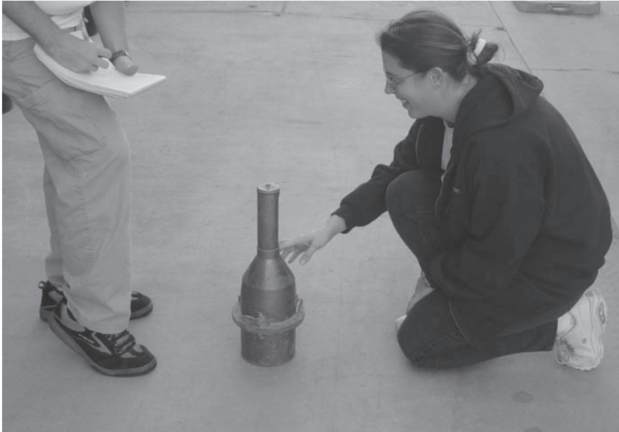
FIGURE A.35 Reading air meter.
