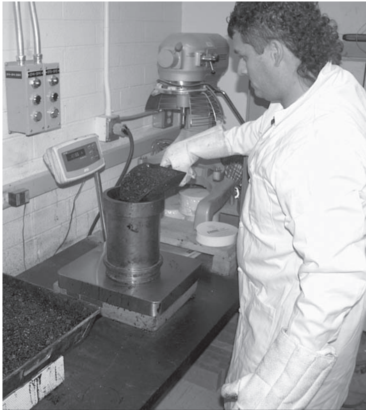
FIGURE A.57 Placing HMA in mold.
