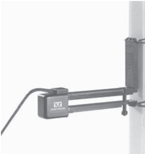
FIGURE A.74 Extensometer on an FRP composite specimen. (Courtesy of Instron®)
