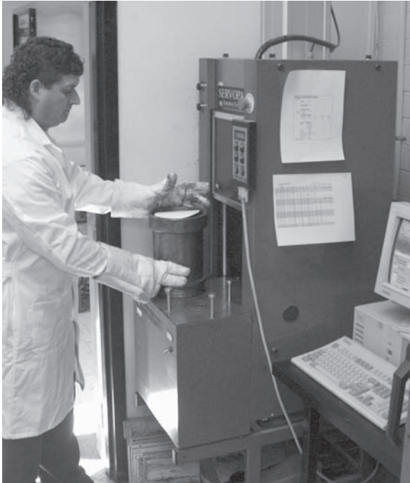
FIGURE A.58 Placing the mold in the gyrotory compactor.
