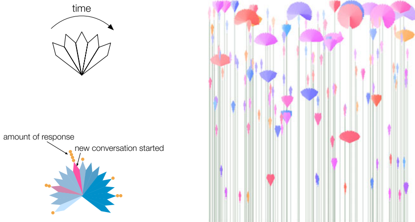
Fig. 7.56: This PeopleGarden shows about 1200 posts entered to a discussion board during a period of two months. Users are represented by flowers whose petals, in turn, represent individual messages posted by a user.
