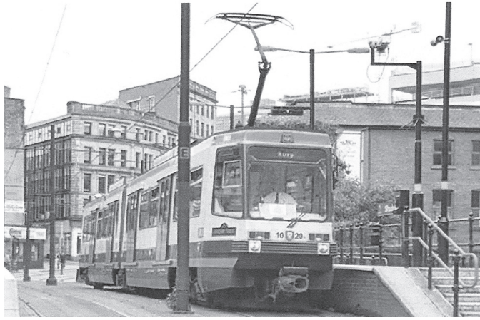
Figure 4.43 High-platform light rail system in Manchester city center (Photo: Greater Manchester Passenger Transport Executive)
