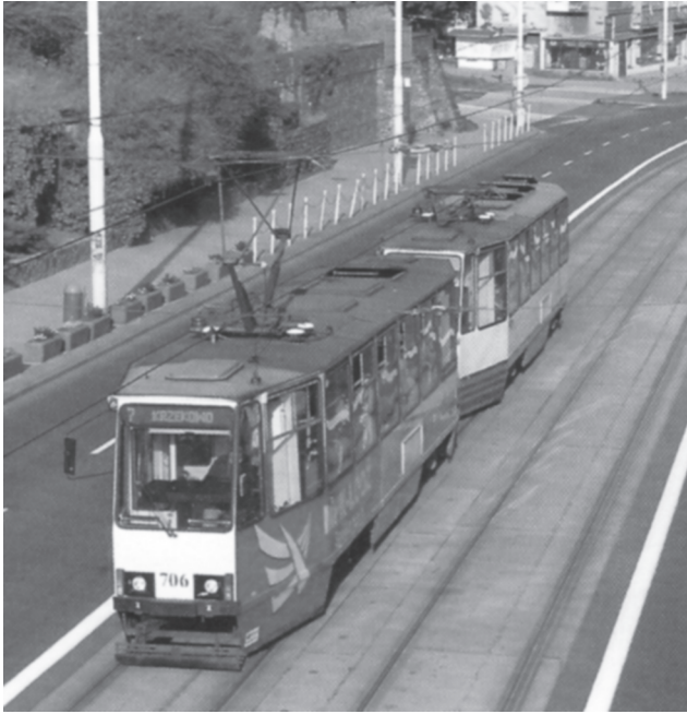
Figure 4.14 Road lane reservation in Szczecin, Poland (Photo: Neil Pulling)
