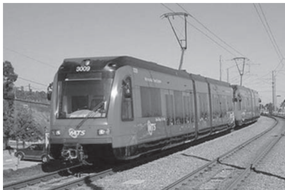
Figure 7.3 Orange line (Mission Valley East) low-floor cars (Photo: San Diego Transit)
