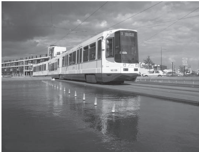
Figure 7.8 Nantes original two-car high-floor and added low-floor center (Photo: Nantes Tramway Authority)
