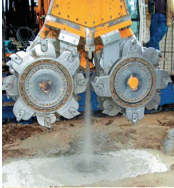
Fig. 6.20 Cutter head used for Cutter Soil Mix. (by Bauer)
