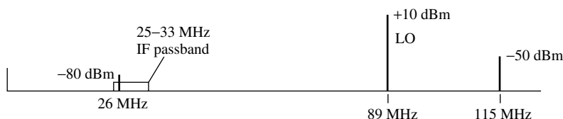
Fig. 8.18 Contaminant transferred from LO to IF.
