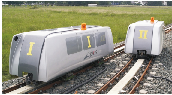
Fig. 2.2 RailCabs on the test track (Scale 1:2.5)
