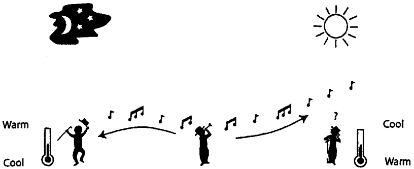
FIG. 3.22 The influence of temperature gradients on the propagation of sound.
