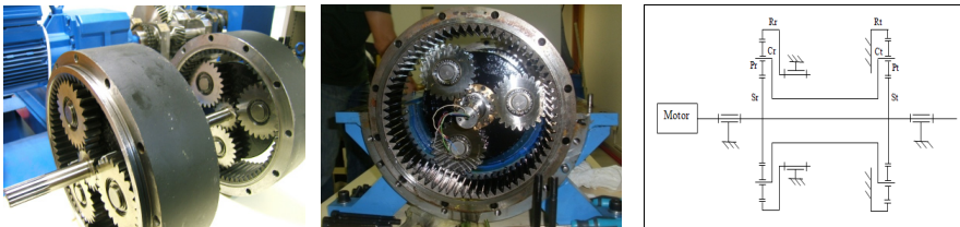
Fig. 1 Back to back planetary gear set rig
