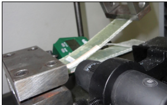
Fig. 2 MMF tests in the deformed configuration
