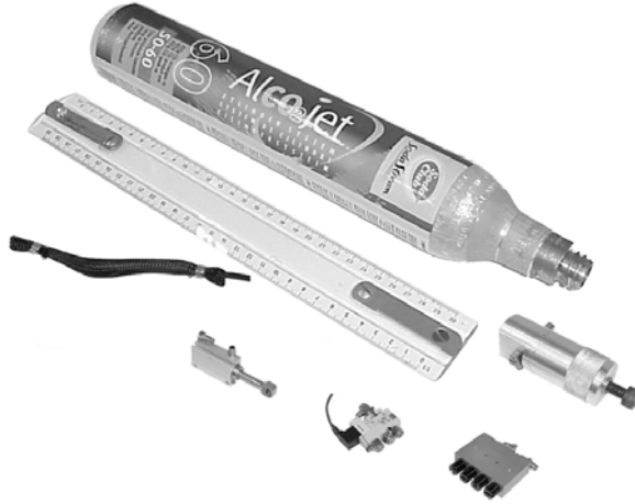
Fig. 5.8. The pneumatic components and a 30 cm ruler to indicate their sizes. The components are clockwise arranged according to the CO 2 flow through the system; 5.8 Mpa CO 2 canister, the first stage pressure regulator to 1.2 Mpa, a block of four second stage regulators to 0.6 Mpa, one of four low-power SMC TM valves, one of four small SMC TM cylinders and one of four Shadow TM McKibben muscles.
