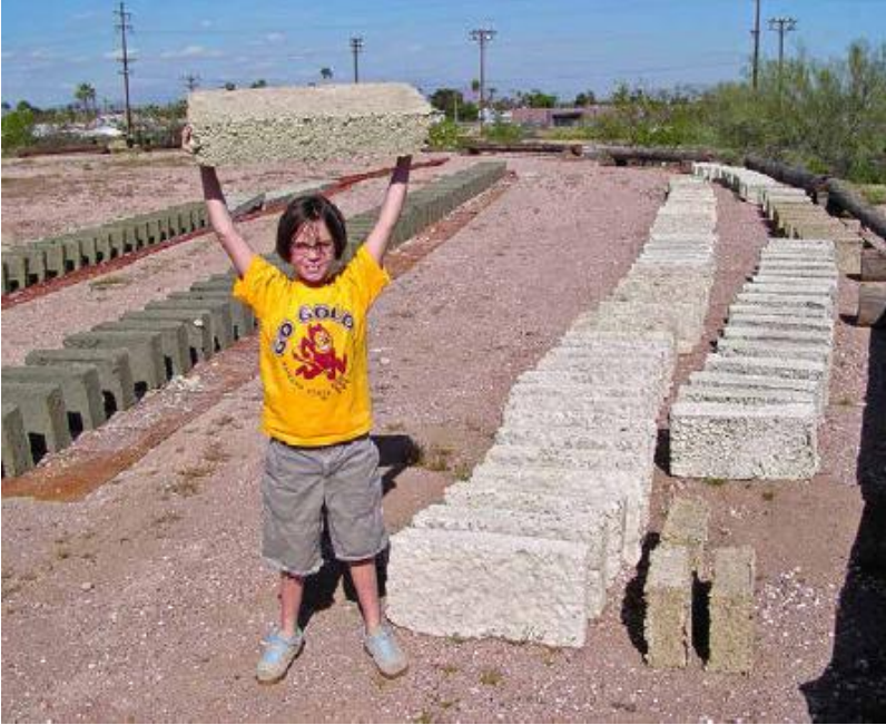
FIGURE 41.2. Nine-year-old Elizabeth Kemp demonstrates that papercrete is lightweight. This is an enormous advantage for owner-builders. [Credit: Barry J. Fuller]
