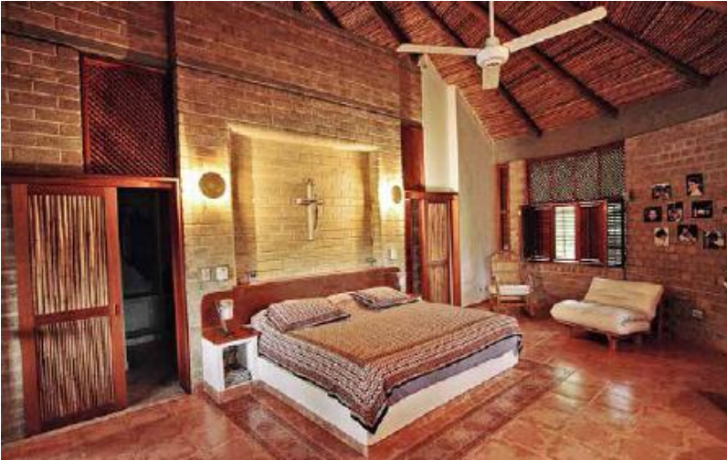
FIGURE 27.6. This dwelling by architect Dario Angulo in Colombia combines CEBs with wood, bamboo, tile and other natural materials to elegant effect. Note the judicious use of concrete to create a structural bond beam in this seismically active country. [Credit: Dario Angulo]
