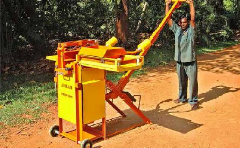
FIGURE 27.1. The hand-operated Auram Press 3000 developed by the Auroville Earth Institute in India. [Credit: Serge Maïni]
