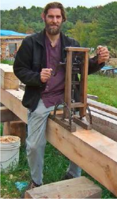
FIGURE 36.4. A boring machine allows a framer to drill a hole perpendicular to the face of the timber using hand power. Two or more of these holes are bored to the desired depth, then squared up with a chisel to make a mortise. [Credit: Devin Smith]
