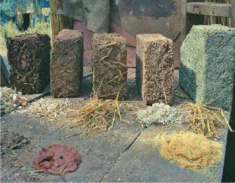
FIGURE 21.6. Athena and Bill Steen created these examples of how a variety of clays and fibers can be mixed together to make lightweight adobe blocks. Note the reed mat and burlap, which can be used as a support for plaster over wood or other materials. [Credit: Catherine Wanek]
