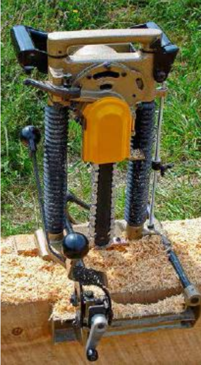
FIGURE 36.5. The chain mortiser may be the most significant advancement in timber-framing technique of the last four centuries. [Credit: Devin Smith]
