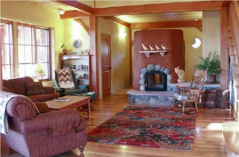
FIGURE 10.2. This EcoNest home in Grass Valley, California, is constructed using natural materials, including timber framing, straw-clay walls and clay plasters. The design features passive solar heating and natural daylighting, all part of the recipe for a healthy house. [Credit: T.J. Heater]
