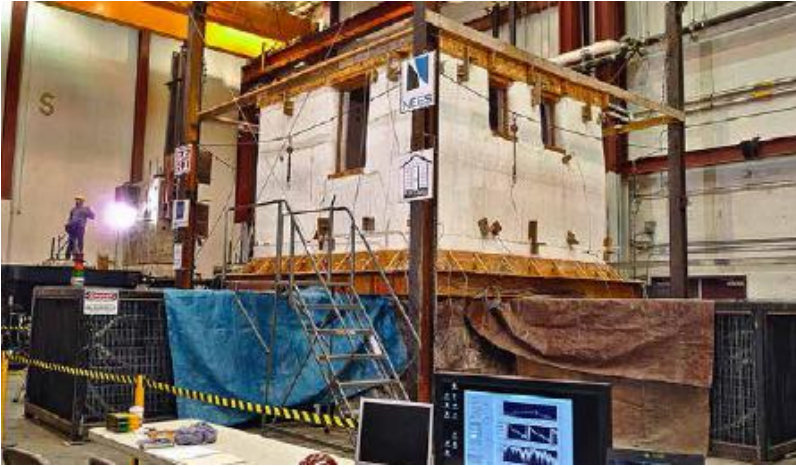
FIGURE 31.6. Tested on a University of Nevada “shake table,” a low-tech straw bale building system developed by Pakistan Straw-bale and Appropriate Building (PAKSBAB) withstood twice the seismic acceleration of the Northridge, California, earthquake. [Credit: Darcey Donovan]
