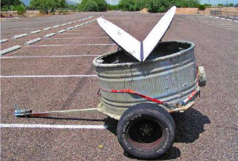
FIGURE 41.3. This tow mixer built by Barry J. Fuller easily tears apart newspapers and magazines — even small catalogs and books. The original wooden cover allowed too much papercrete to escape and was replaced by a plastic tarp, secured with a tie-down strap. [Credit: Barry J. Fuller]
