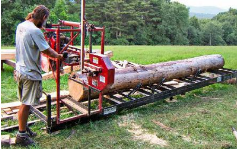
FIGURE 36.1. Timbers can be milled onsite using a portable mill like this Wood-Mizer. This allows the utilization of onsite resources, reduces transportation cost and energy and allows waste products to be returned to the forest whence they came. [Credit: Devin Smith]
