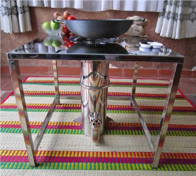
FIGURE 18.4. This stainless steel gasifier, designed by Paul Olivier, is being manufactured for distribution in Vietnam. It converts rice hulls and other agricultural wastes into cooking gas and biochar, a prized soil amendment. [Credit: Paul Olivier]
