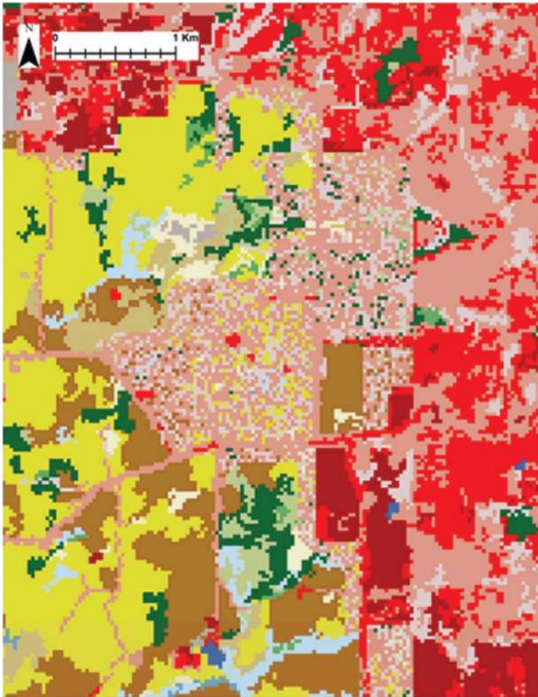
FIGURE 8.7 Example of grid cell raster mosaic phenomena depicting potential future land cover change. Exact arrangement of grid cells is determined randomly where there are more candidate pixels for transformation than are required.
