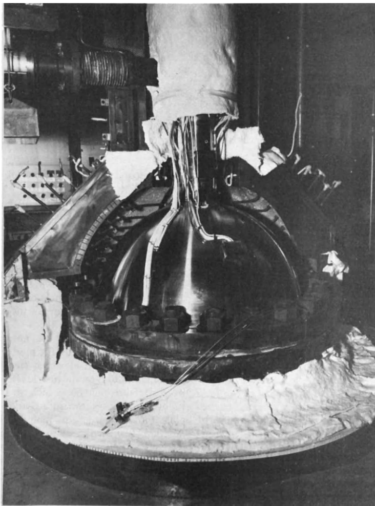
Fig. 13. Instrumented nozzle-to-sphere specimen of type 304 stainless steel.
