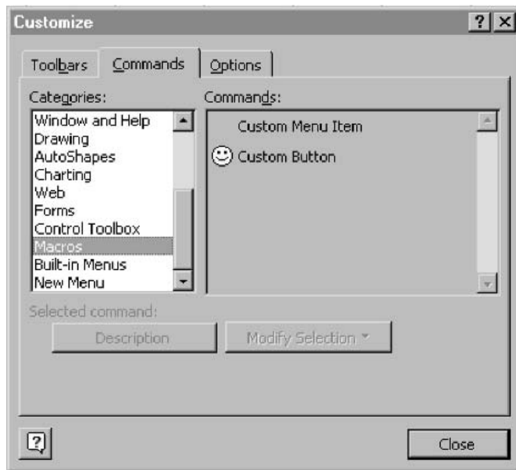
Figure A.19 Associating a macro with a menu item or a button
