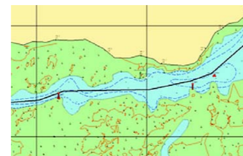
Figure 4.6.7 Mapping of dangerous areas for navigation showing channel and aids to navigation (1:2000).
