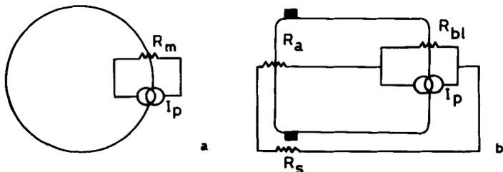
FIG. 1. Equivalent electrical circuits used to calculate the effect of the pump current  $I_p$  on the membrane potential, in a nonpolarized cell (a) and in an epithelial cell (b).
