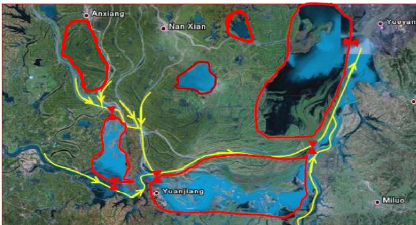
Figure 4. Application of SPP to the eastern, southern and western lakes where the red lines are the levees, yellow lines are the streams and the triangles are the sluice gates.
