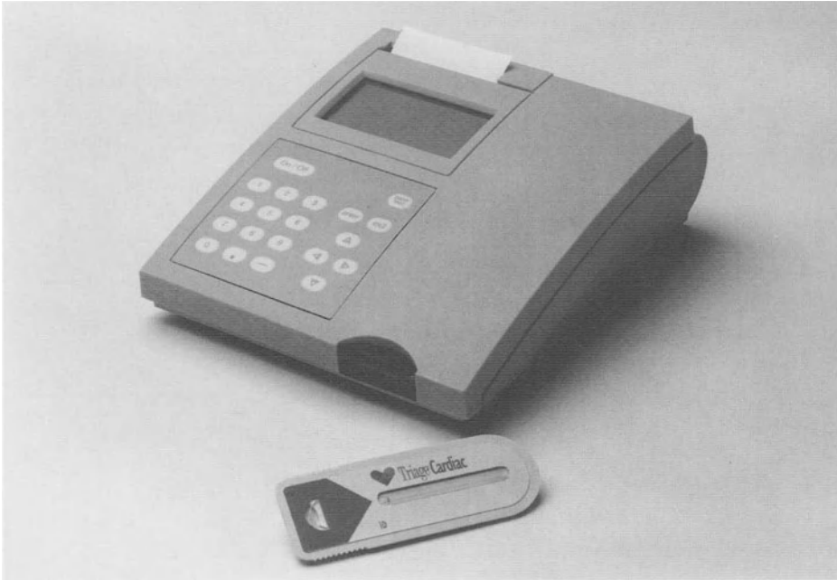
Fig. 7. The Triage ® Meter and Triage ® Cardiac Panel, showing the instrument and immunoassay cartridge (courtesy Biosite Diagnostics).
