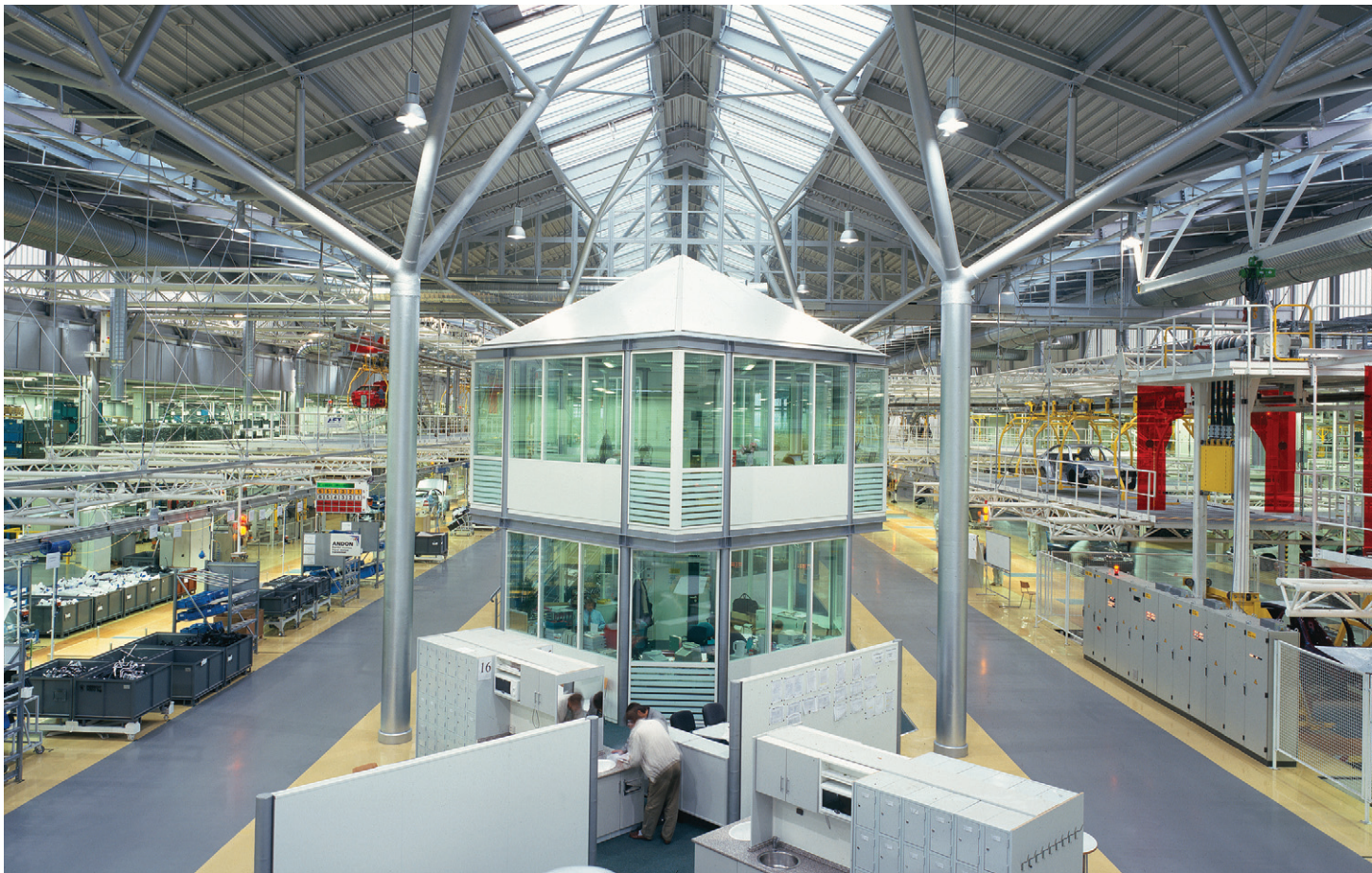
Figure 4-3 The form of the Skoda plant's interior follows the flow of the assembly process and promotes awareness of what is happening in the process.
