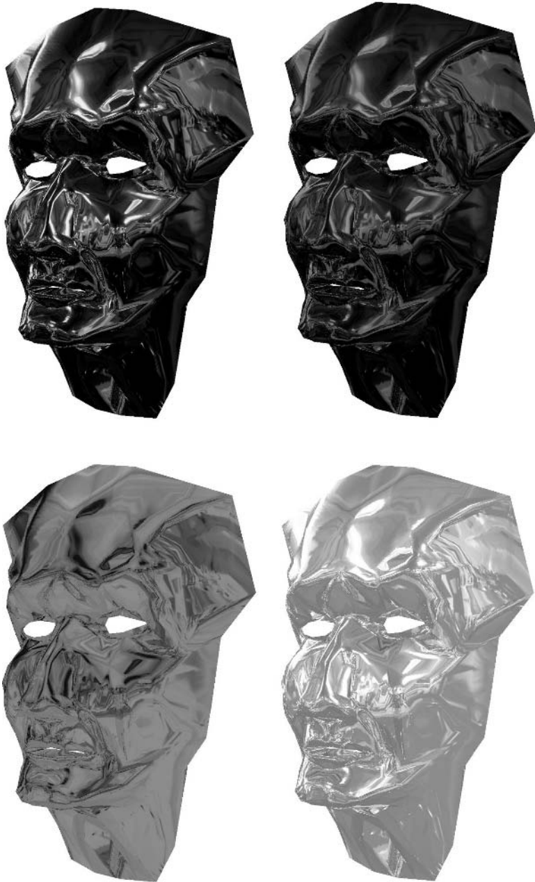
Figure 5.5 Screen shots from the environment map sample application. Top left: Replacement mode. Top right: Modulation mode. Bottom left: Blend mode. Bottom right: Add mode. (See also Color Plate 5.5.)
