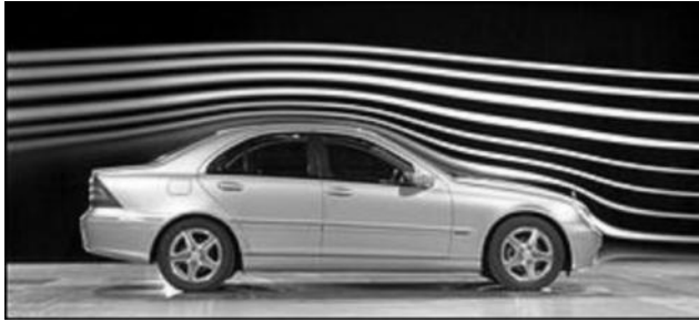
FIGURE 18.1 Smoke-traced streaklines of flow around a car. (From DaimlerChrysler. With permission.)
