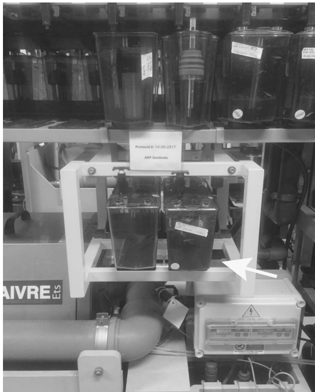
FIGURE 24.5 Sentinel tanks. Specialized housing tanks called sentinel tanks are designed to expose animals to effluent water to detect pathogens in the system. In this example (white arrow), the tanks are mounted on a special, designated rack on a RAS.
