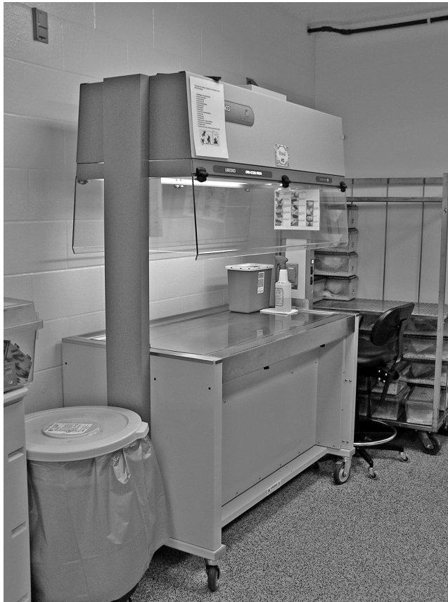
FIGURE 21.7 Example of a laminar flow workstation. In this configuration, air is HEPA filtered in the top of the unit and forced down over the work surface. Exhaust ports on the edges of the work surface collect the air for additional filtration before the air is exhausted into the room. (Photo by Deb Hickman.)
