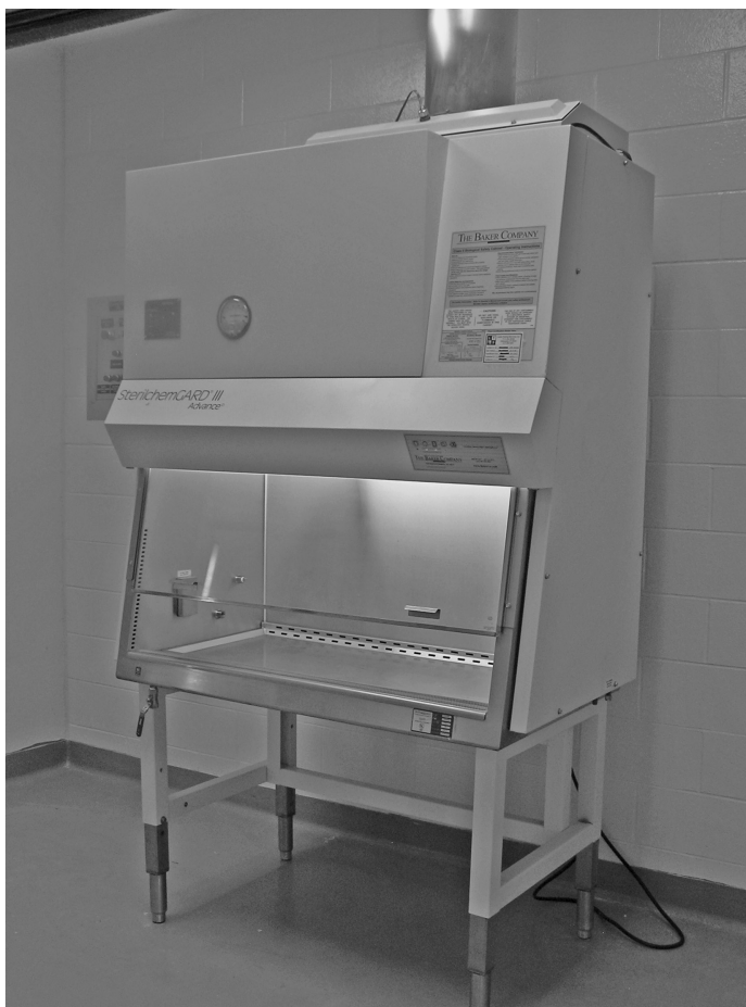
FIGURE 21.8 Example of a BSC suitable for use with biological hazards. (Photo by Deb Hickman.)
