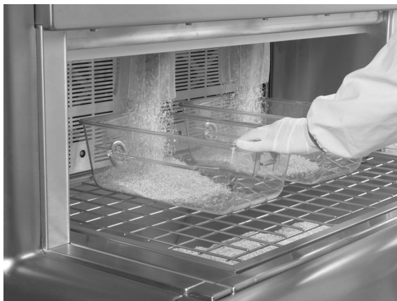
FIGURE 27.3 Automatic bedding dispenser. (Courtesy of Tecniplast.)
