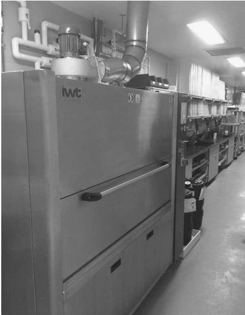
FIGURE 24.4 Tank sanitization. New tank washers are being developed specifically to safely sanitize aquatic housing tanks.
