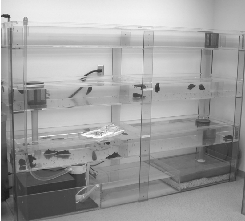
FIGURE 25.1 Housing system for Aplysia , a species commonly used in neuroscience research. (Photo by D.P. Baumann.)
