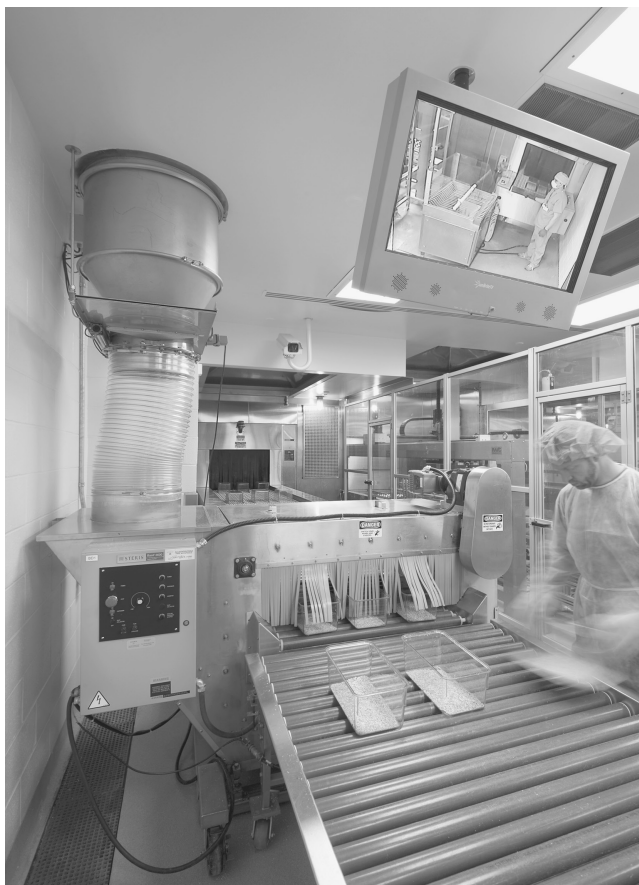
FIGURE 27.4 In-line bedding dispenser with integrated pneumatic delivery system. (Courtesy of MSKCC.)
