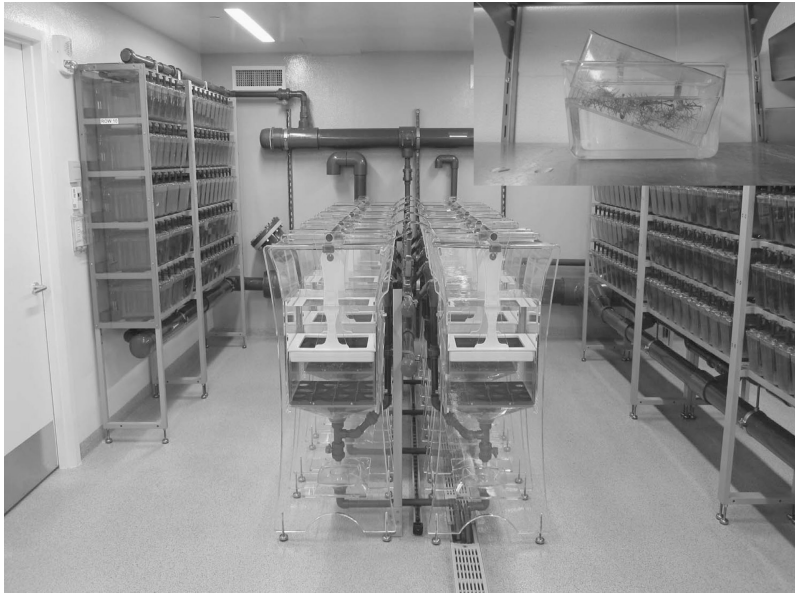
FIGURE 24.6 Breeding systems. Specialized group breeding tanks (for zebrafish) are used to generate large quantities of embryos for experiments. Inset: Small breeding tank/insert used for individual pairs or small groups (<10) of fish.
