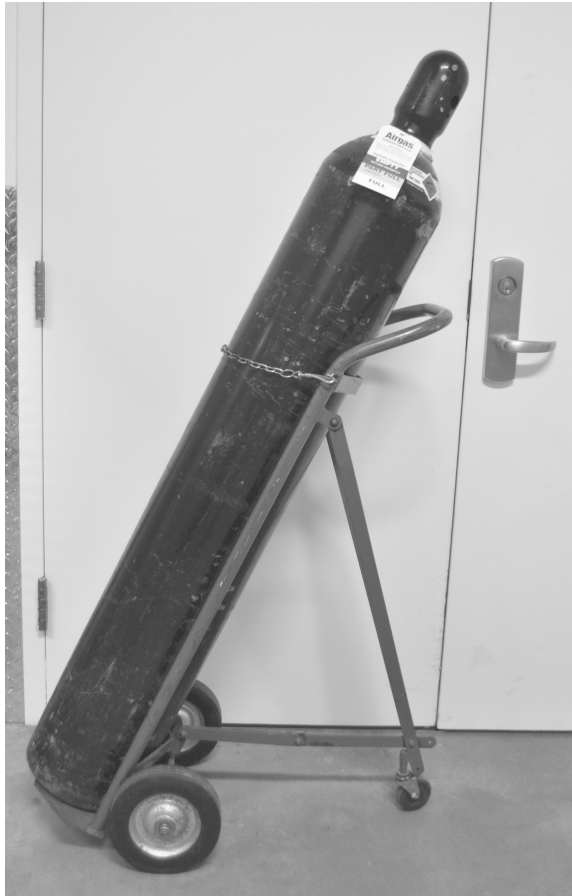
FIGURE 26.14 Example gas tank–securing device. This type of cart allows the tank to be easily moved as well. (Photo by Michelle Wallace-Fields.)
