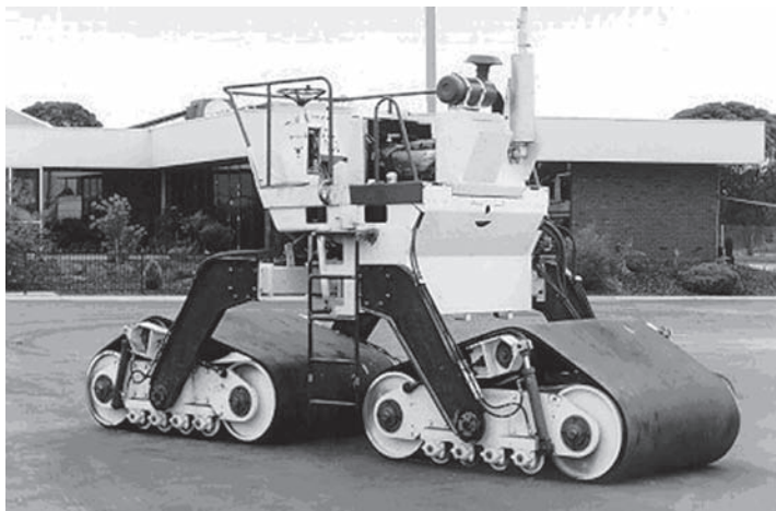
Figure 3. New generation successor to AMIR, the HIPAC compactor.
