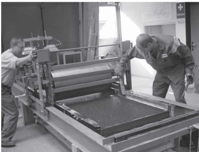
Figure 1. Laboratory steel roller compactor.
