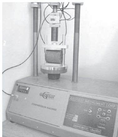
Figure 3. Machine used for ITS and UCS test.
