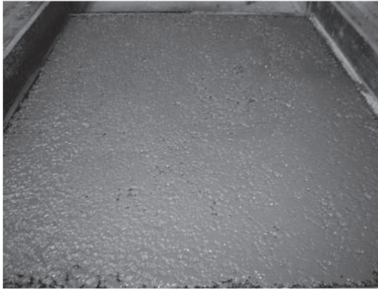
Figure 7. Surface of the base layer after the application of wet dirt (wet fine corundum).
