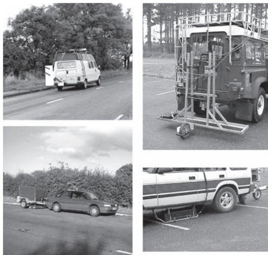
Figure 10. UK ground penetrating radar equipment taking part in comparative trials.
