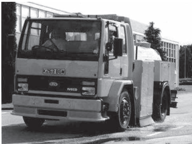
Figure 5. Sideway-force coefficient routine investigation machine (SCRIM).
