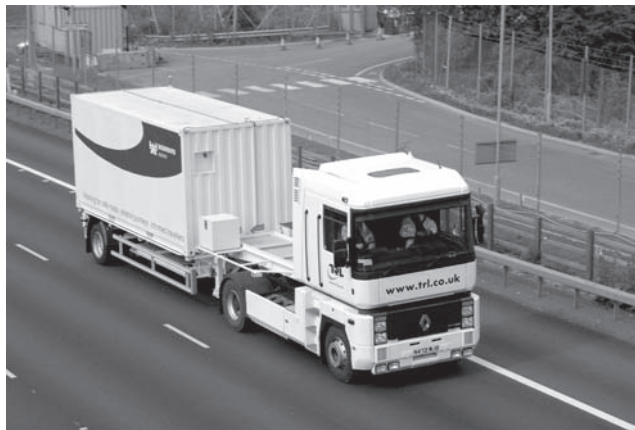
Figure 9. UK highways agency TSD surveying deflection response of motorway at 80 km/h.
