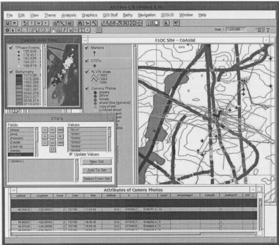
Figure 12.2 Example of a typical graphic interface for Vents Program scientists working in the field. Display includes a detailed map of the study area with previous submersible tracklines, CTD stations, interpreted camera images, bathymetry and lava flow boundaries. Insets include a time-dependent epicentre map with bathymetry of the broader study area, metadata for CTD casts, and an attribute table of interpreted camera images with fresh lava flows highlighted. This data base was continuously updated as new observations were collected.
