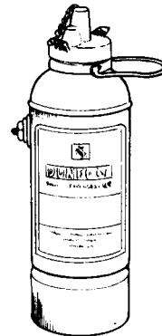
Figure 2.13 Dry powder extinguisher
