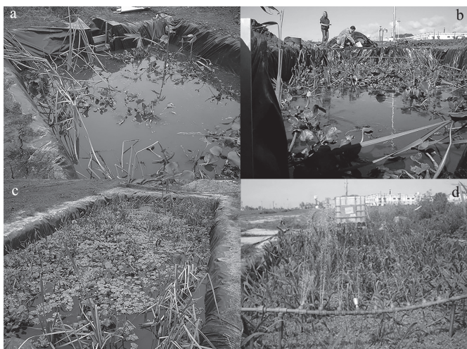
Figure 1. Pilot scale wetland: (a) initially; (b) after 1 month; (c) after 3 months; (d) after 9 months from the beginning of operation.
