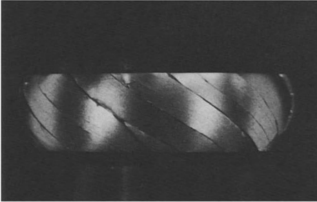
Fig. 6. Cracked outer surface of upset steel cylinder after approximately 70 percent reduction-in-height.
