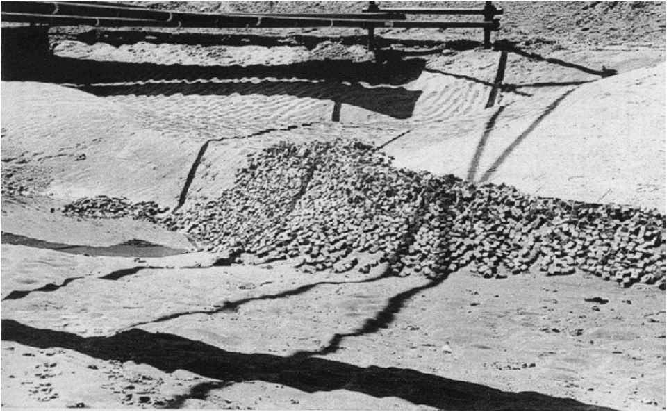
Figure 11-39 Model test with falling apron (CNR,1994)
