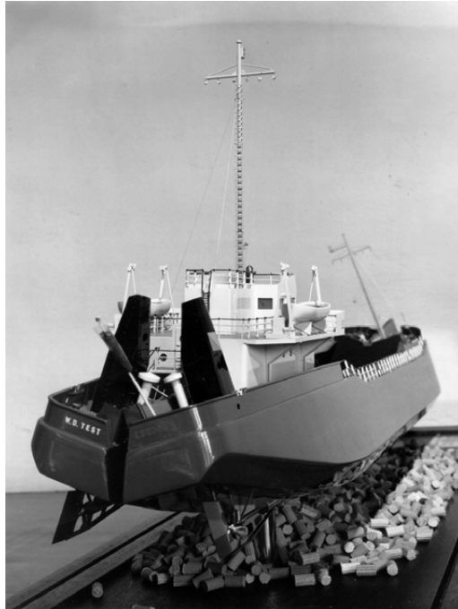
Figure 13-3 Split barge (Boskalis)
