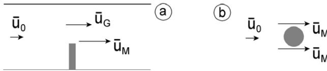
Figure 3-16 Definition of velocities in relation to K_v
