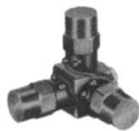
Figure 8.31 Example of a three axis piezoelectric accelerometer [Ziegler]
