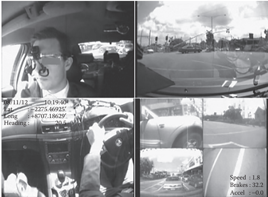
FIGURE 2.2 Example still frame from multi-camera footage in an instrumented vehicle.
