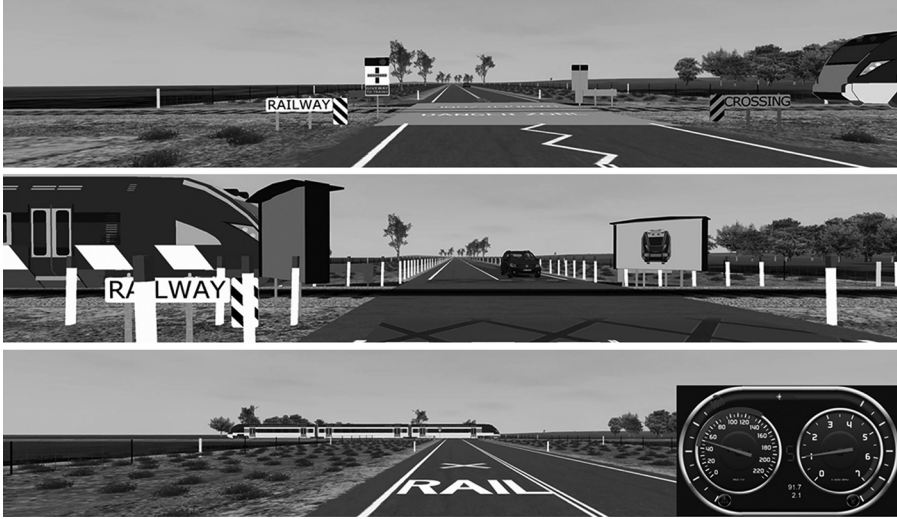
FIGURE 9.3 Screen shots depicting the three novel rural rail level crossing designs evaluated in Simulator Study 2 and Study 3: the Simple But Strong crossing (top panel); the Ecological Interface Design crossing (middle panel); the GPS Average Speed interface (bottom panel).
