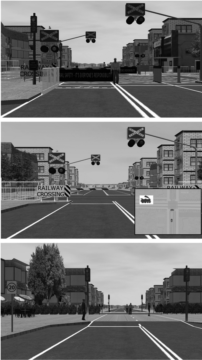
FIGURE 9.1 Screen shots depicting the novel urban rail level crossing designs: the Comprehensive Risk Control crossing (top panel); the Intelligent Level Crossing (middle panel); the Community Courtyard crossing (bottom panel).
