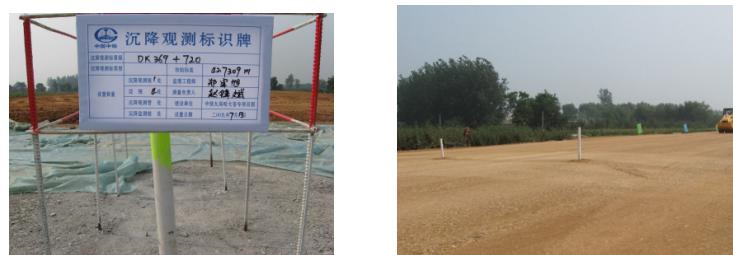
**Figure 10. the measurement of the settlements**
