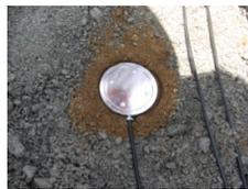
Figure 14. the measurement of compressive stress (Soil pressure box)
