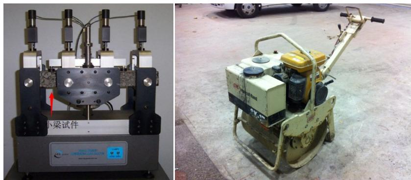
**Figure 1. Four-Point Bending Fixture (Left) and Roller for the Test (Right)**
