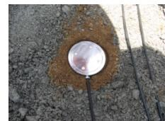
**Figure 14. the measurement of compressive stress (Soil pressure box)**
