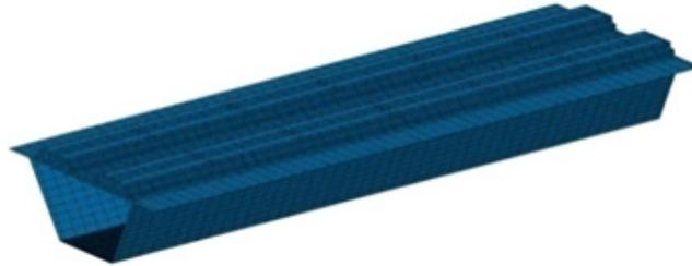
**Figure 1. Finite element model of CRTS-I slab ballastless track-bridge coupling dynamics**
