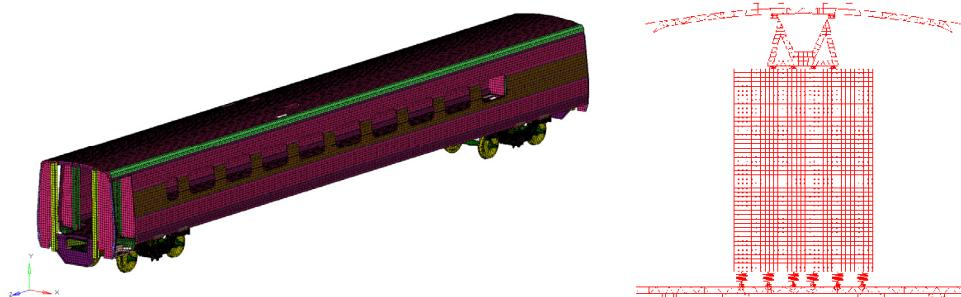
**Figure 4. The finite element model**
