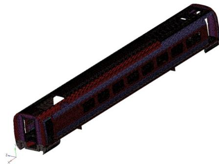
**Figure 1. Car bodywok finite element model**
