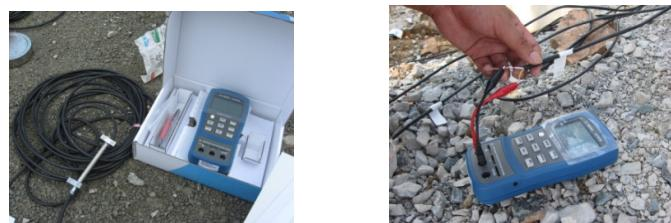
**Figure 18. measuring instrument of geogrid tension**
