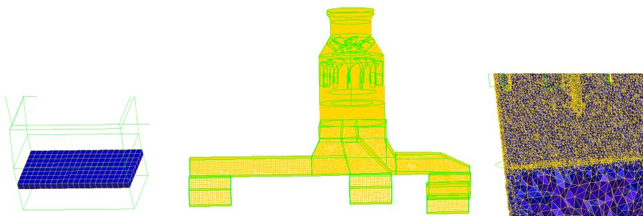
**Figure 2. Finite elements of the whole model and Local amplification view**
