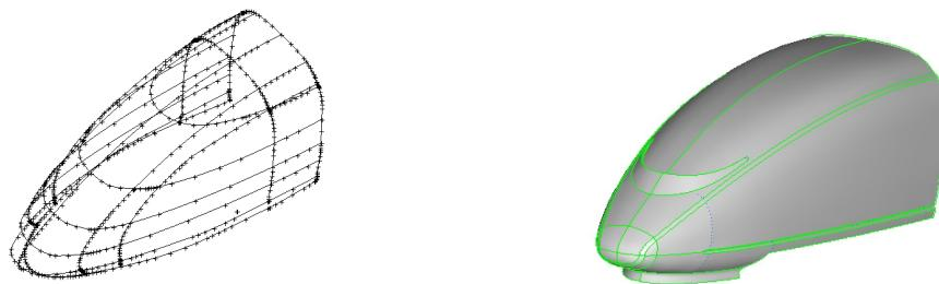
**Figure 4. Staggered grid line and geometric model of train head**
