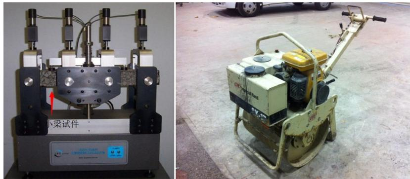
**Figure 1. Four-Point Bending Fixture (Left) and Roller for the Test (Right)**
