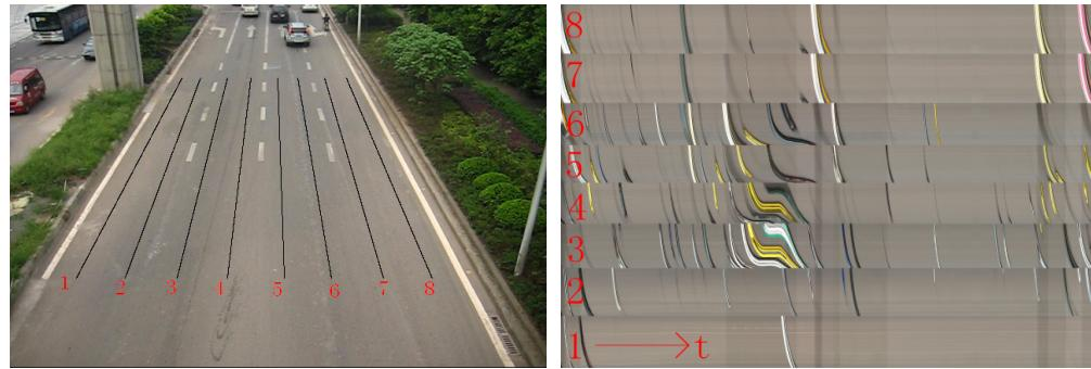
(a) The position of line-t section      (b) The epipolar plane image
