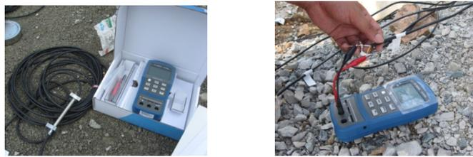
Figure 18. measuring instrument of geogrid tension
