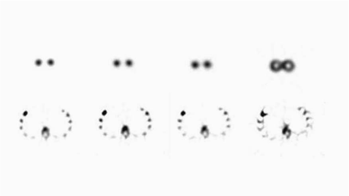
FIGURE 17.11. Artifact from inadequate center of rotation (COR) calibration: the effect an inappropriately specified COR has on SPECT image quality. The top row is a series of point sources and the bottom row is a ^{99m}\text{Tc} -MDP bone scan. The first image in each row, far left, represents the data recon-
