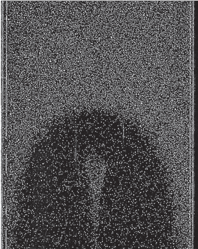
FIGURE 3.1.4 PIV image of upward propagating lean limit methane flame.
