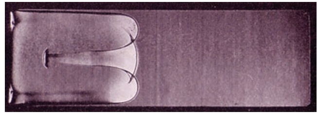
FIGURE 5.3.5 The flame shape created when a weak shock (pressure ratio 1.10) interacts with it from the right. The image shows a flame funnel, 2.5ms after the interaction begins; the flame is a stoichiometric butane/air mixture. (Adapted from Markstein, G.H., Nonsteady Flame Propagation , AGARDograph, Pergamon Press, New York, 1964.)
