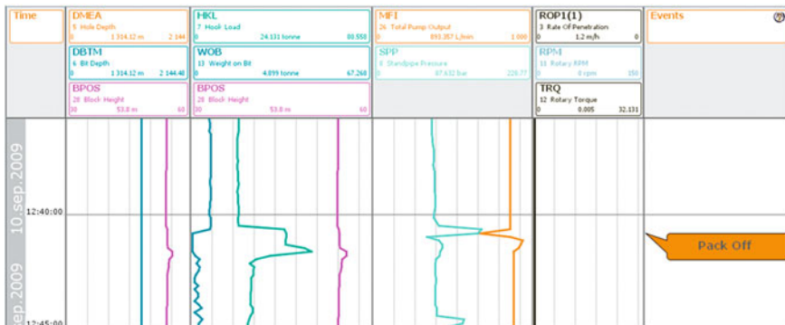
Fig. 11 A pack off event is recognized and shown in the time view when the pressure (SPP) increases while the mud flow (MFI) is stable
