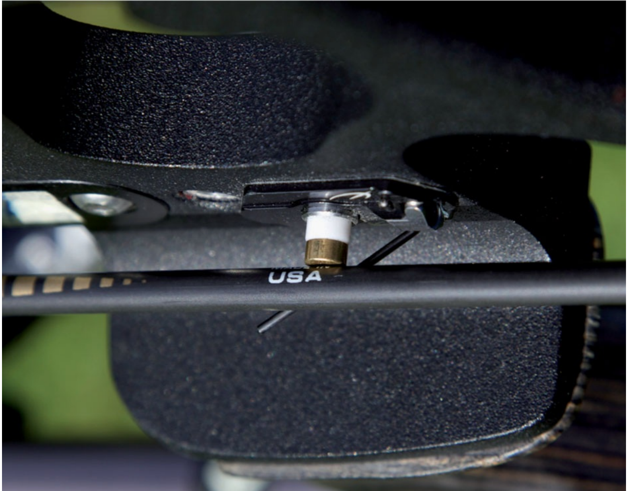
Arrow rest arm set wrongly from above.
