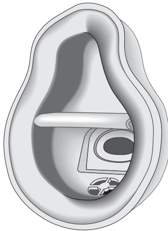
Figure 7 Prototype facemask occluding the nose. This ensures mouth breathing, thereby avoiding nasal drug deposition.
