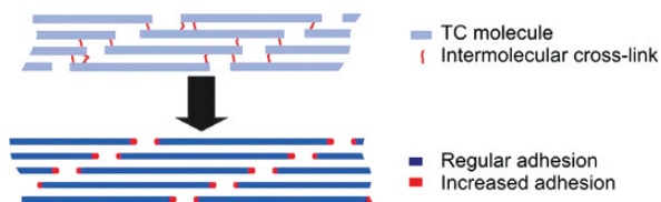
Fig. 8.28 Schematic showing how the presence of cross-links is modeled by increased adhesion at the ends of each molecule, in segments of 60 \text{ \AA} to the left and right of each tropocollagen molecule. Implementing a variation of the amplification of the adhesion strength constitutes a simplistic model for varying cross-link densities. A parameter \beta is introduced that describes the increase of adhesion at the ends of each TC molecule, so that \tau = \beta\tau XL ( \tau is the adhesion force/length between two TC molecules). The parameter \beta = 15 corresponds to the case when approximately one cross-link is present at each end of a tropocollagen molecule
