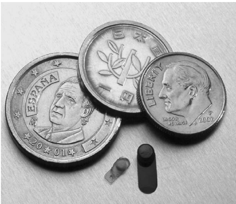
Figure 5 Photograph of a drug delivery device containing 2 mg of fluocinolone acetone (left). Ganciclovir device is shown on the right for comparison. Note the smaller size of the fluocinolone device. The drug core is surrounded by a polyvinyl alcohol/silicone laminate.
