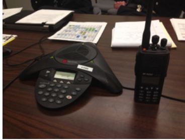
Figure 3-2. A speakerphone is commonly used for conference call incident bridges; use it like the public safety radio on the right
