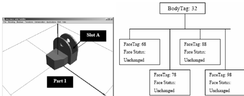
Figure 4.12. Designed part and corresponding information model
