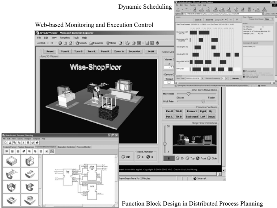
Figure 8.19. An integrated system for collaborative manufacturing
