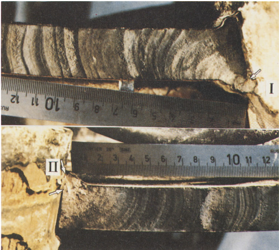
Fig. 5 Initiation point for the fatigue cracks in the brace D6.
