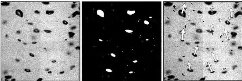
Fig. 2. Gray scale image of bubbly flow with added tracer particles (left), detected objects in the binary image (middle) and instantaneous velocity vectors (right).
